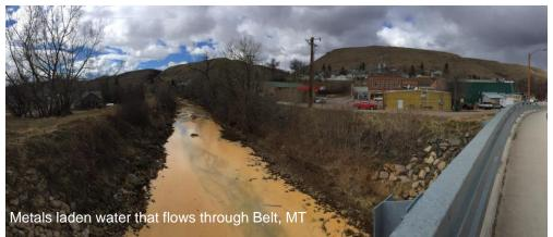
The AML Program is planning to build a water treatment plant in Belt to treat acid mine drainage from the abandoned coal mines surrounding the town. The pH-2 water contains elevated levels of metals including iron and aluminum. This water contaminates Belt Creek which runs through the middle of the community. The treatment plant is designed to meet all water quality standards and will restore Belt Creek to its beneficial uses.
