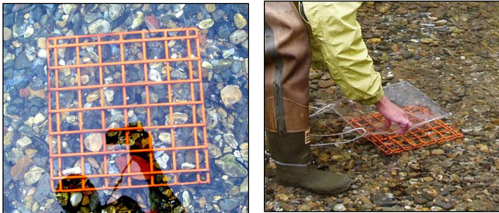
Figure I-2. Grid design used for grid tosses to determine percent fines in pool tails.
