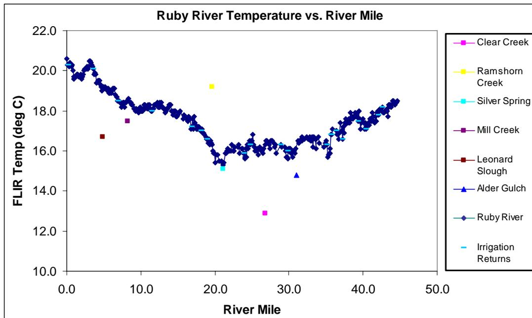
**Figure 7. Channel temperatures plotted by river mile for Lower Ruby River**
