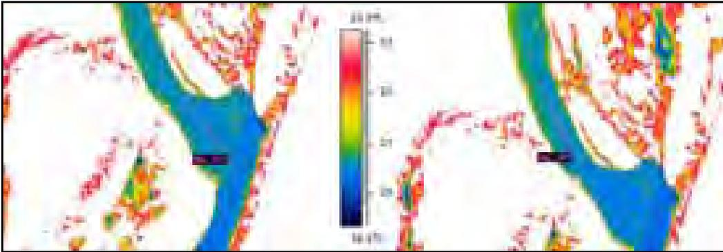
**Figure 5. Temperature sampling method. The image on the right was captured two seconds after the image on the left as the helicopter was moving upstream. Temperature data for each image is averaged along the magenta line in the center of each image.**
