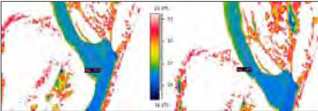
**Figure 2: Temperature sampling method.** The image on the right was captured two seconds after the image on the left as the helicopter was moving upstream. Temperature data for each image is averaged along the magenta line in the center of each image.
