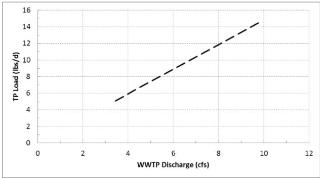
Figure 5-11. WLA for total phosphorus from the Kalispell Wastewater Treatment Plant.
