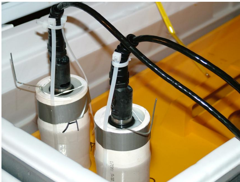
Figure 3.2. Measurement of sediment oxygen demand in sediment core samples, Yellowstone River, August 2006. A. Paired sediment cores in their water bath, with YSI model 85 DO meters attached. The tube on the right only contained river water and was used to measure BOD. B. Close-up of the sealed sediment cores and attached YSI DO probes. The metal wires were attached to paddles used to stir the water above the sediments just prior to taking the DO measurements. Water bath temperature was maintained at the temperature measured in the river during sediment collection.
