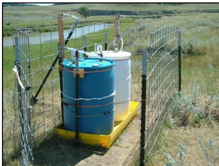
**Figure 3-3. The Nutrient Supply Tanks for the High Dose Reach.**
