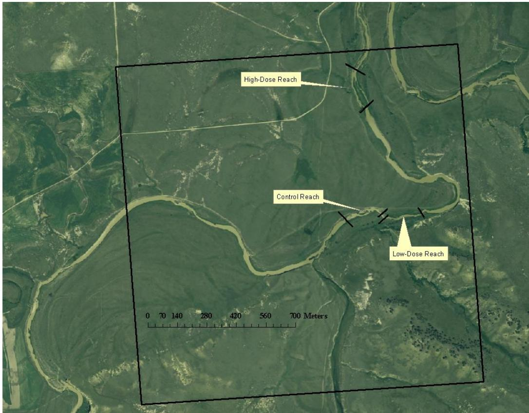
Figure 3.2. Box Elder Creek study site. Stream flows from left to right. The black outlined box is the boundary of the state-owned parcel. Start- and end-points of the Control, Low-Dose, and High-Dose reaches are shown by black lines perpendicular to stream flow.
