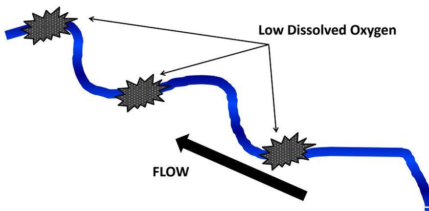
**Figure 5-1. Longitudinal Zones of Low Dissolved Oxygen, as Suggested by Findings in the High Dose Reach.**
