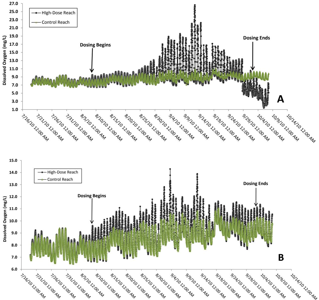
**Figure 4-5. Dissolved Oxygen Patterns Recorded by Sondes Located in the Control- and High Dose Reaches in 2010.**
