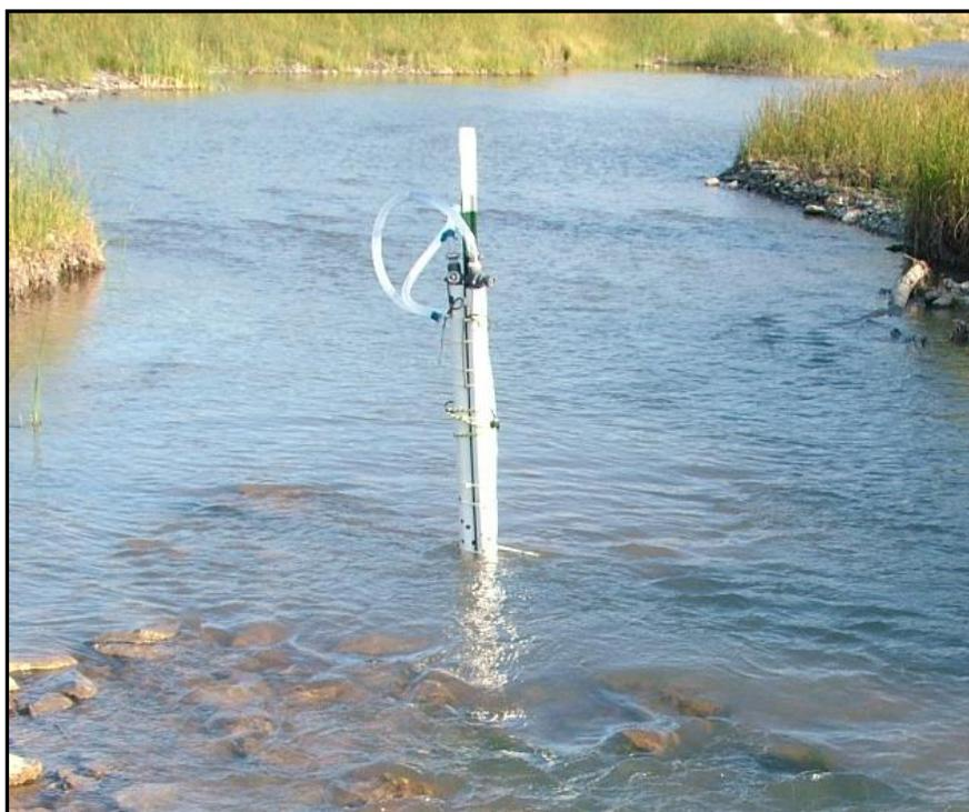
**Figure 3-4. The Nutrient-dripper Assembly, Located Mid-channel at the Head of a Riffle.**
