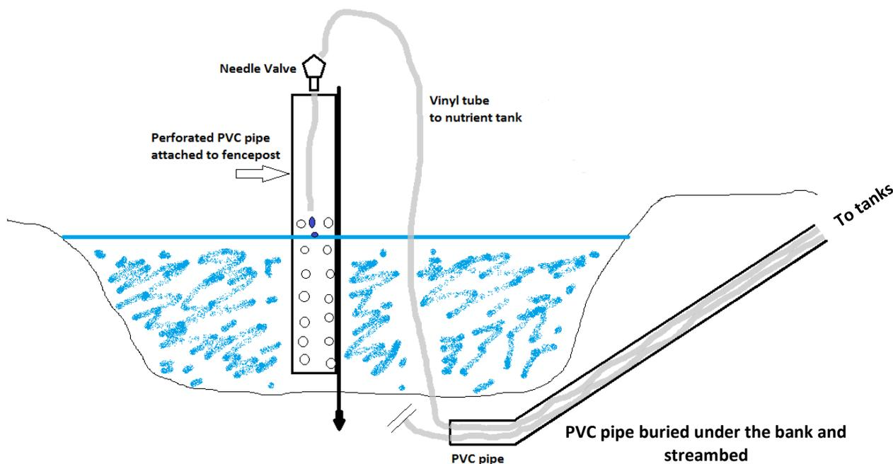
**Figure 3-5. Cross-section Diagram of the Instream Nutrient-dripper Assembly.**
