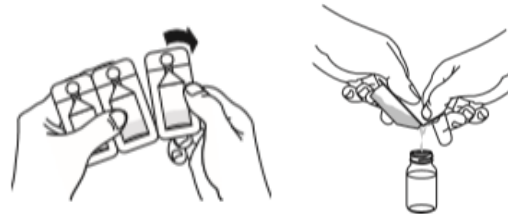
Figure 3 – Adding Colilert reagent packets to E. coli samples (IDEXX Laboratories, Inc., 2019)
