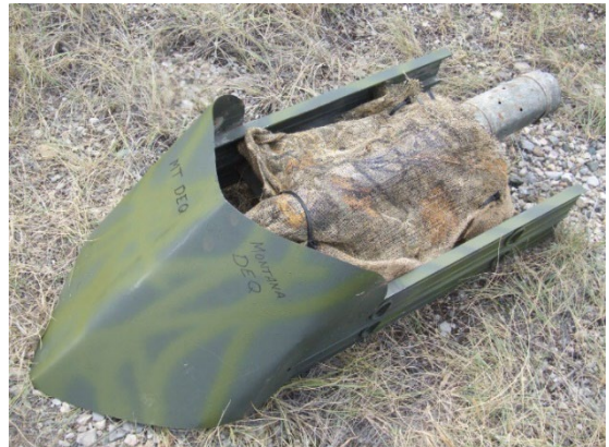
Figure D-7. Sonde with camouflage. Camo burlap in place over the sonde, and sheet metal shroud in place over the sensor end of the sonde.
