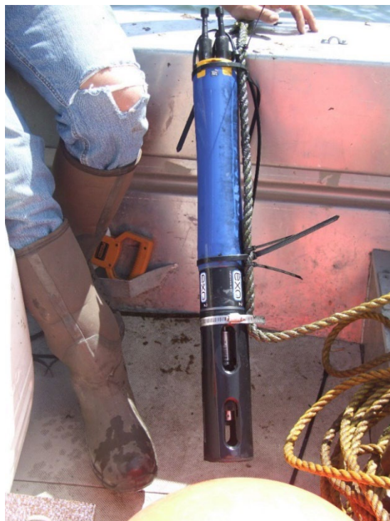
Figure D-2. Sonde attached to buoy line close-up. YSI EXO™2 sonde attached to polypropylene buoy line with multiple (4) zip ties and hose clamps. Smaller zip ties around poly rope prevents movement of attachment points on the line.
