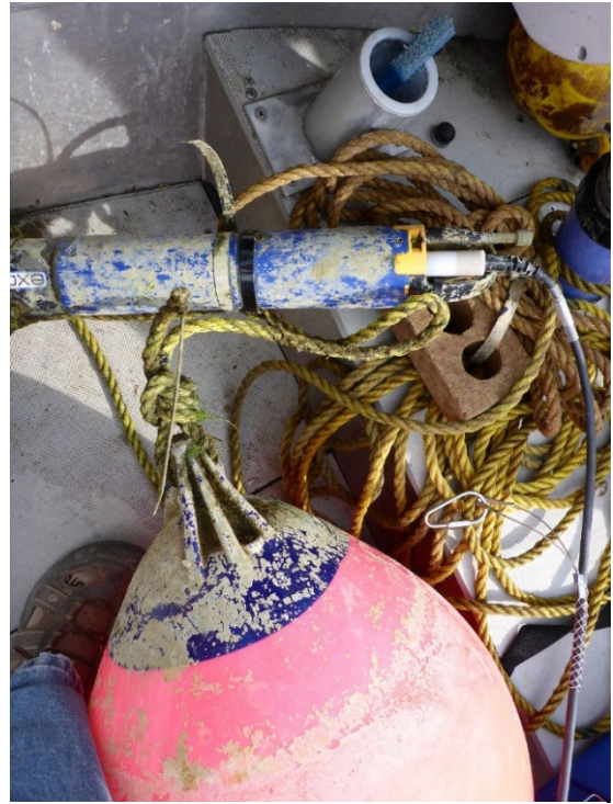
Figure D-5. Post-deployment condition – calcium carbonate. Buoy with calcium carbonate crusts, upper sonde and brick intermediate line weight.
