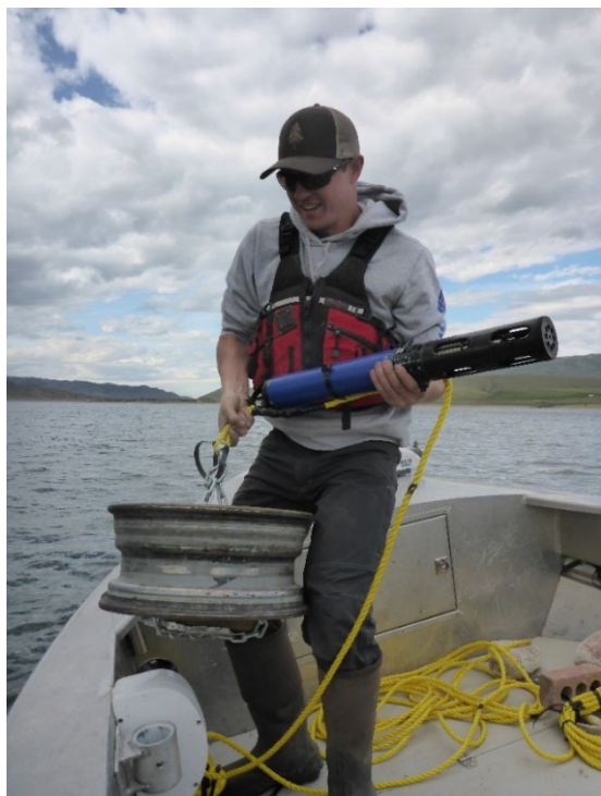
Figure D-1. Sonde attached to buoy line. Lower YSI sonde attached to buoy line in a sensors-upward orientation.
