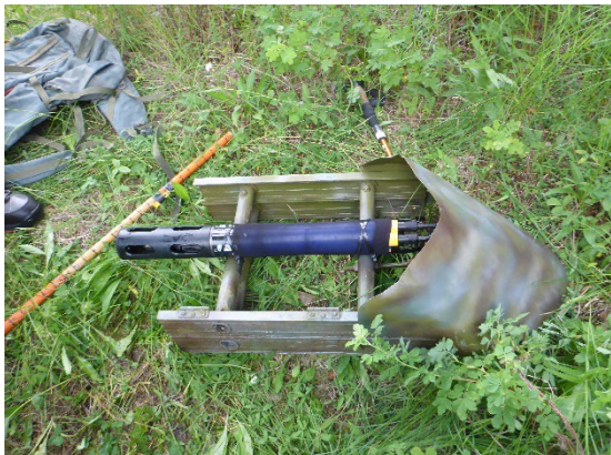
Figure D-8. Sonde and sturgeon. YSI EXO™2 sonde and sturgeon fixture.
