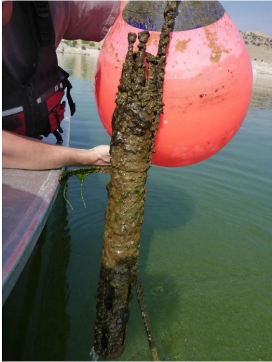
Figure D-6. Post-deployment condition – calcium carbonate and algal growth. Sondes in the euphotic zone of reservoirs tend to accumulate a lot of algal growth and calcium carbonate.
