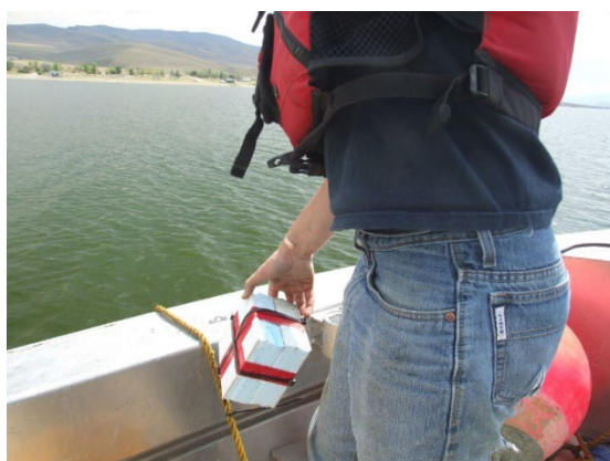
Figure D-4. Intermediate buoy. Small Dow foam board buoy added to buoy line to help the lower sonde stay off the lake bed.
