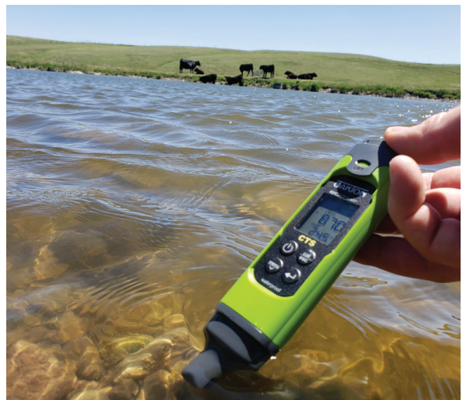
Using a specific conductance meter to estimate salt concentration in a stock pond. Photo by Adam Sigler.
