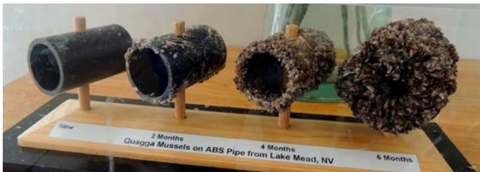
QUAGGA MUSSELS ON ABS PIPE FROM LAKE MEAD
