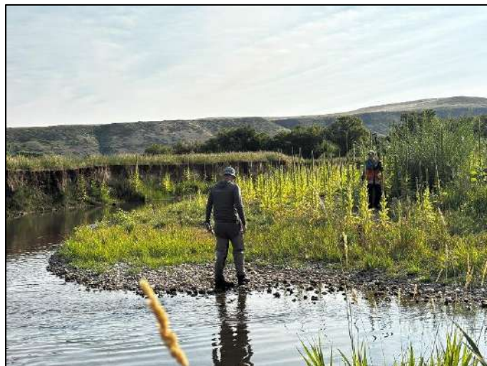
Figure 12. Point bar and floodplain development adjacent to long vertical eroding bank near upstream end of the McKamey Ranch. This is one of the few areas where natural recruitment of willow and cottonwood were observed.
