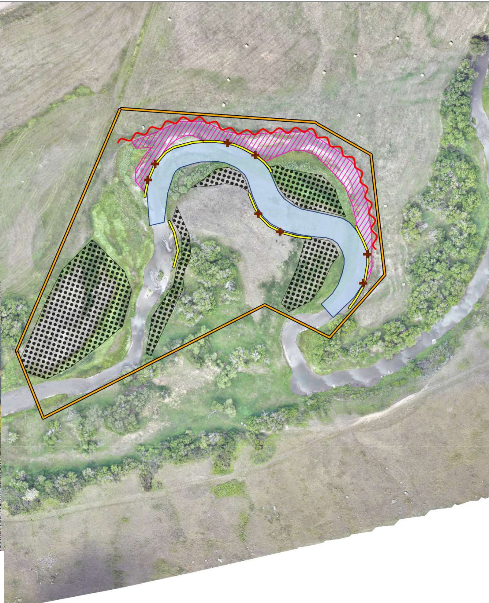
HIGH LATERAL ERODING BANK EXAMPLE PHOTO PHOTO TAKEN ON 8/22/2025 SHOWING THE LATERALLY ERODING BANK IN HOUND CREEK PHASE 1 PROJECT AREA. THIS BANK WOULD BE LAYED BACK AND THE EXISTING CHANNEL SEGMENT WOULD BE ABANDONED AND FILLED TO CREATE CONNECTED FLOODPLAIN.
