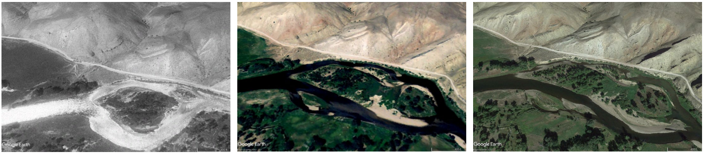
Figure 1. Aerial imagery of the Big Hole River in 1995, 2008, and 2014 showing aggradation of the channel along the northern stream bed.
