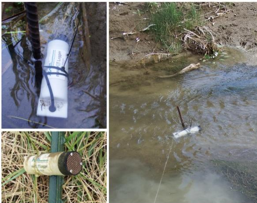
Figure A-3. Dissolved Oxygen Sonde Deployment.
