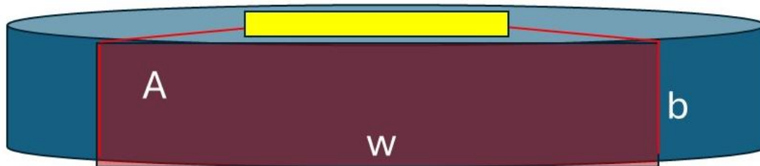
Figure 19: Mixing zone schematic. The yellow rectangle is a RIB, and the blue cylinder is the source specific mixing zone extending from the RIB with a radius of 305 ft. The red box A is the cross-sectional area of a downgradient slice of aquifer, where b is the aquifer thickness and w is an estimate of the width of the mixing zone that will travel to surface water.
