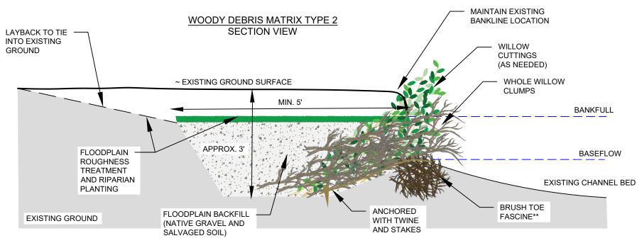
\*\* BRUSH TOE FASCINE CONSTRUCTED WITH BUNDLES OF JUNIPER BRANCHES (OR OTHER) PLACED PARALLEL TO STREAMFLOW AND ANCHORED BENEATH WHOLE WILLOW CLUMPS USING BIODEGRADABLE TWINE AND 2FT WOODEN STAKES
