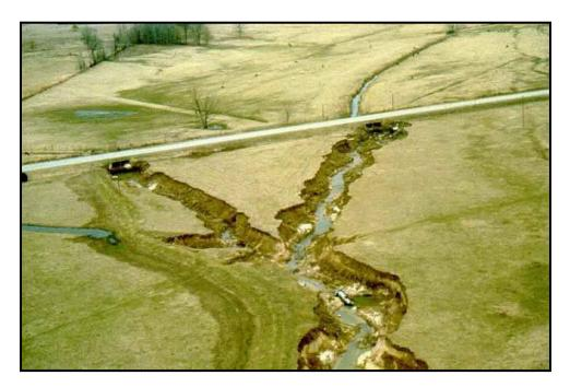
Figure 17. Stream downcutting caused by channelization downstream; the headcuts migrated upstream until intercepted by a road culvert.
