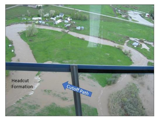
Figure 20. Example meander cutoff during a May 2008 flood on the East Gallatin River in Bozeman (DNRC).
