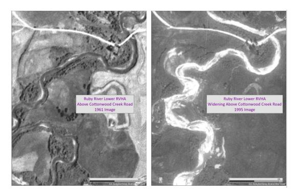
Figure 21. Channel widening between 1961 (left) and 1995 (right) attributed to 1984 flood.
