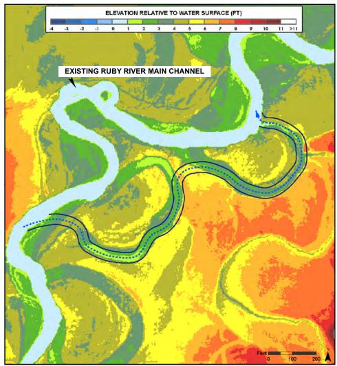
The design realignment path of Main Channel Relocation #1
