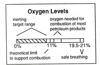
**Test with an Oxygen Indicator -** to measure the effectiveness of the inerting procedure.
