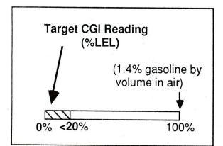
Test with a Combustible Gas Indicator (CGI) - to measure the reduction in the concentration of flammable vapors when purging:
