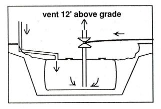
take into account the size of the vent opening as well as the rate at which air is pumped into the tank.
