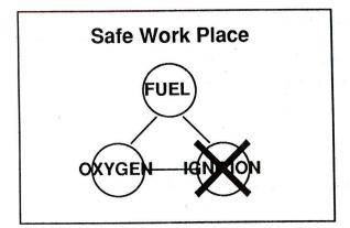
**PREPARE A SAFE WORK PLACE** - before the tank is approached or excavation begins.
