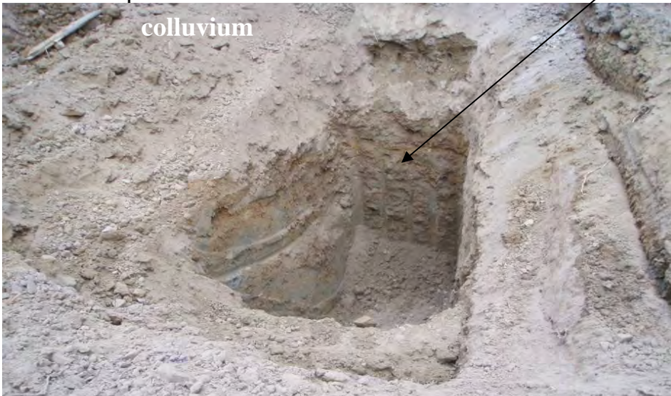
Photo 3: 09-SGTP-3 looking North. Highly weathered diorite in the test pit.
