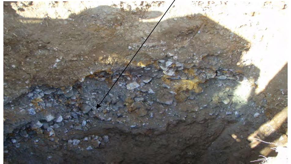
Photo 4: 09-MHTP-3 Looking West into the test pit. Gray layer is flotation tailings from the impoundment.
