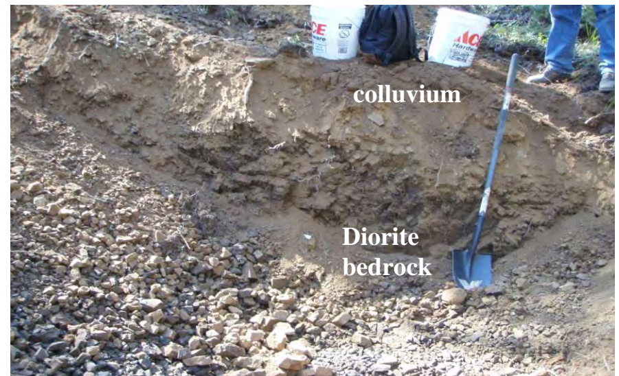
Photo 8: 09-PMTP-8 looking west. Pit located adjacent to diorite outcrop on west side of site.
