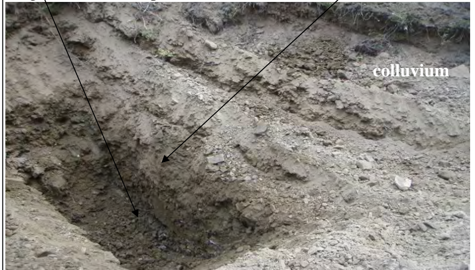
Photo 6: 09-SGTP-6 looking Southerly. Weathered diorite and argillite in the test pit.
