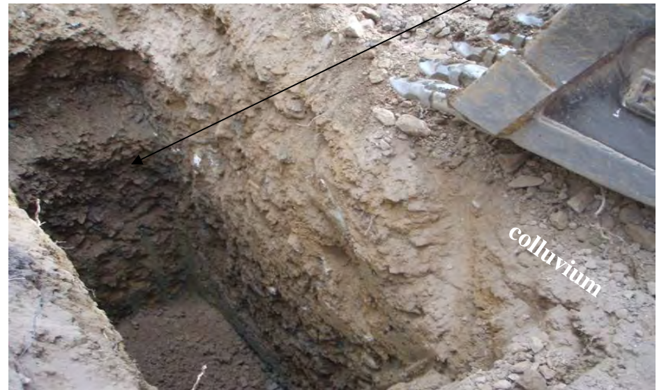
Photo 4: 09-SGTP-4 looking East. Weathered diorite in the test pit.
