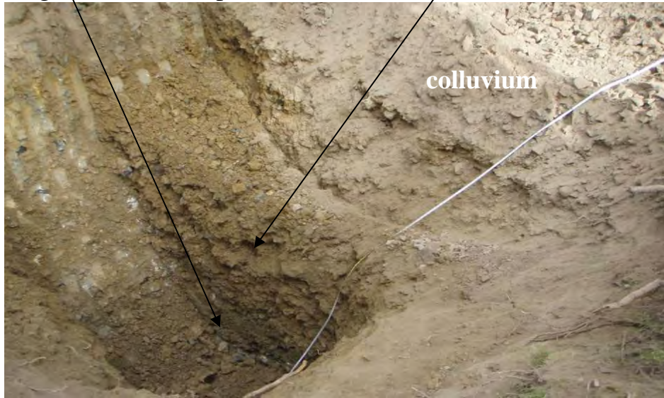
Photo 5: 09-SGTP-5 looking North. Weathered diorite and argillite in the test pit.
