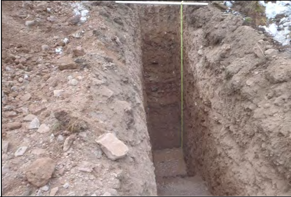
Picture # - 37 Description - S35TP-111. Final Excavation Depth at 18.7'. Water Flowing out of Sand and Gravel Layer from 16' to 17' Date - October 3, 2012 Project - Section 35 Repository Design Investigation
