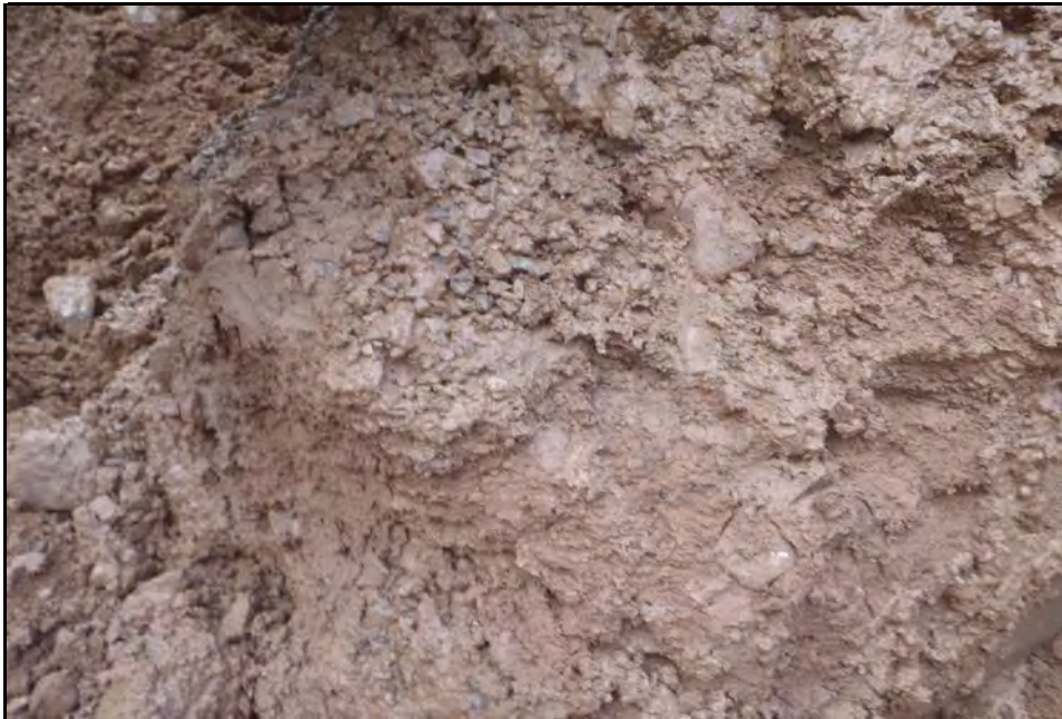
Picture # - 38 Description - S35TP-111. Excavated Wet Sand and Gravel from 16' to 17' Date - October 3, 2012 Project - Section 35 Repository Design Investigation
