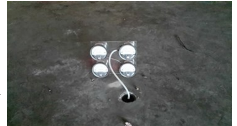
Vacuum influence monitoring equipment set up on soil vapor probe during SVE well testing.
