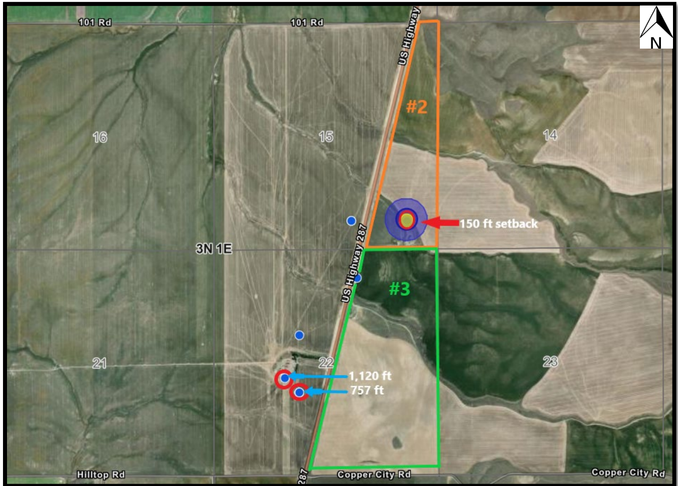
Figure 8: Location of Nearby Groundwater Production Wells Sites #2, #3 (Abandoned GWIC wells in blue, active GWIC wells circled in red, approximate Site #2 in orange, approximate Site #3 in green, distance from Sites #2, #3 to GWIC wells within 1-mile radius)
