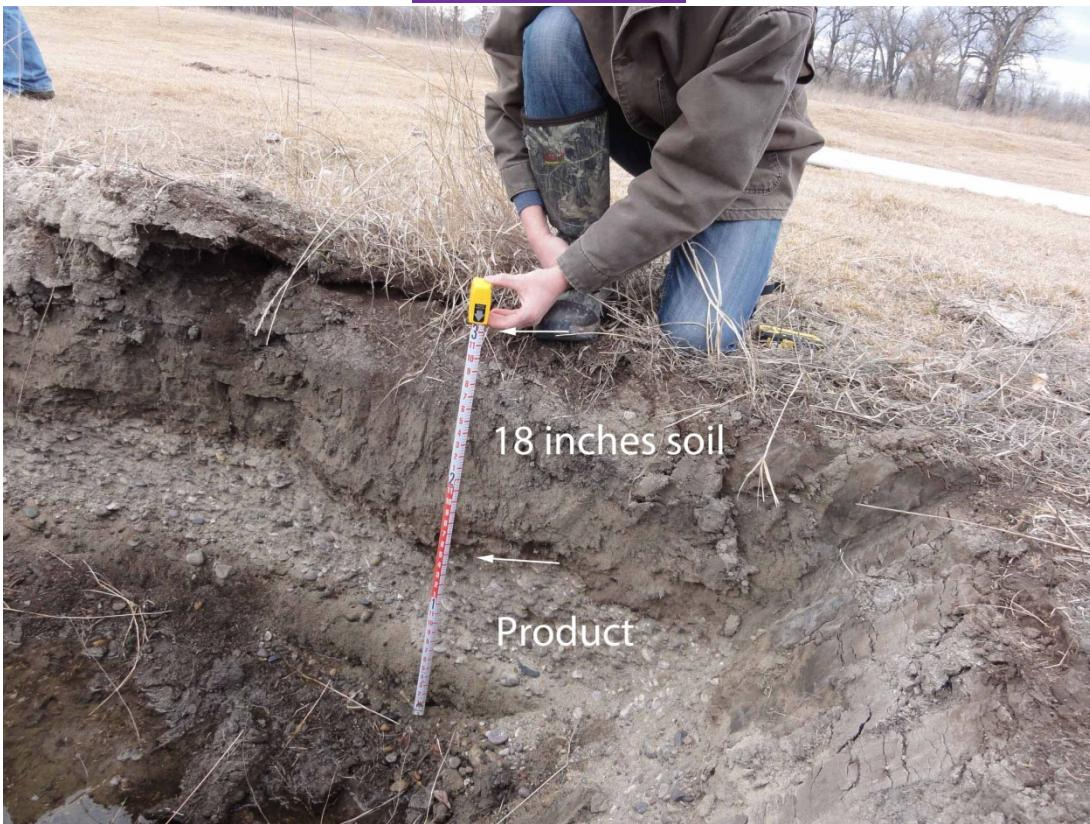
Clear, discernible soil profile. Tick marks on Tape Measure can be clearly identified and tape measure extends 3 feet.
