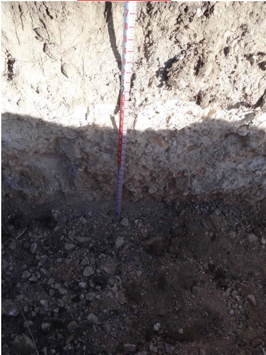
Top 3 feet of soil test pit is not shown and soil profile is washed out due to poor lighting, making the soil profile indiscernible.
