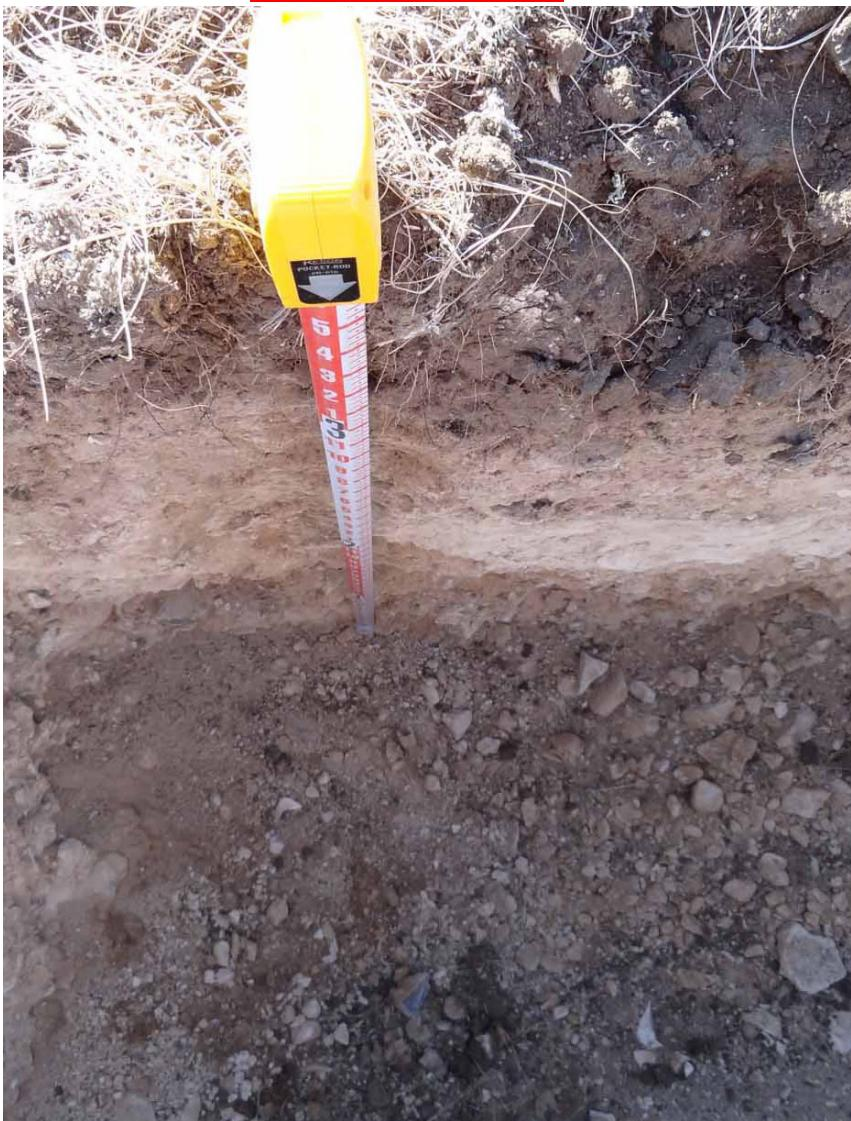
Angle looking down on soil profile is too steep to identify soil characteristics or utilize scale accurately.
