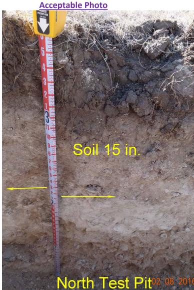
Scale and soil profile is clear and readable. Top three feet of soil profile is shown.
