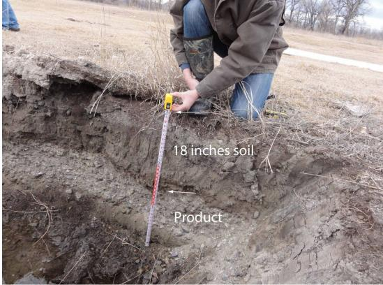
Clear, discernable soil profile. Tick marks on Tape Measure can be clearly identified and tape measure extends 3 feet.
