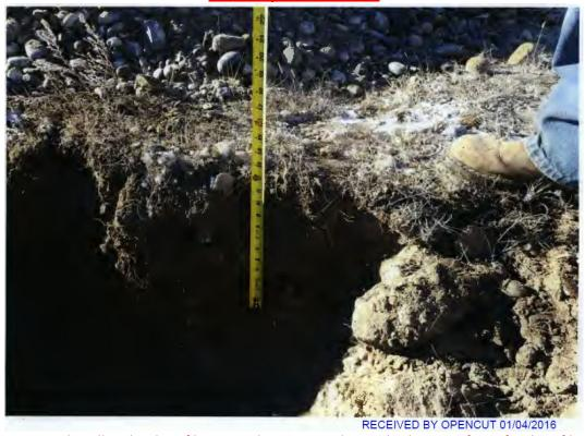
Shadow covers test pit sidewall and soil profile cannot be seen. Scale not displaying 3 feet of soil profile.
