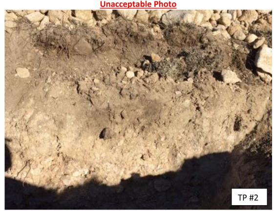
No scale in photo & shadow obscuring portion of test pit sidewall.
