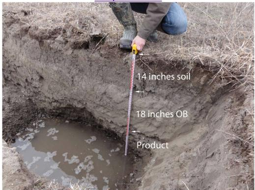
Clear, discernable soil profile. Tick marks on Tape Measure can be clearly identified and tape measure extends 3'+.
