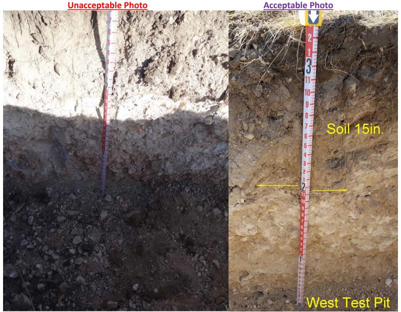
Top 3 feet of soil test pit is not shown and soil profile is washed out due to poor lighting, making the soil profile indiscernible.
