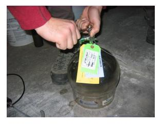
Double check that the Summa canister is tightly closed and remove the shroud. Use the wrenches to remove the flow controller from the canister and replace the brass nut on top of the Summa canister. Remove tubing from the slab by simply pulling it out. Make sure that all relevant information has been documented on the tags on the Summa canister, and that it matches the information on the field forms.
