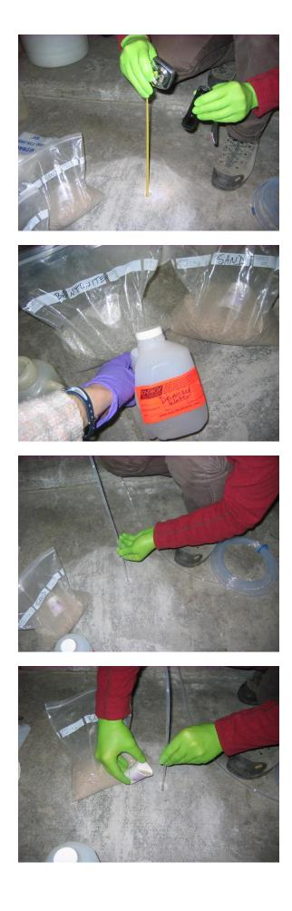
Measure the depth of the hole created beneath the slab and record the slab thickness. A small flashlight is helpful for measuring slab thickness.
