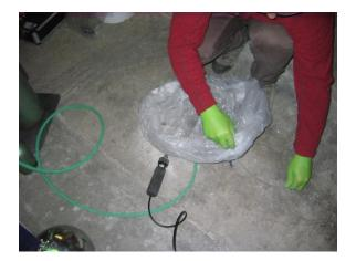
Place the clear plastic shroud (the garbage bag) around the sub-slab sampling point, encompassing the helium canister hose and the helium meter tubing. The end of the sub-slab sampling train Teflon tubing should remain outside of the shroud. Throughout the leak check and sample collection, try not to disturb the seal between the cement mound and the probe tubing in order to maintain the integrity of the seal.
