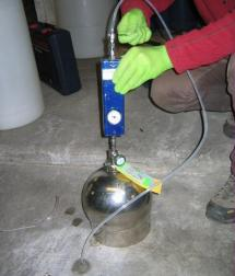
Connect the tubing to the top of the flow controller and tighten firmly using 9/16" and 1/2" wrenches.
