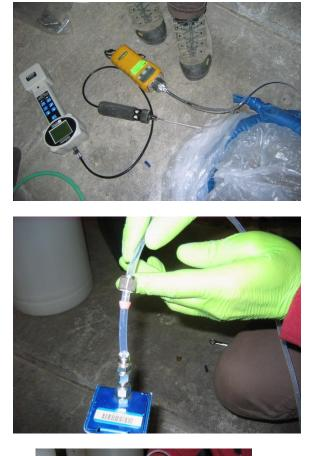
Connect the PID meter to the Teflon tubing sampling train. Allow meter to reach a stable reading and record on the sampling form.
