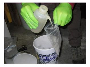
Put away the bentonite. LIGHTLY hydrate the bentonite with the de-ionized water. A pipet or similar may be helpful to avoid adding too much water. The idea is to add just enough water to allow the bentonite to expand and seal the hole, but not so much that it percolates through the bentonite and into the sand below. If water is pulled through the sampling train, it will ruin the sample.
