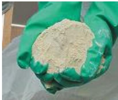
The product is supplied as a dry powder in five-gallon pails with 25 lbs/11.3 kg per pail or in drums with 100 lbs/44.6 kg per drum. PermeOx Ultra will release approximately 18% oxygen by weight over an estimated 12-month period.
