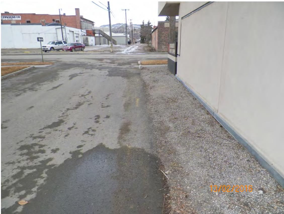
Photo 3. View west across Oak Street showing the powerline location and that of the gas line (yellow stripe) in the middle of the photo. The sanitary sewer line is also buried in the alley.
