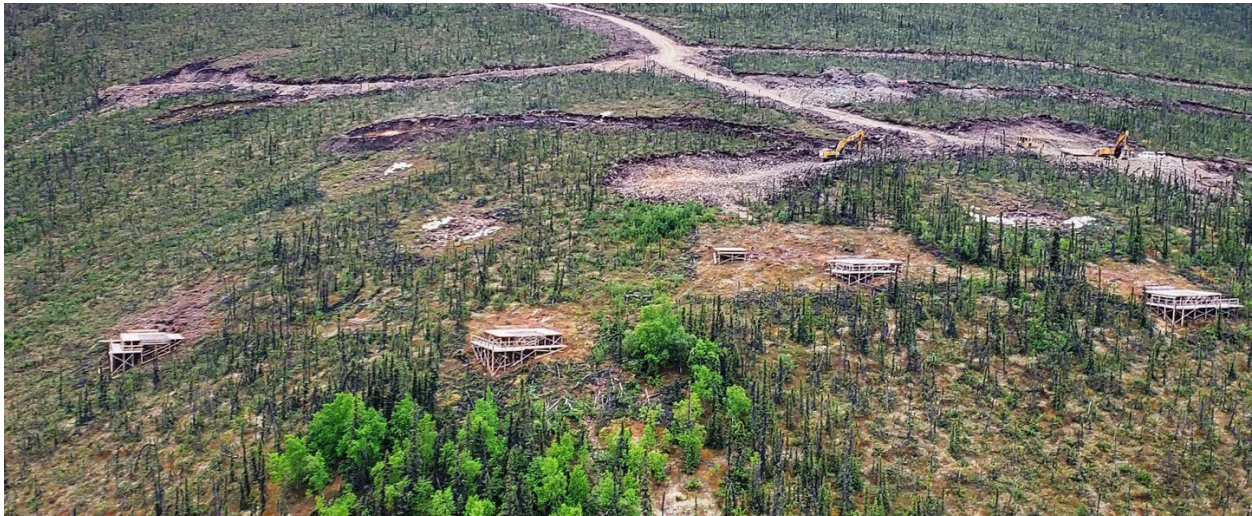
Figure 2-2. Typical Wooden Platforms for Use in Exploration
