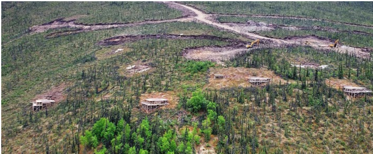
Figure 3. Wooden platform arrangement for drill program.
