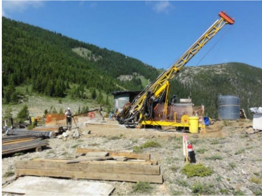
Figure 2. Typical helicopter supported diamond drill rig.
