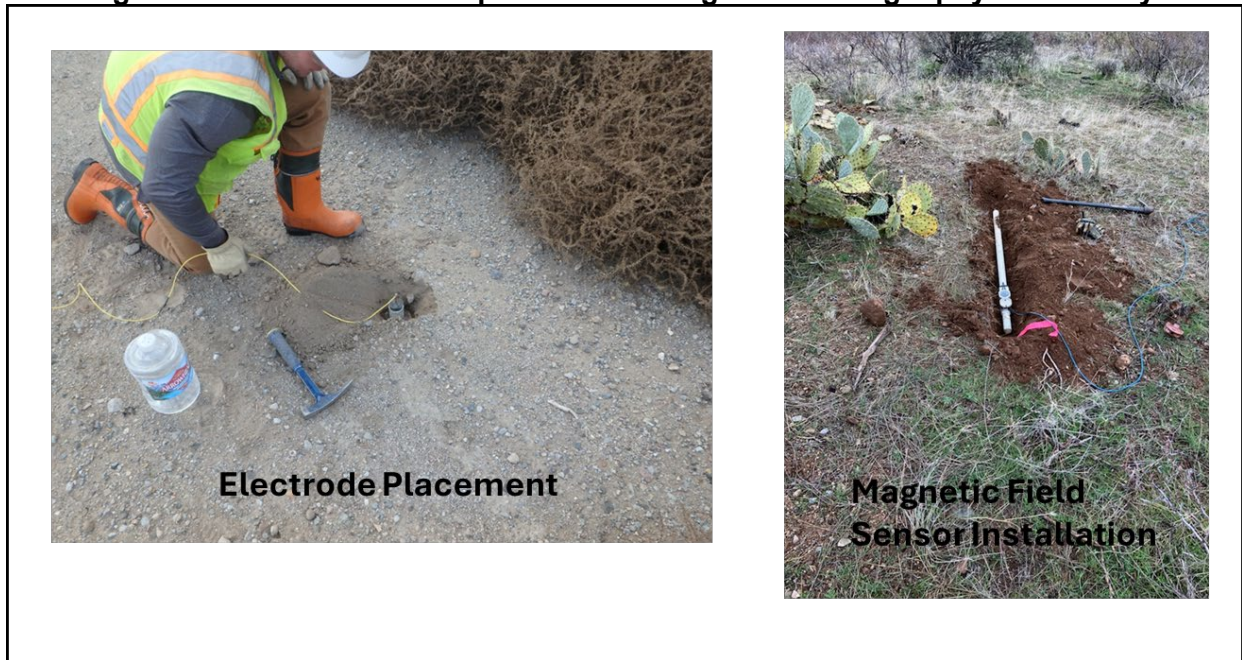
Figure 6: Installation of components of a Mageto Telluric geophysical survey.
