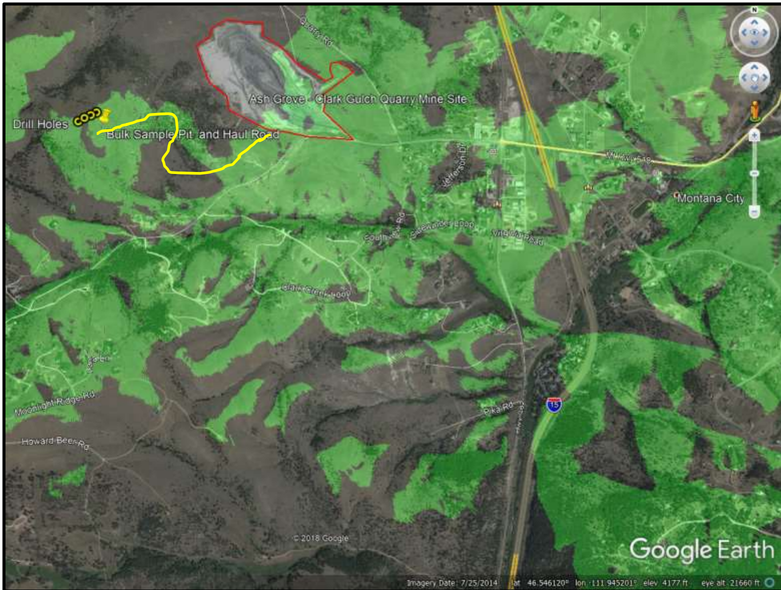
Figure 2: Viewshed Analysis (Google Earth, 2019). Pin represents highest topographic proposed disturbance, which represents the maximum extent of visibility. Green shading represents land that may view project site if a viewer is located at an observation point that is unobstructed by topography or forested vegetation
