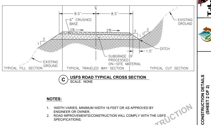
**USFS ROAD TYPICAL CROSS SECTION** SCALE: NONE
