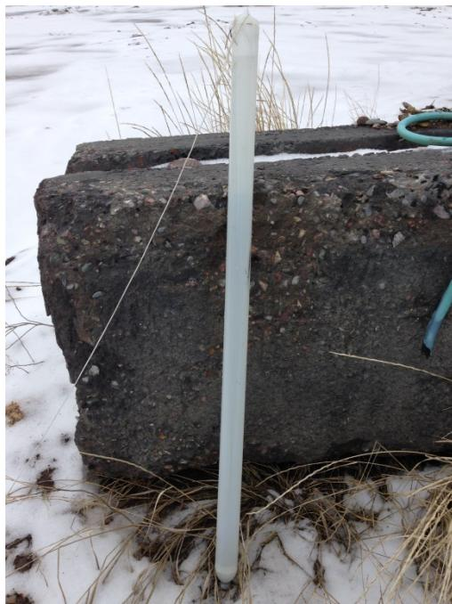
Photo 1. View of upright bailer with MW-11 contents
