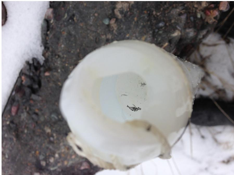
Photo 3. Close-up top view of LNAPL sheen on water surface on surface of bailer
