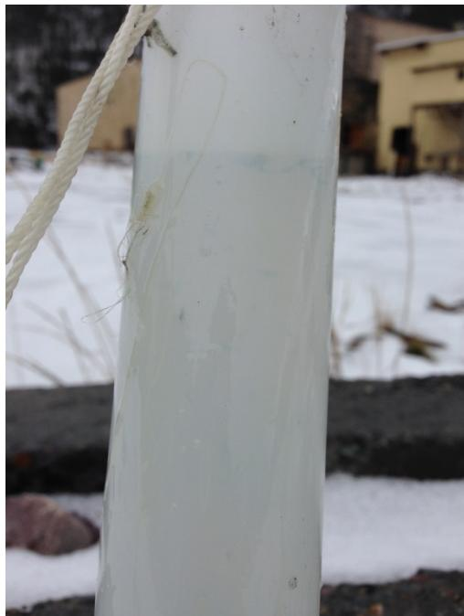
Photo 2. Close-up view of LNAPL sheen on water surface and on surface of bailer
