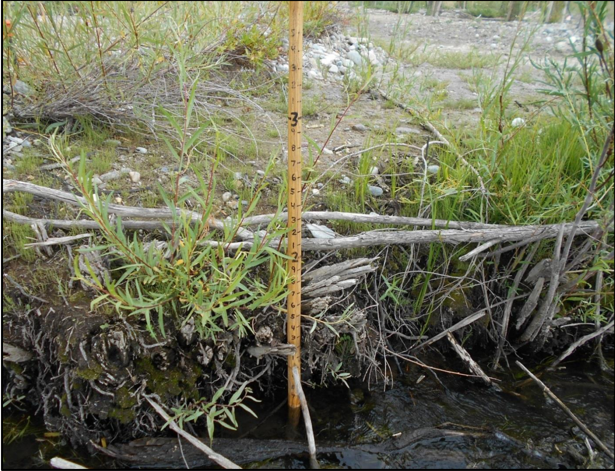
Figure 4-14. View of designed secondary channel elevation at inlet in Phase 1 of the Clark Fork River Operable Unit on August 20, 2014. Mean daily streamflow at the Clark Fork River at Galen site [USGS, 2015b] was 100 cfs on August 20, 2014.
