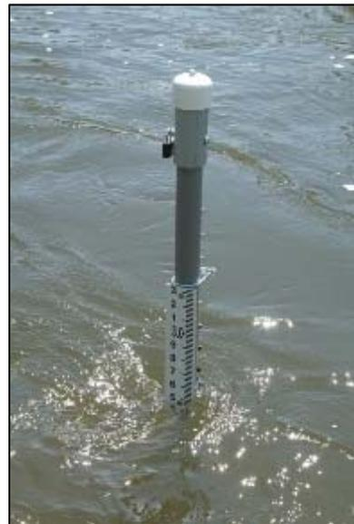
The height of the top of each staff gauge relative to a benchmark established on the nearby bridge deck was determined with a laser level at the time of installation and again at the end of the deployment. These measurements served as controls to determine any vertical shift in the stilling wells and staff gauges over the period of data collection, and are included in **Appendix F-1**.
