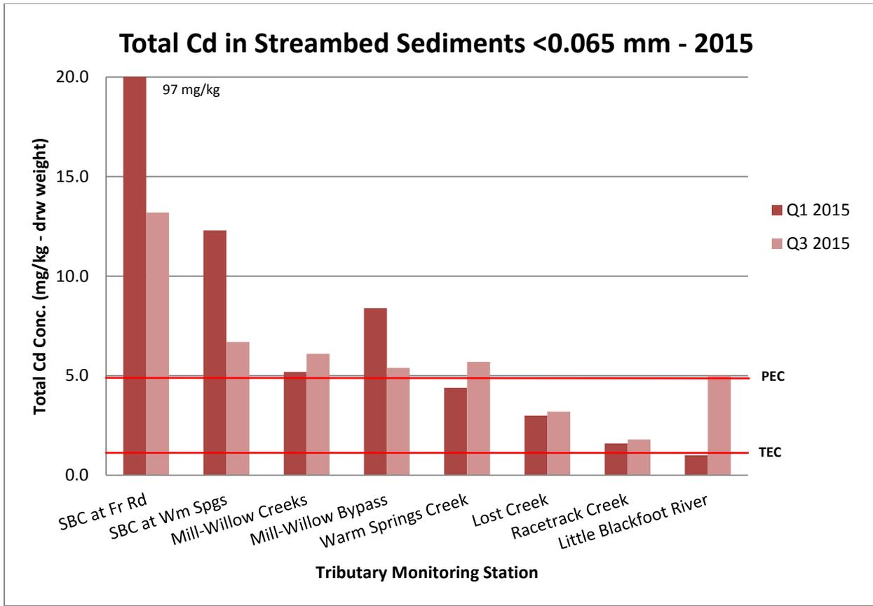
Figure 3-5. Total cadmium (Cd) concentrations (dry weight) in Clark Fork River tributary sediment samples, 2015. Red lines represent the “threshold effect concentration” (TEC) and the “probable effect concentration” (PEC) [MacDonald et al., 2000].
