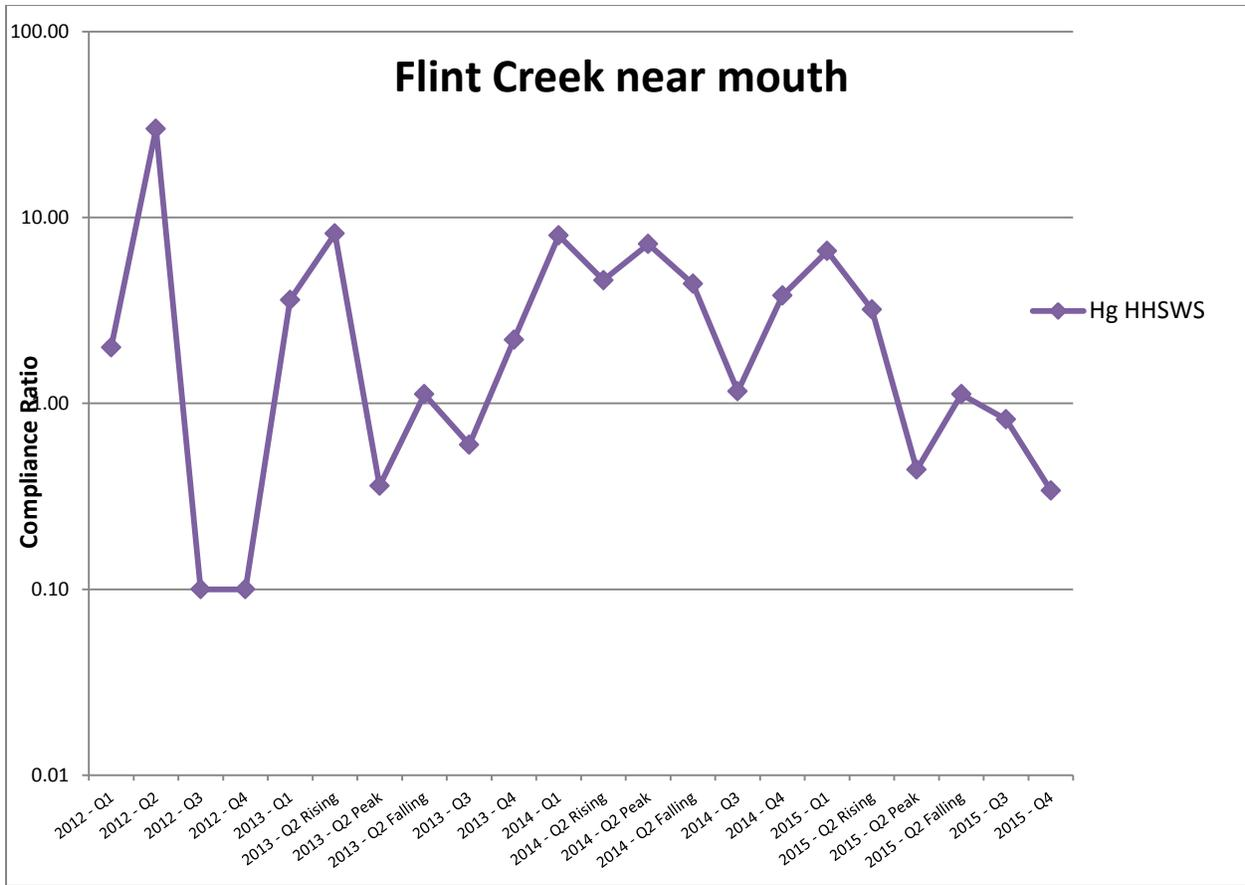
**Figure 2-80. Total mercury (Hg) compliance ratios for the Flint Creek near mouth site, 2012-2015. Compliance ratios are based on the human health surface water standard (HHSWS) [MDEQ, 2012b].**
