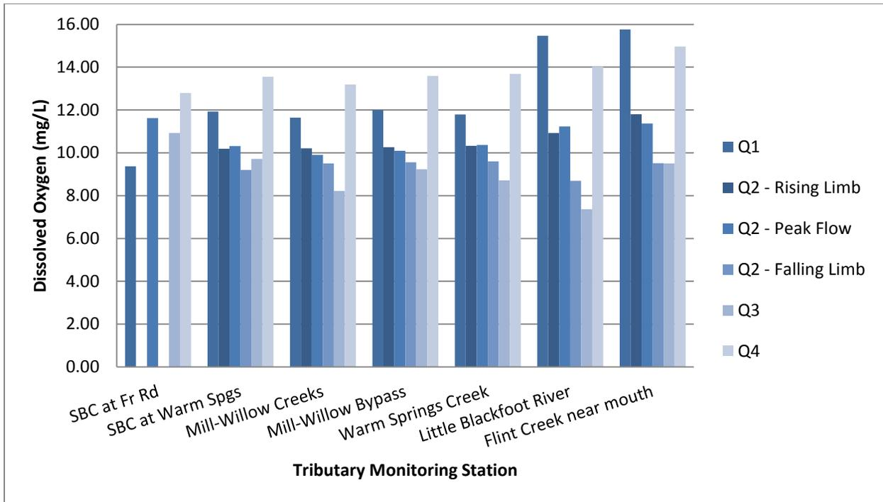
Figure 2-15. Dissolved oxygen concentrations at tributary sampling sites in the Clark Fork River Operable Unit, 2015. No samples were collected during the Q2-Rising Limb and Q2-Falling Limb monitoring periods at the “SBC at Fr Rd” site.
