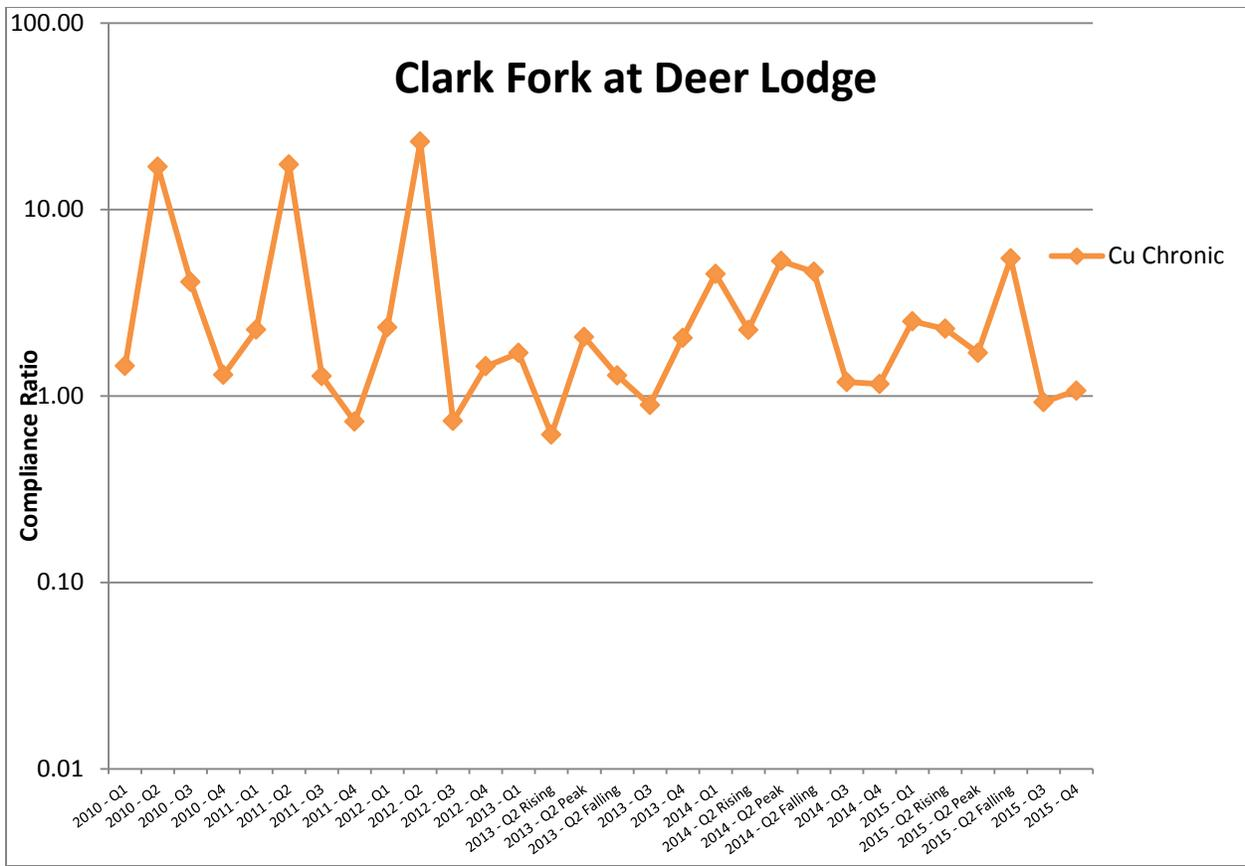
**Figure 2-55. Total recoverable copper (Cu) compliance ratios for the Clark Fork River at Deer Lodge site, 2010-2015. Compliance ratios are based on the chronic aquatic life standard [MDEQ, 2012b].**
