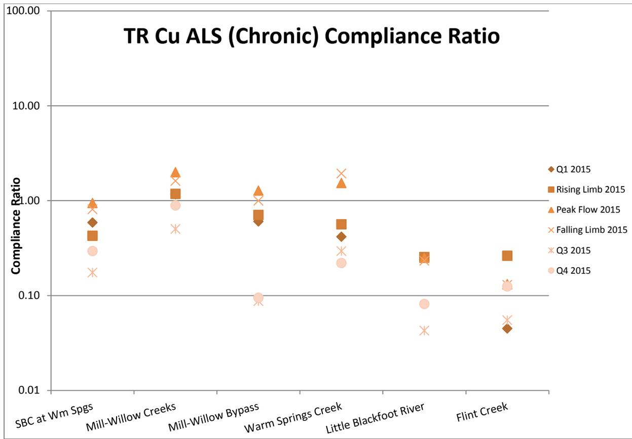
**Figure 2-62. Total recoverable copper (TR Cu) compliance ratios for the Clark Fork River tributary sites, 2015. Compliance ratios are based on the chronic aquatic life standard (ALS) [MDEQ, 2012b].**
