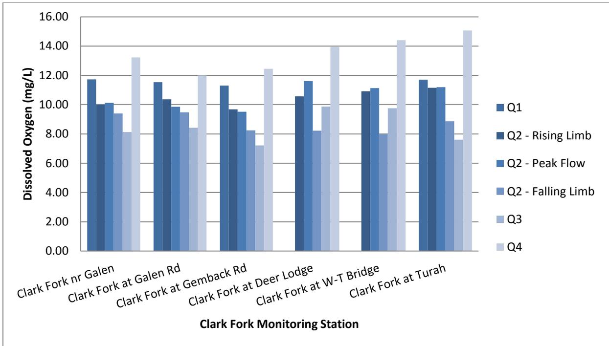
Figure 2-13. Dissolved oxygen concentrations at mainstem sampling sites in the Clark Fork River Operable Unit, 2015.
