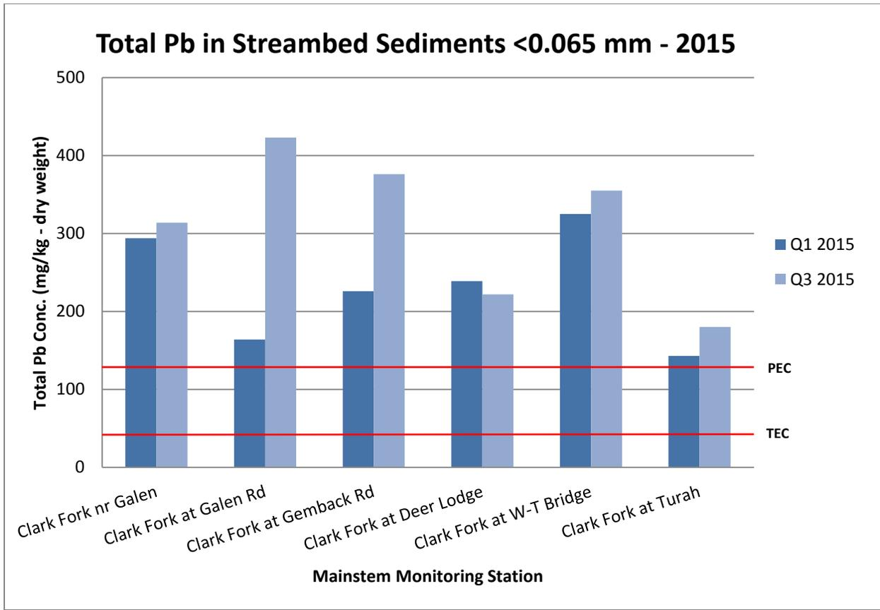
**Figure 3-8. Total lead (Pb) concentrations (dry weight) in Clark Fork River mainstem sediment samples, 2015. Red lines represent the “threshold effect concentration” (TEC) and the “probable effect concentration” (PEC) [MacDonald et al., 2000].**
