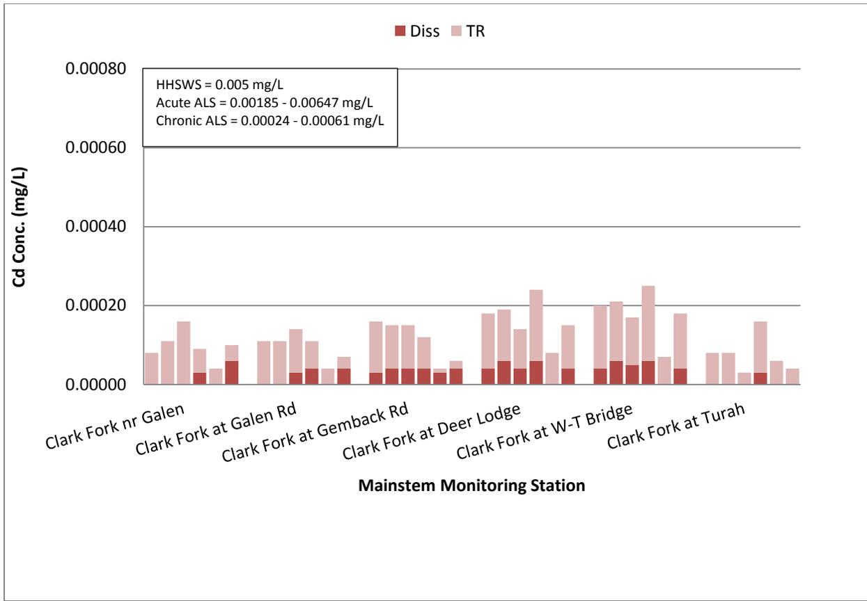
**Figure 2-45. Total recoverable (TR) and dissolved (Diss) cadmium (Cd) concentrations at mainstem sampling sites in the Clark Fork River Operable Unit, 2015. Applicable water quality standards are the aquatic life standards (ALS) and the human health surface water standard (HHSWS) [MDEQ, 2012b].**
