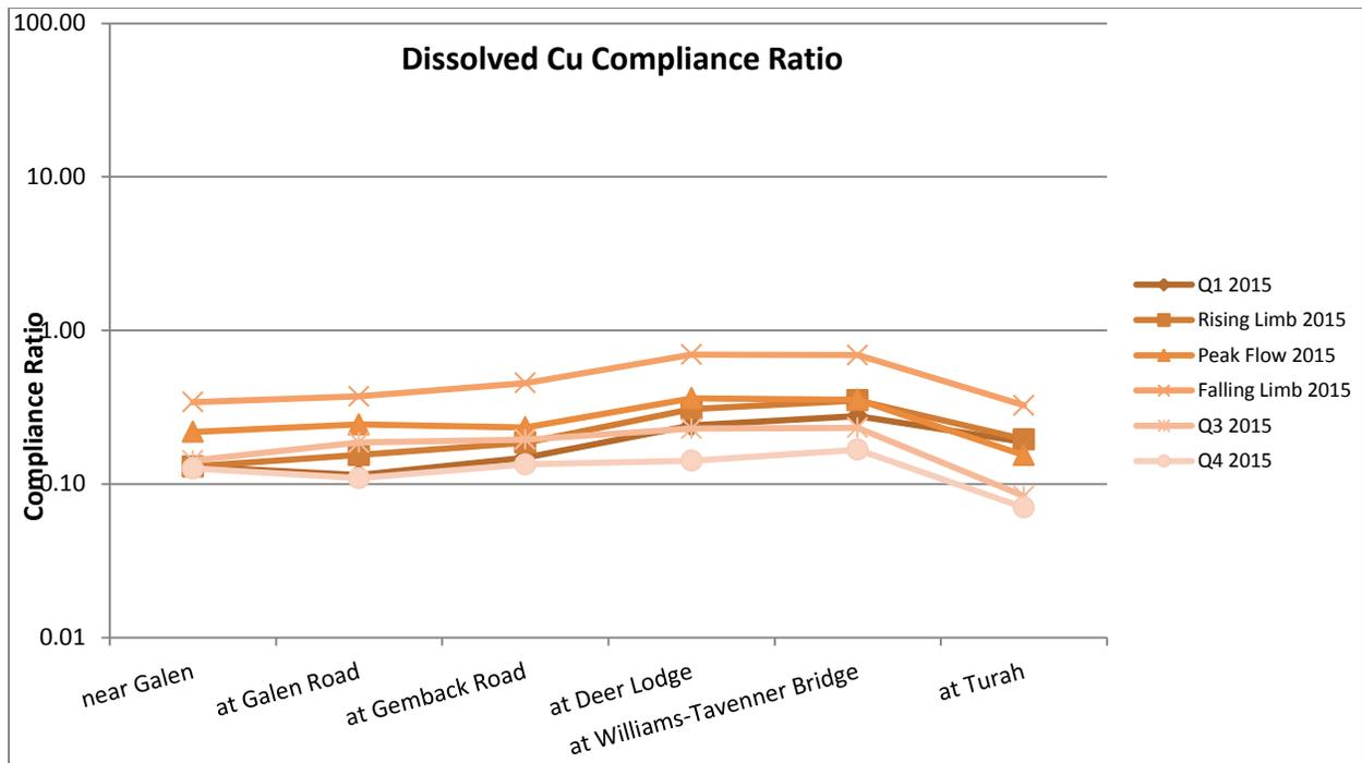
**Figure 2-57. Dissolved copper (Cu) compliance ratios for the Clark Fork River mainstem sites, 2015. Compliance ratios are based on the federal ambient water quality criteria [USEPA, 1986].**
