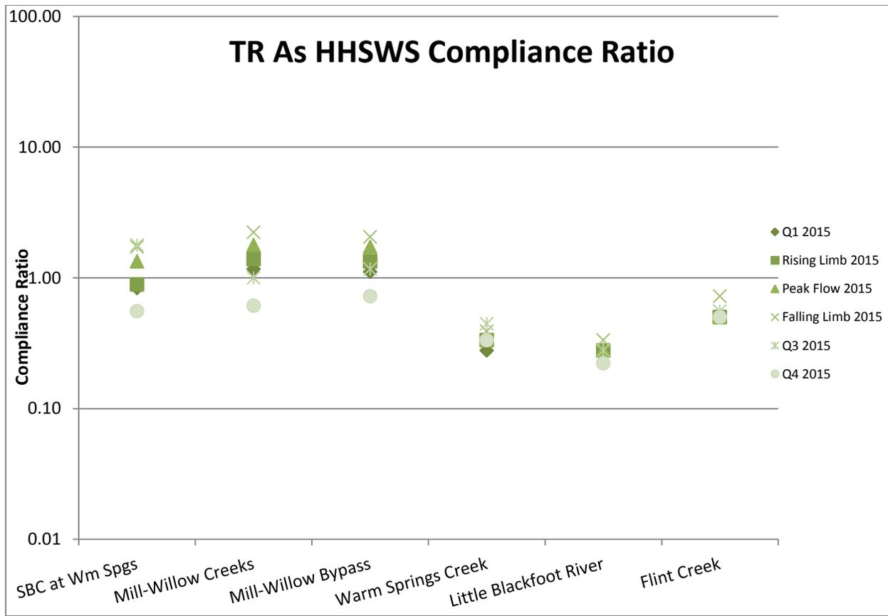
**Figure 2-44. Total recoverable arsenic (TR As) compliance ratios for the Clark Fork River tributary sites, 2015. Compliance ratio is based on Clark Fork River Operable Unit Record of Decision performance goal for total recoverable arsenic (TR As HHSWS) concentration [USEPA, 2004].**
