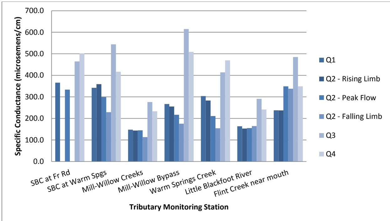
**Figure 2-12. Conductivity at tributary sampling sites in the Clark Fork River Operable Unit, 2015. No samples were collected during the Q2-Rising Limb and Q2-Falling Limb monitoring periods at the “SBC at Fr Rd” site.**
