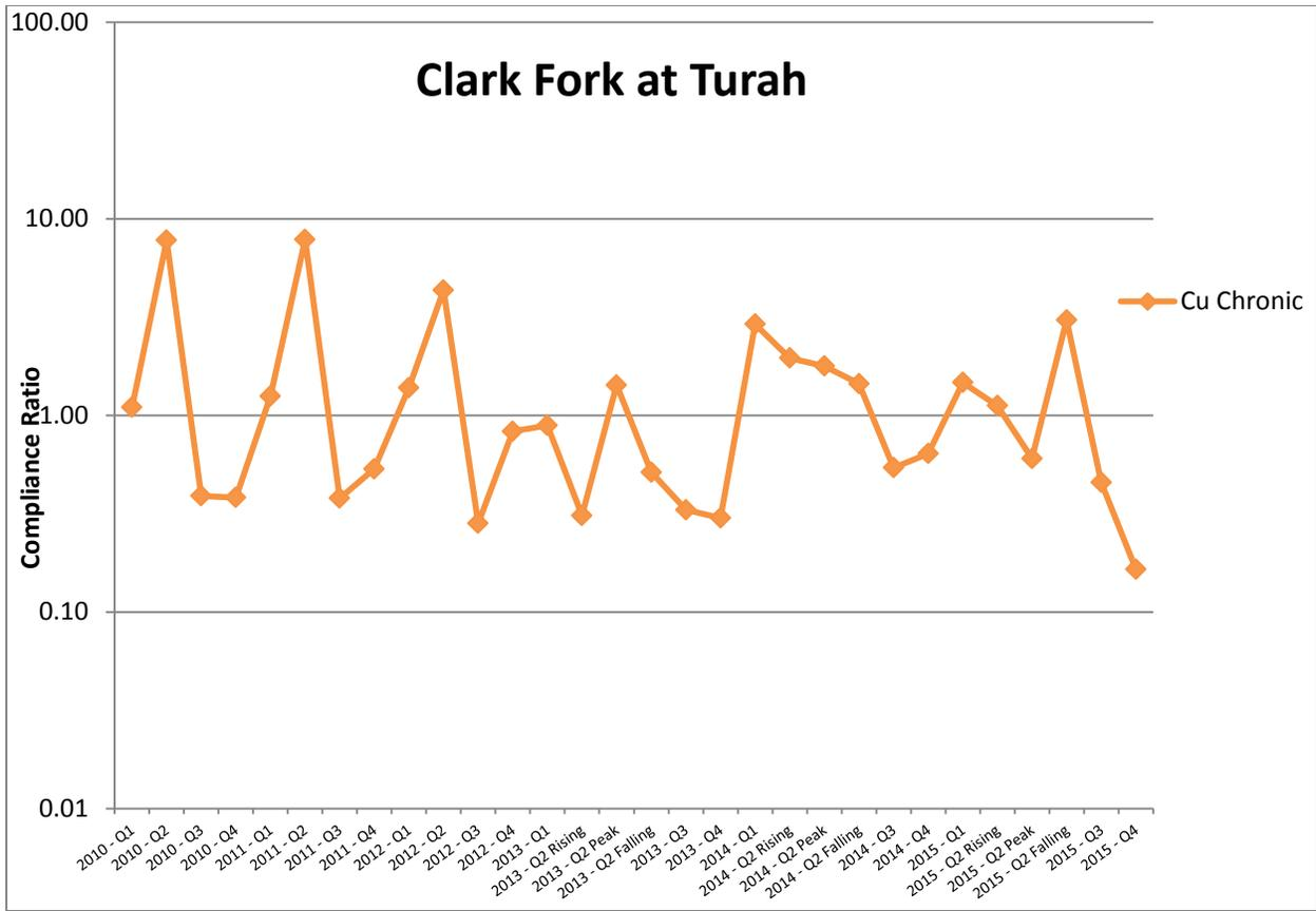
**Figure 2-56. Total recoverable copper (Cu) compliance ratios for the Clark Fork River at Turah site, 2010-2015. Compliance ratios are based on the chronic aquatic life standard [MDEQ, 2012b].**
