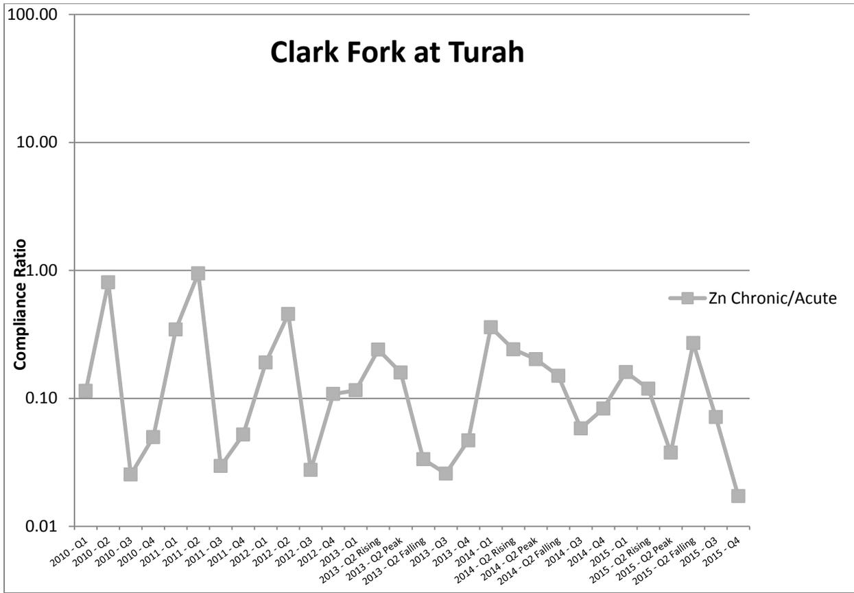
**Figure 2-74. Total recoverable zinc (Zn) compliance ratios for the Clark Fork River at Turah site, 2010-2015. Compliance ratios are based on the aquatic life standard [MDEQ, 2012b].**
