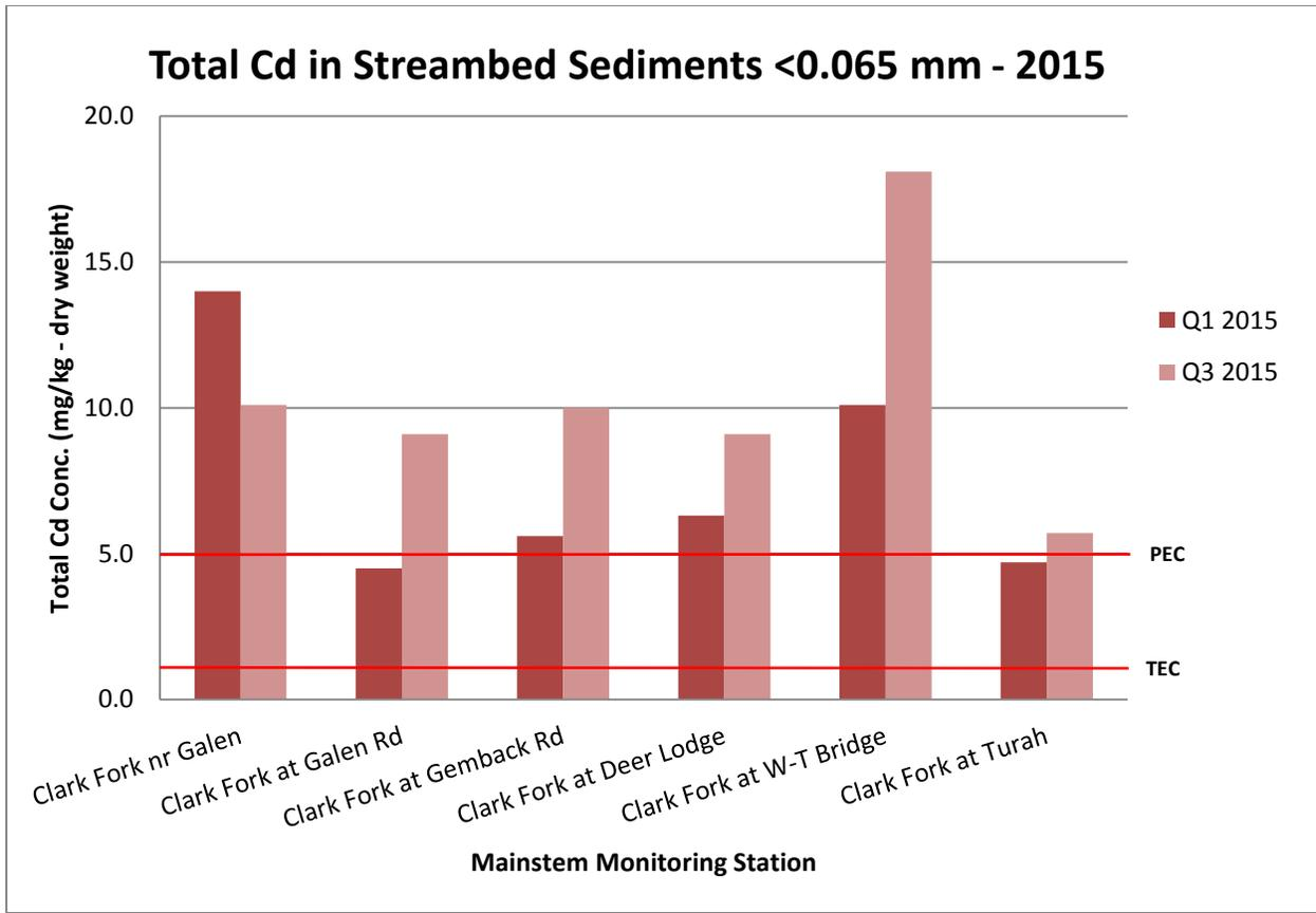
**Figure 3-4. Total cadmium (Cd) concentrations (dry weight) in Clark Fork River mainstem sediment samples, 2015. Red lines represent the “threshold effect concentration” (TEC) and the “probable effect concentration” (PEC) [MacDonald et al., 2000].**
