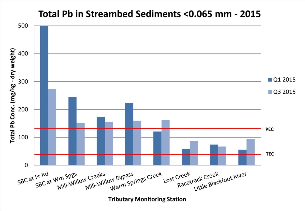
**Figure 3-9. Total lead (Pb) concentrations (dry weight) in Clark Fork River tributary sediment samples, 2015. Red lines represent the “threshold effect concentration” (TEC) and the “probable effect concentration” (PEC) [MacDonald et al., 2000].**
