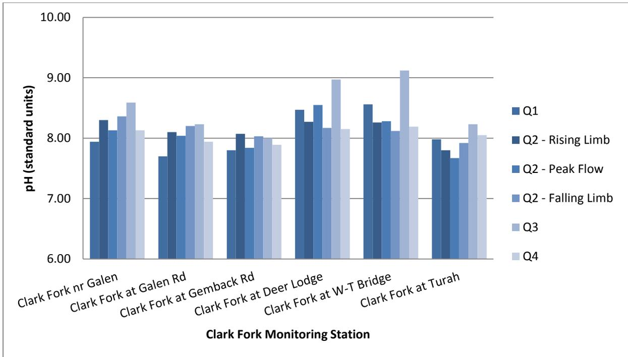
Figure 2-9. Surface water pH at mainstem sampling sites in the Clark Fork River Operable Unit, 2015.
