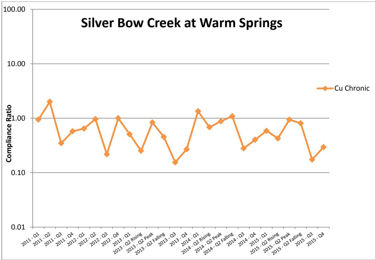
**Figure 2-60. Total recoverable copper (Cu) compliance ratios for the Silver Bow Creek at Warm Springs site, 2011-2015. Compliance ratios are based on the chronic and acute aquatic life standards [MDEQ, 2012b].**
