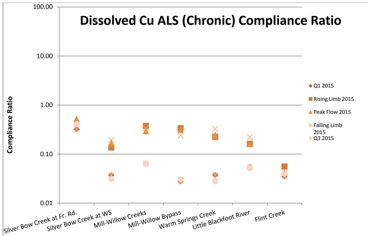
**Figure 2-61. Dissolved copper (Cu) compliance ratios for the Clark Fork River tributary sites, 2015. Compliance ratios are based on the federal ambient water quality criteria [USEPA, 1986]<sup>11</sup>.**
