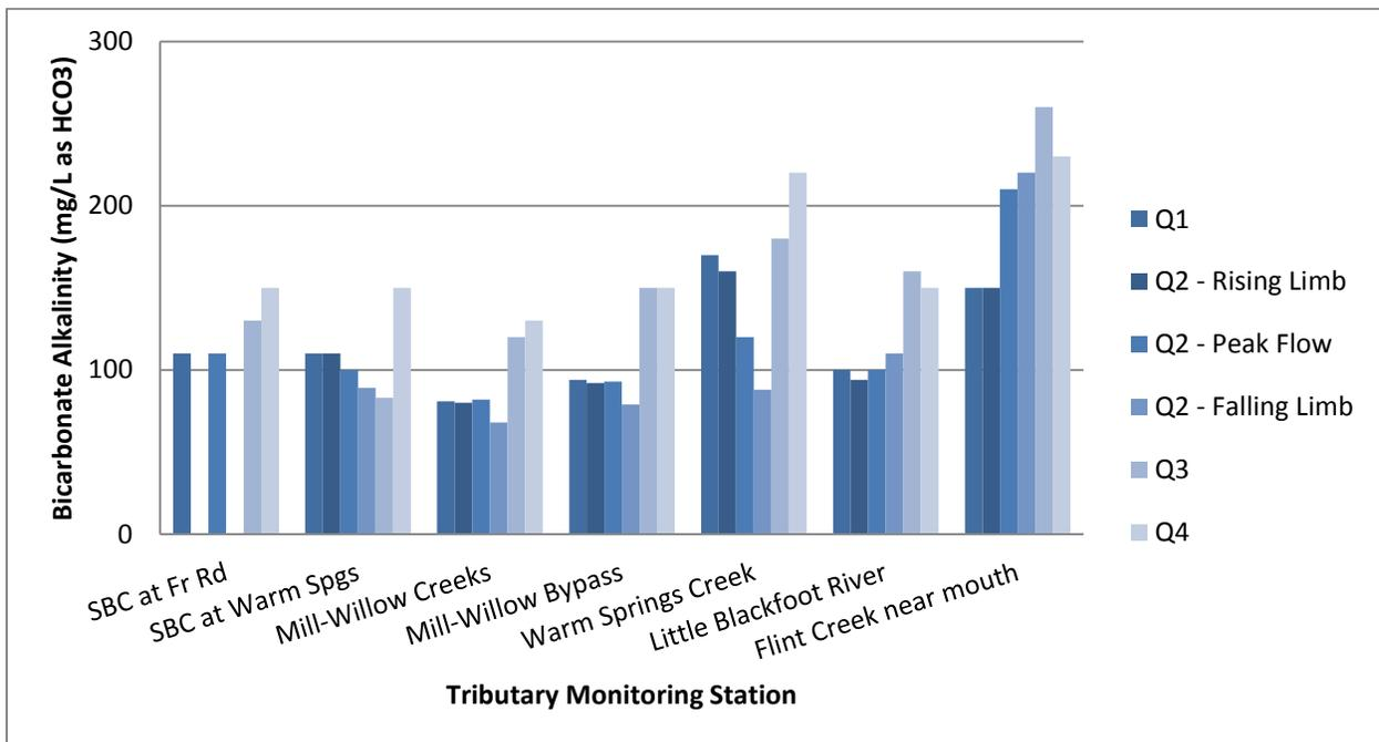
Figure 2-26. Bicarbonate alkalinity at tributary sampling sites in the Clark Fork River Operable Unit, 2015. No samples were collected during the Q2-Rising Limb and Q2-Falling Limb monitoring periods at the “SBC at Fr Rd” site.
