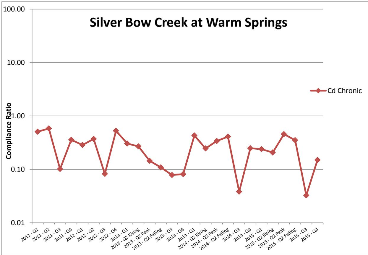
**Figure 2-51. Total recoverable cadmium (Cd) compliance ratios for the Silver Bow Creek at Warm Springs site, 2011-2015. Compliance ratios are based on the chronic aquatic life standard [MDEQ, 2012b].**
