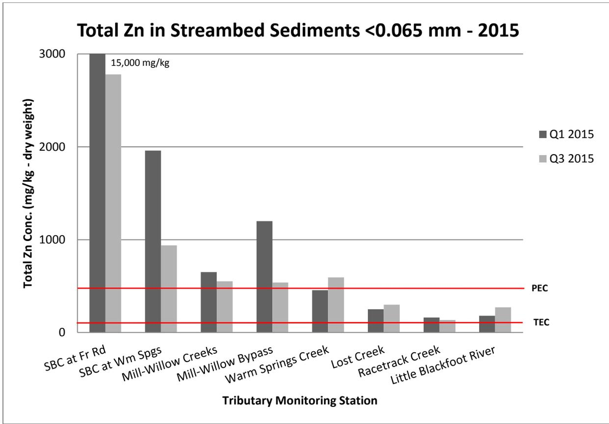
**Figure 3-11. Total zinc (Zn) concentrations (dry weight) in Clark Fork River tributary sediment samples, 2015. Red lines represent the “threshold effect concentration” (TEC) and the “probable effect concentration” (PEC) [MacDonald et al., 2000].**
