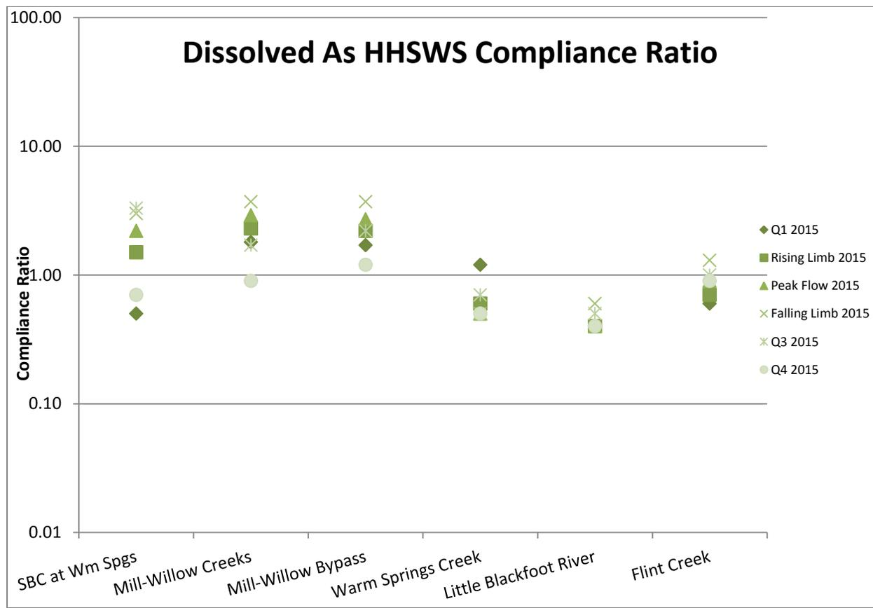
**Figure 2-43. Dissolved arsenic (As) compliance ratios for the Clark Fork River tributary sites, 2015. Compliance ratio is based on Clark Fork River Operable Unit Record of Decision performance goal for dissolved arsenic (Dissolved As HHSWS) concentration [USEPA, 2004].**
