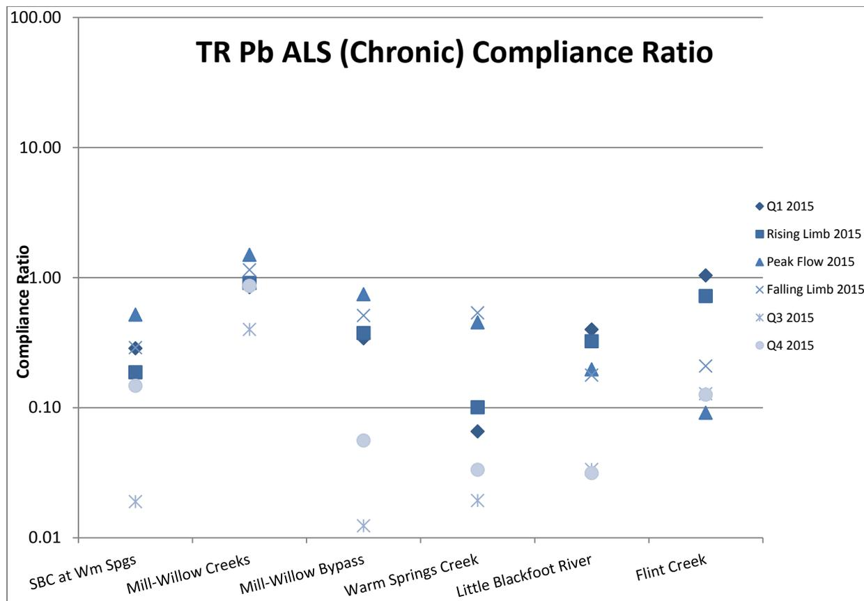
Figure 2-70. Total recoverable lead (TR Pb) compliance ratios for the Clark Fork River tributary sites, 2015. Compliance ratios are based on the chronic aquatic life standard (ALS) [MDEQ, 2012b].
