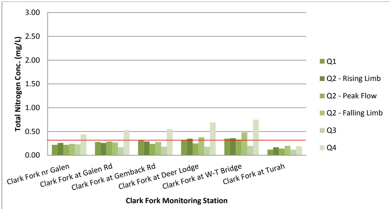
Figure 2-29. Total nitrogen concentrations (mg/L) at Clark Fork River mainstem monitoring stations, 2015. Red line represents total nitrogen standard [MDEQ, 2014].
