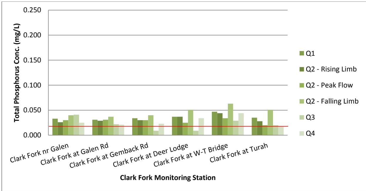
Figure 2-33. Total phosphorus concentrations (mg/L) at Clark Fork River mainstem monitoring stations, 2015. Red line represents total phosphorus standard [ARM 17.30.631].
