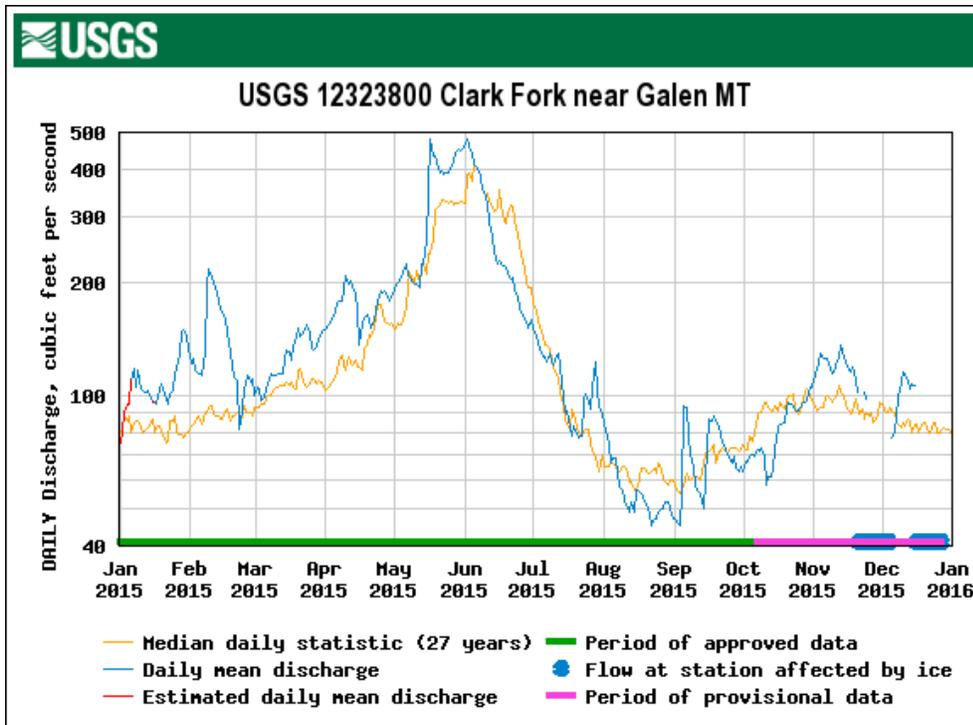
Figure 2-3. Hydrograph for Clark Fork near Galen, 2015.
