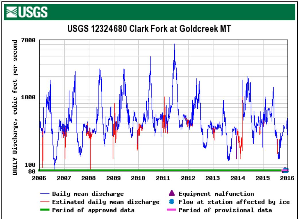
Figure 7-17. USGS hydrograph from the Clark Fork River gauge near Goldcreek.
