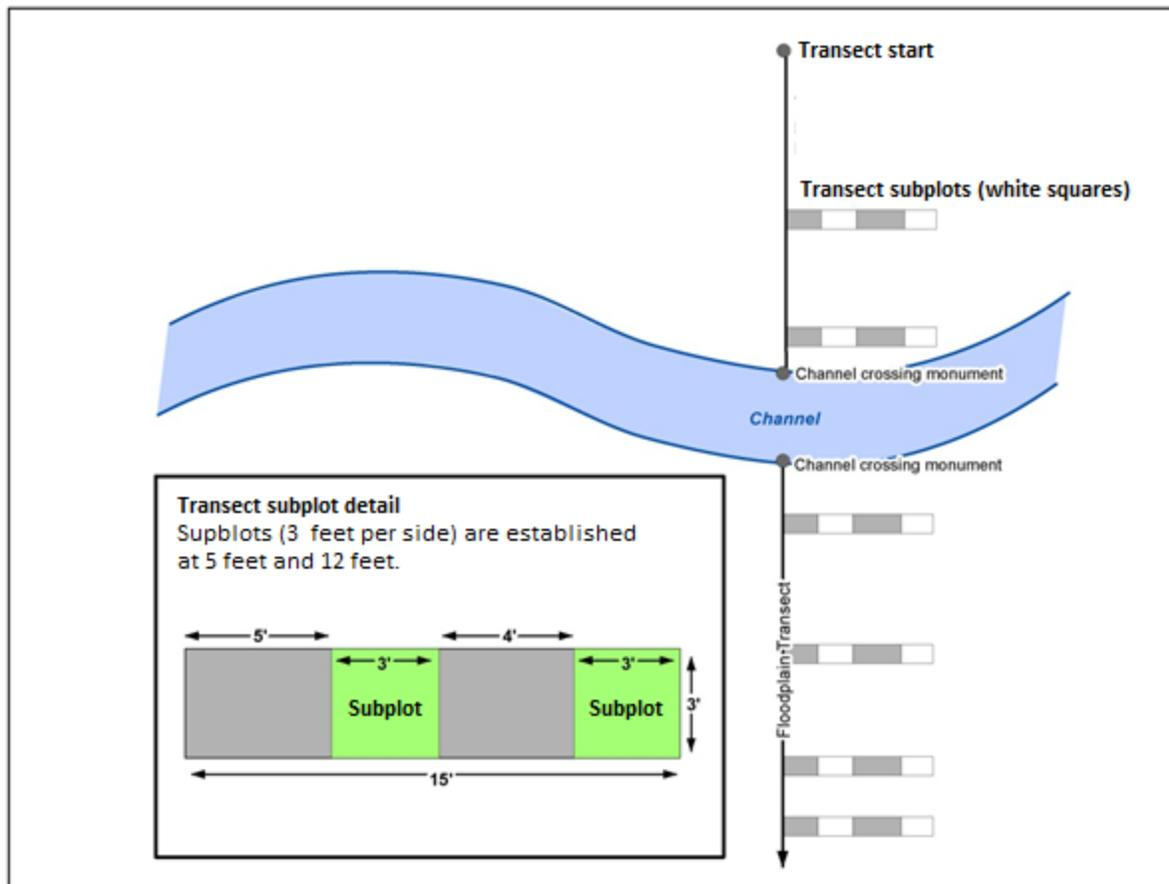
**Figure 4-3. Schematic of floodplain transect sampling design for Phase 1 of the Clark Fork River Operable Unit (figure adapted from Sacry et al. [2012]). Floodplain transect and subplot locations determined by Sacry et al. [2012].**
