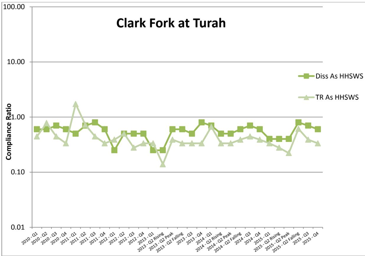
**Figure 2-38. Total recoverable (TR) and dissolved (Diss) arsenic (As) compliance ratios for the Clark Fork River at Turah site, 2010-2015. Compliance ratios are based on the Clark Fork River Operable Unit Record of Decision performance goals for dissolved (Diss As HHSWS) and total recoverable (TR As HHSWS) arsenic concentrations [USEPA, 2004].**
