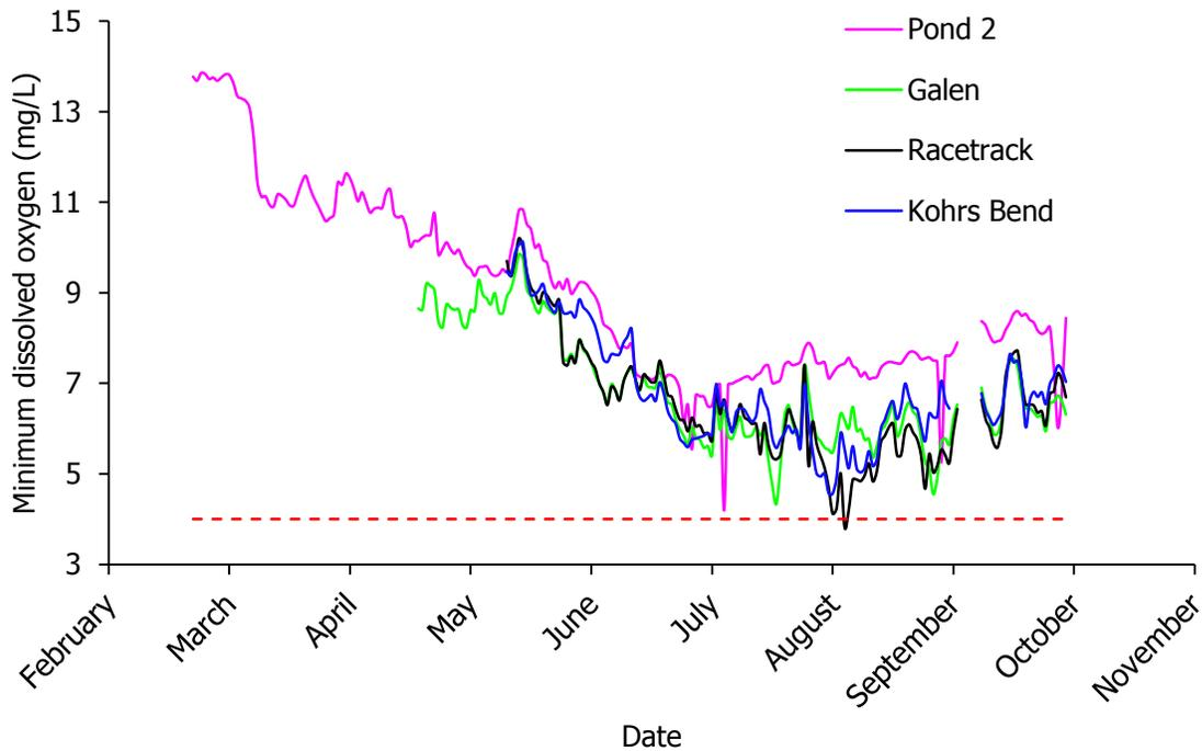
**Figure 7-16. Minimum daily dissolved oxygen concentrations at 2015 caged fish sites. The red dashed horizontal line denotes the freshwater ALS one day minimum.**
