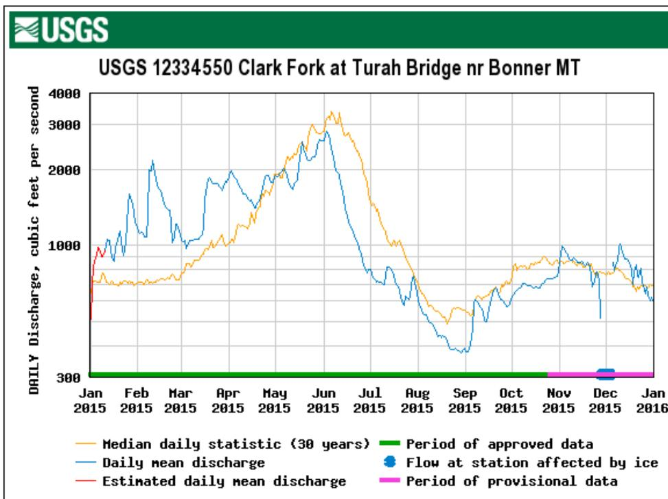
Figure 2-6. Hydrograph for Clark Fork at Turah Bridge, 2015.
