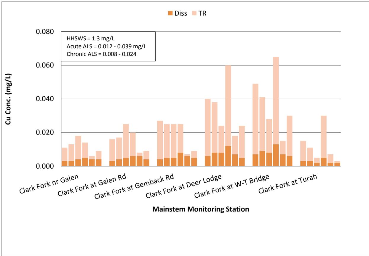
**Figure 2-53. Total recoverable (TR) and dissolved (Diss) copper (Cu) concentrations at mainstem sampling sites in the Clark Fork River Operable Unit, 2015. Applicable water quality standards are the aquatic life standards (ALS) and the human health surface water standard (HHSWS) [MDEQ, 2012b].**
