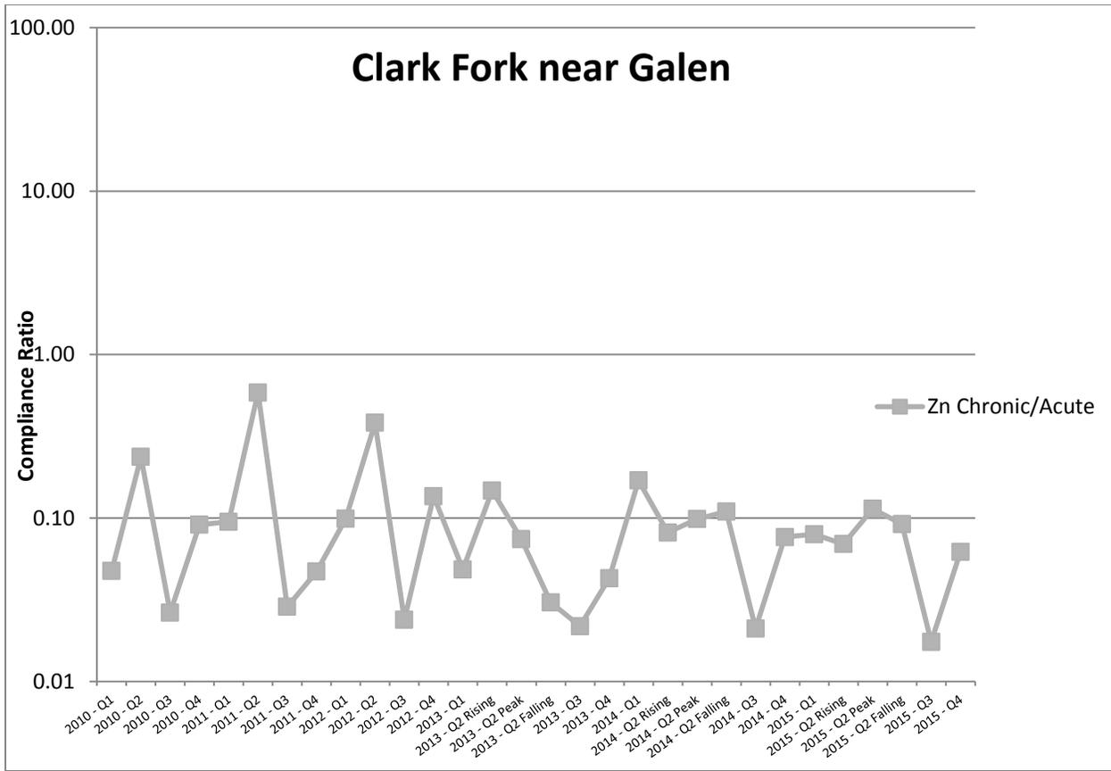
**Figure 2-72. Total recoverable zinc (Zn) compliance ratios for the Clark Fork River near Galen site, 2010-2015. Compliance ratios are based on the aquatic life standard [MDEQ, 2012b].**
