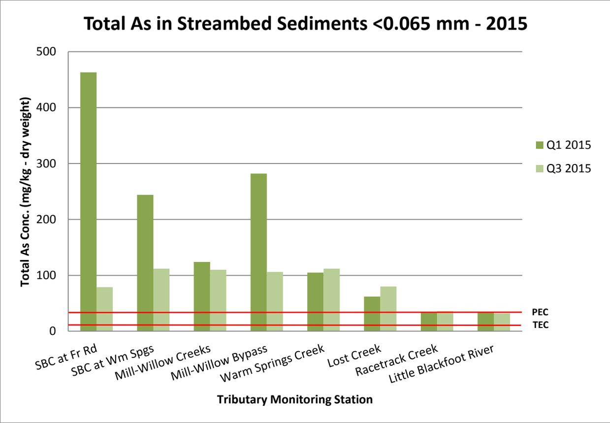
**Figure 3-3. Total arsenic (As) concentrations (dry weight) in Clark Fork River tributary sediment samples, 2015. Red lines represent the “threshold effect concentration” (TEC) and the “probable effect concentration” (PEC) [MacDonald et al., 2000].**
