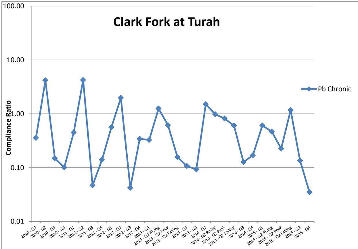
**Figure 2-66. Total recoverable lead (Pb) compliance ratios for the Clark Fork River at Turah site, 2010-2015. Compliance ratios are based on the chronic aquatic life standard [MDEQ, 2012b].**
