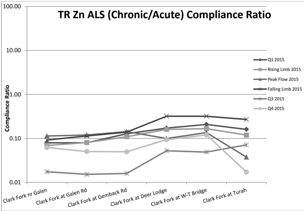
**Figure 2-75. Total recoverable zinc (TR Zn) compliance ratios for the Clark Fork River mainstem sites, 2015 Compliance ratios are based on the chronic and acute aquatic life standard (ALS) [MDEQ, 2012b].**
