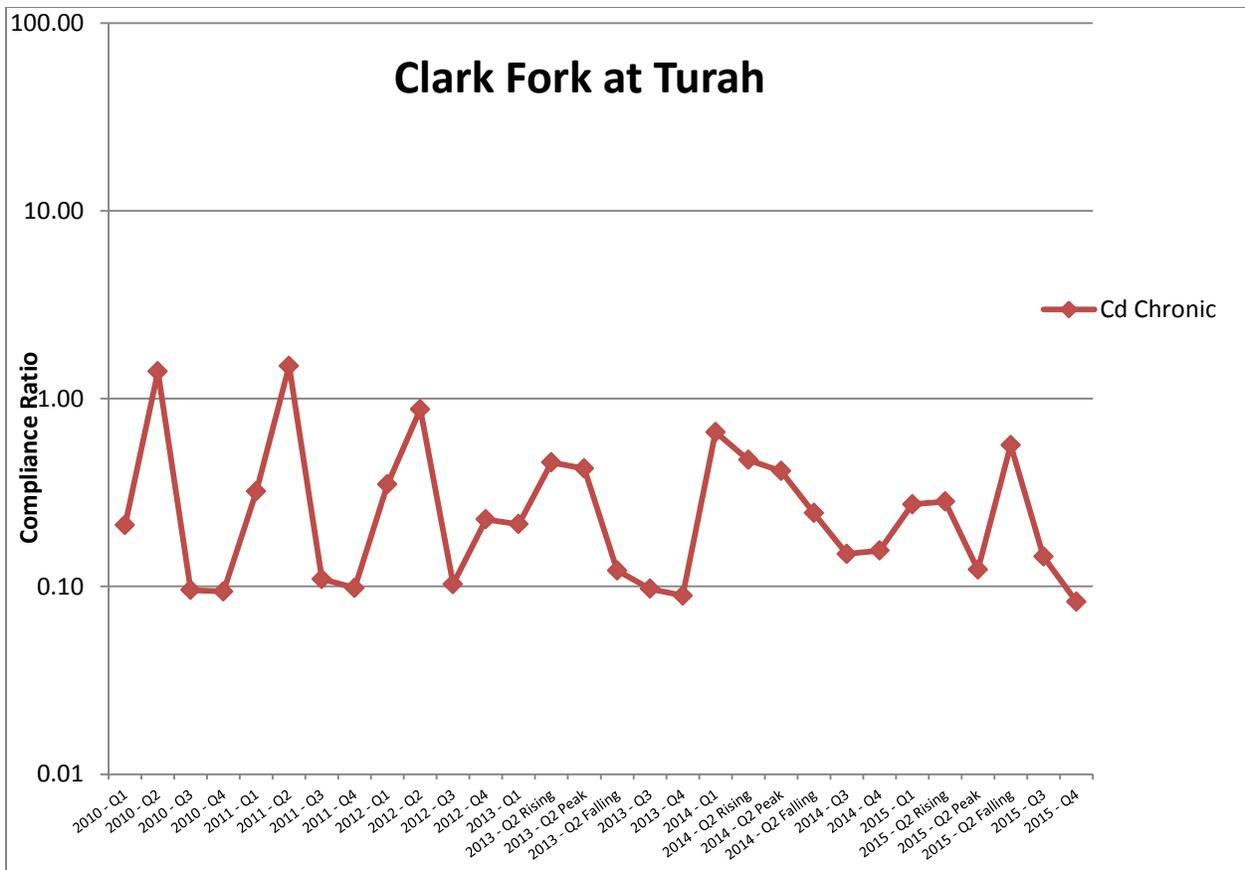
**Figure 2-48. Total recoverable cadmium (Cd) compliance ratios for the Clark Fork River at Turah site, 2010-2015. Compliance ratios are based on the chronic aquatic life standard [MDEQ, 2012b].**
