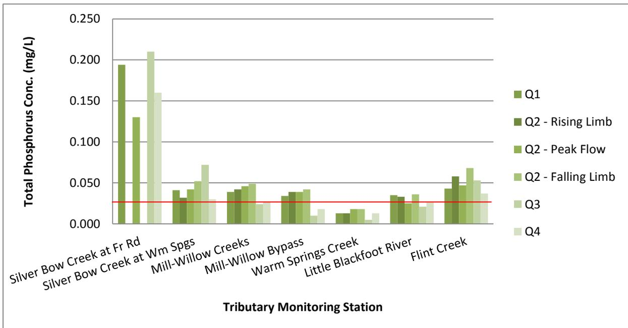
Figure 2-34. Total phosphorus concentrations (mg/L) at Clark Fork River tributary monitoring stations, 2015. Red line represents total phosphorus standard [MDEQ, 2014]. No samples were collected during the Q2-Rising Limb and Q2-Falling Limb monitoring periods at the “Silver Bow Creek at Fr Rd” site.
