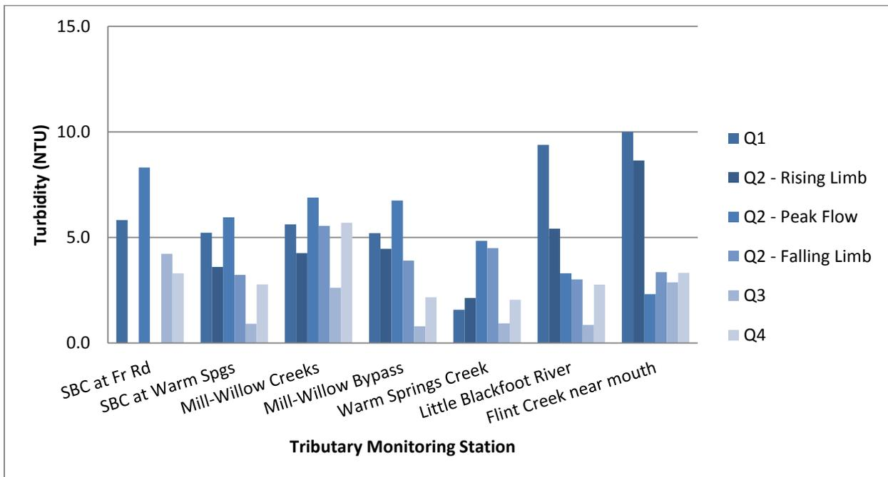
Figure 2-18. Turbidity at tributary sampling sites in the Clark Fork River Operable Unit, 2015. No samples were collected during the Q2-Rising Limb and Q2-Falling Limb monitoring periods at the “SBC at Fr Rd” site.
