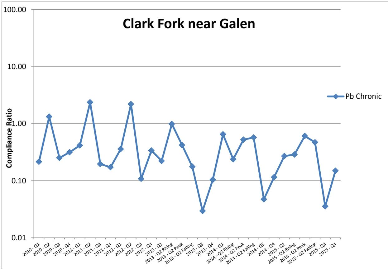
**Figure 2-64. Total recoverable lead (Pb) compliance ratios for the Clark Fork River near Galen site, 2010-2015. Compliance ratios are based on the chronic aquatic life standard [MDEQ, 2012b].**
