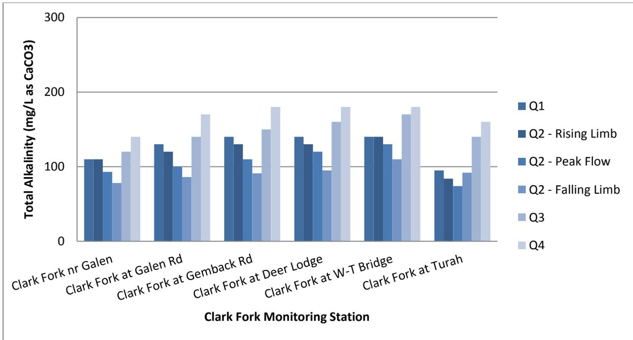
Figure 2-23. Alkalinity at mainstem sampling sites in the Clark Fork River Operable Unit, 2015.
