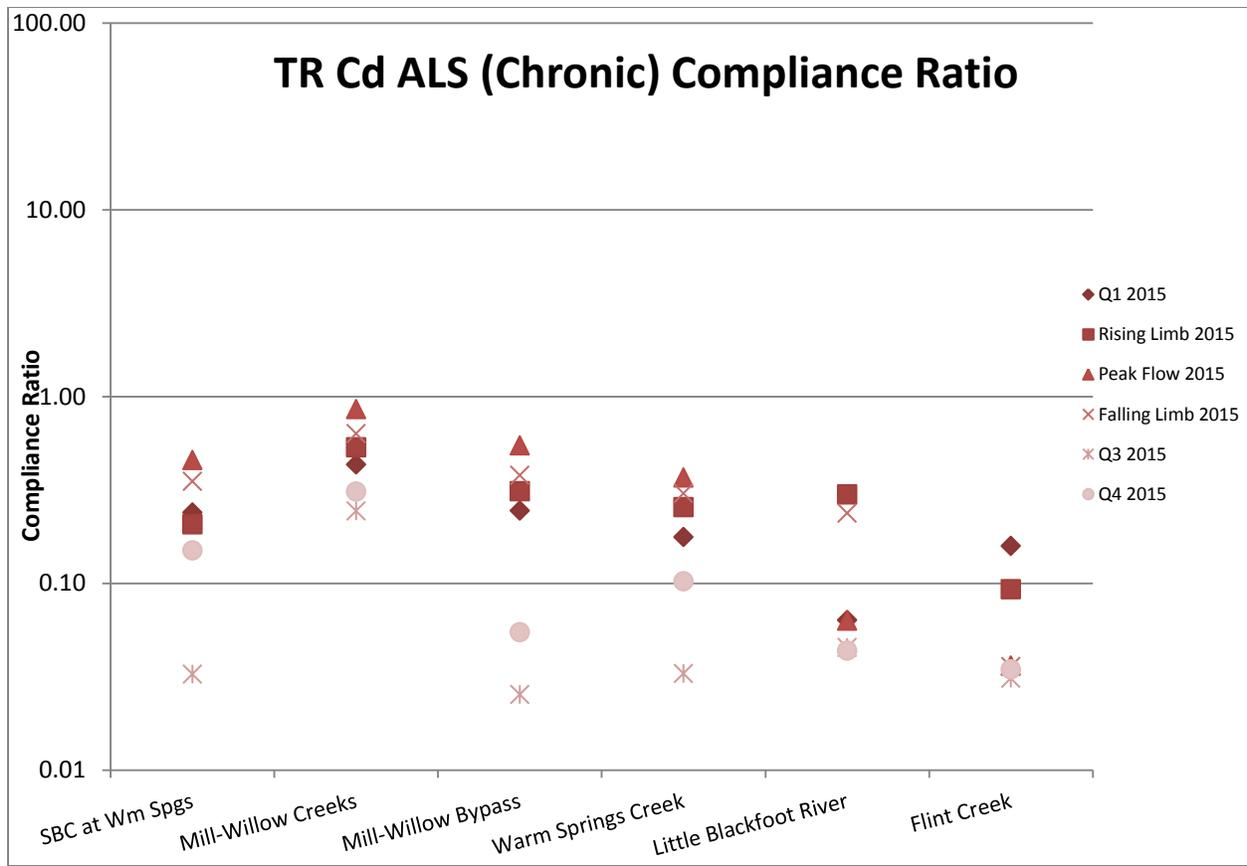
**Figure 2-52. Total recoverable cadmium (TR Cd) compliance ratios for the Clark Fork River tributary sites, 2015. Compliance ratios are based on the chronic aquatic life standard (ALS) [MDEQ, 2012b].**
