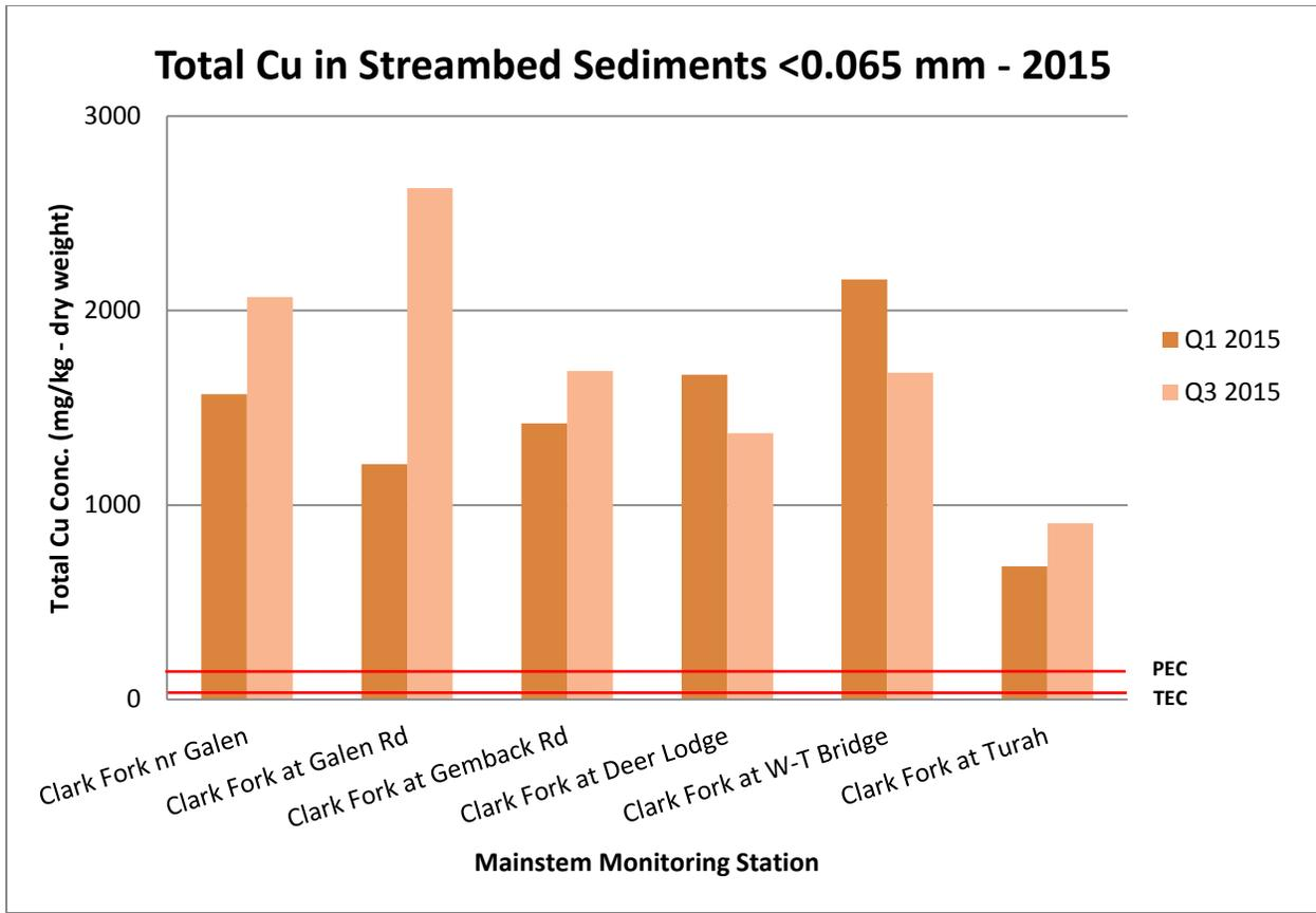
**Figure 3-6. Total copper (Cu) concentrations (dry weight) in Clark Fork River mainstem sediment samples, 2015. Red lines represent the “threshold effect concentration” (TEC) and the “probable effect concentration” (PEC) [MacDonald et al., 2000].**
