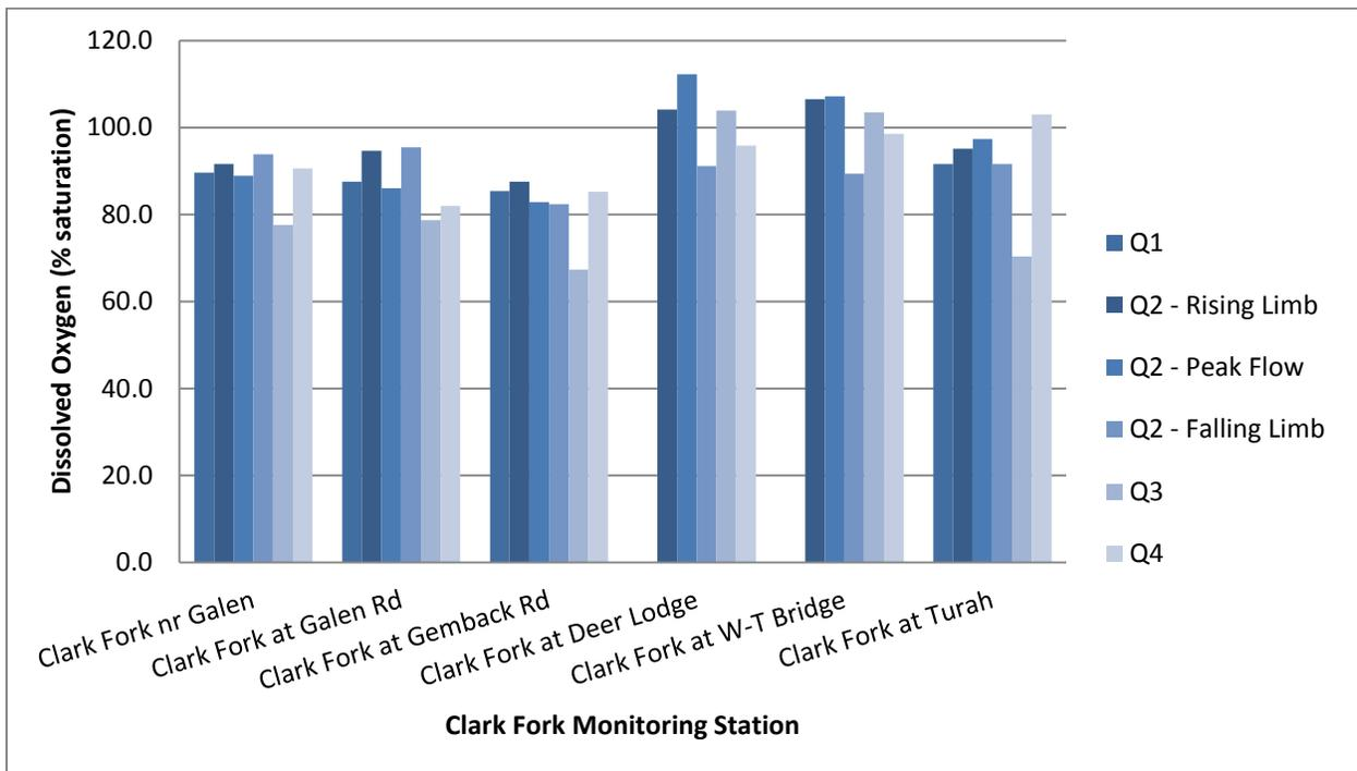
Figure 2-14. Dissolved oxygen saturation at mainstem sampling sites in the Clark Fork River Operable Unit, 2015.
