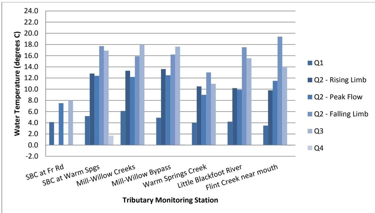
**Figure 2-8. Surface water temperatures at tributary sampling sites in the Clark Fork River Operable Unit, 2015. Temperatures during the fourth quarter (Q4) monitoring period were at or near 0 C at some sites. No samples were collected during the Q2-Rising Limb and Q2-Falling Limb monitoring periods at the “SBC at Fr Rd” site.**
