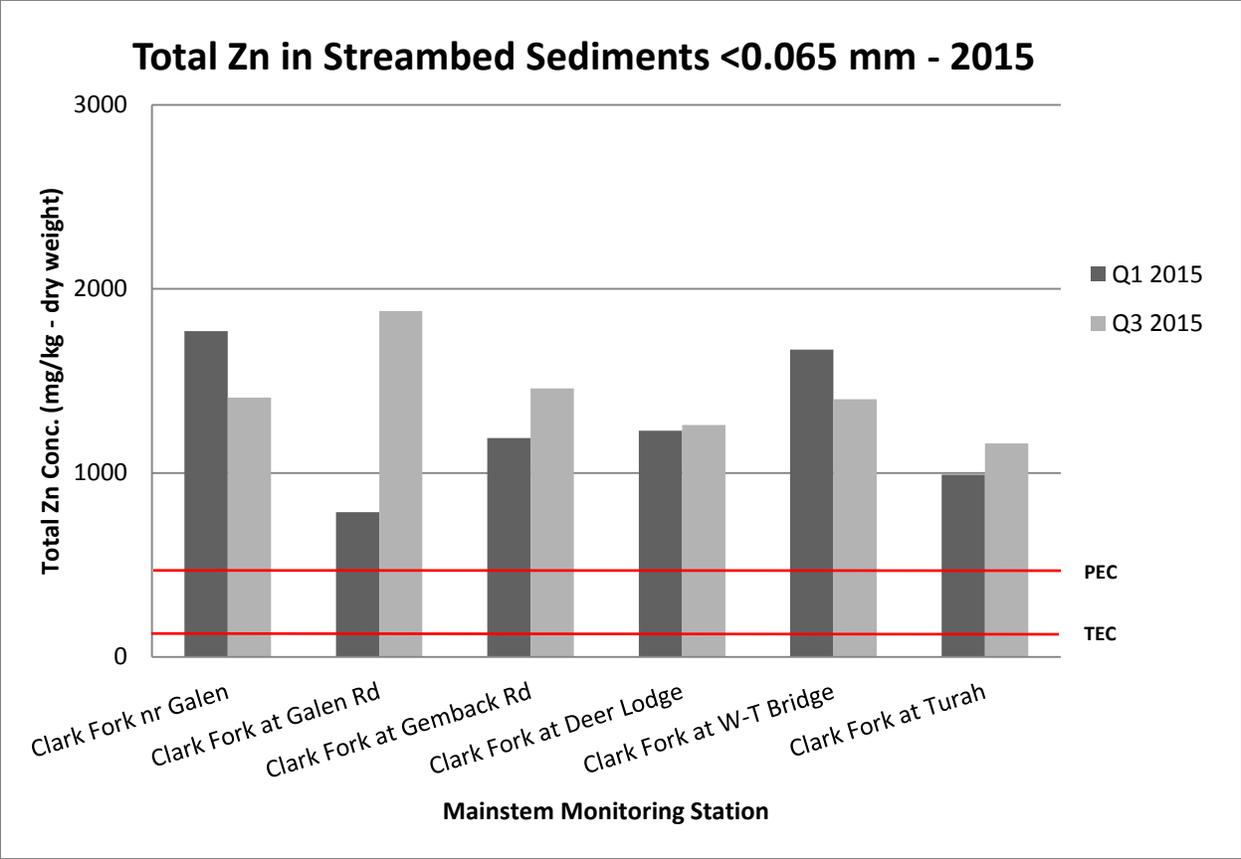
Figure 3-10. Total zinc (Zn) concentrations (dry weight) in Clark Fork River mainstem sediment samples, 2015. Red lines represent the “threshold effect concentration” (TEC) and the “probable effect concentration” (PEC) [MacDonald et al., 2000].
