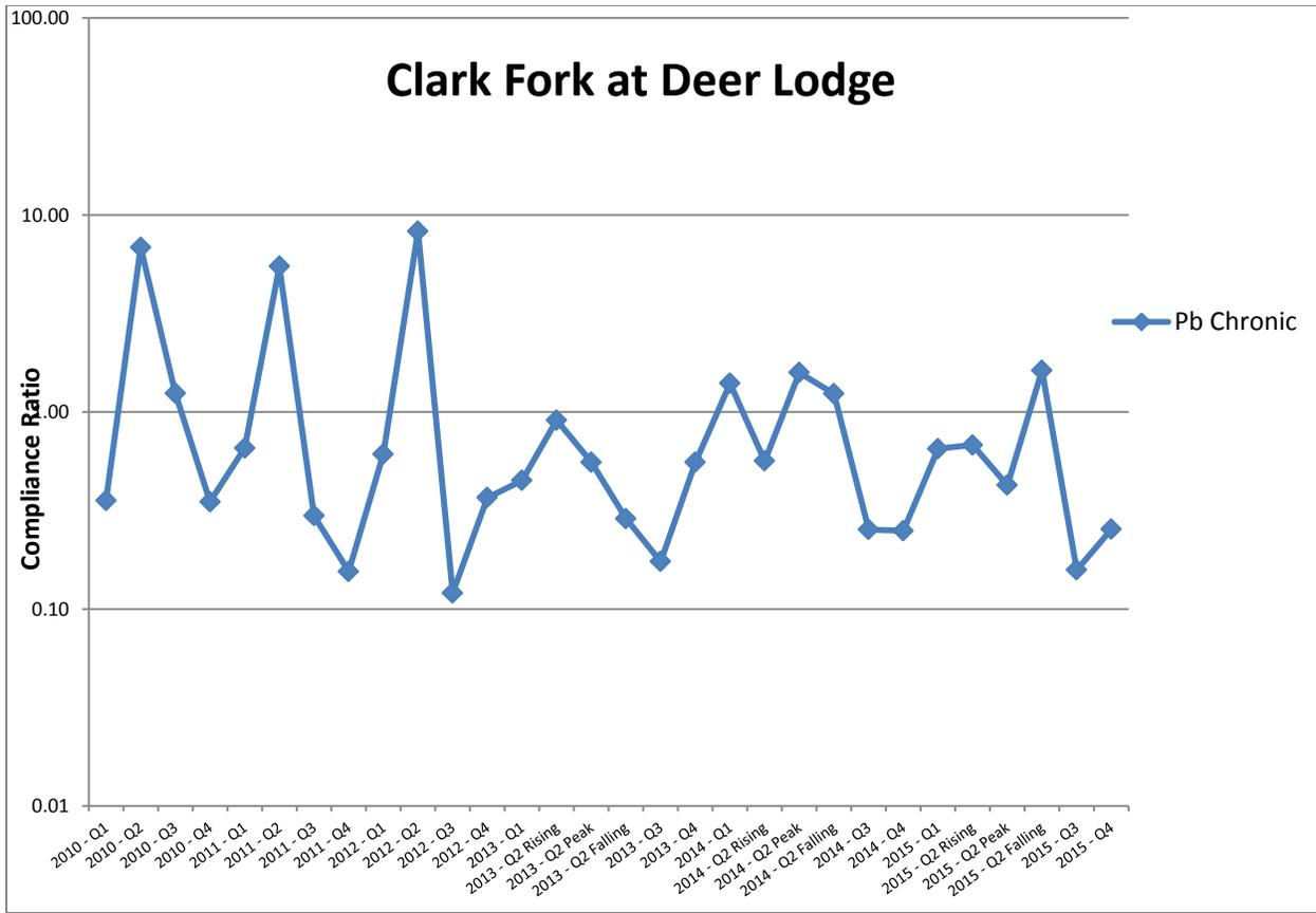
**Figure 2-65. Total recoverable lead (Pb) compliance ratios for the Clark Fork River at Deer Lodge site, 2010-2015. Compliance ratios are based on the chronic aquatic life standard [MDEQ, 2012b].**
