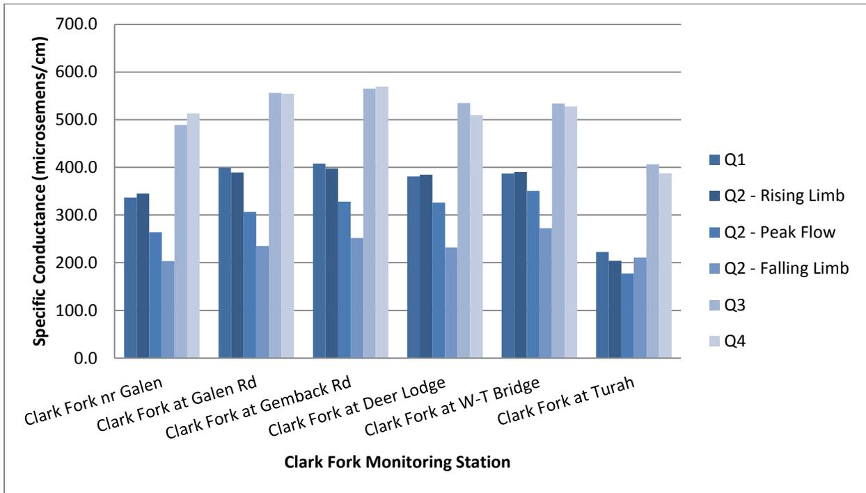
**Figure 2-11. Conductivity at mainstem sampling sites in the Clark Fork River Operable Unit, 2015.**
