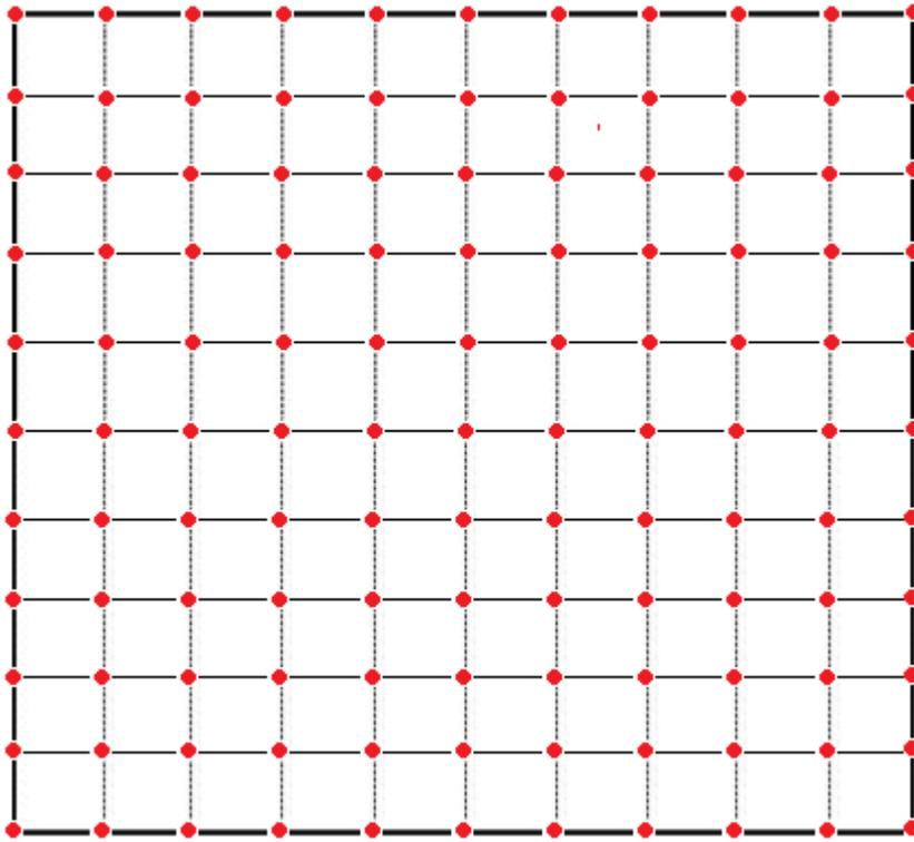
**Figure 4-4. Schematic sampling grid for floodplain canopy cover within floodplain plots. Sampling grid lines were evenly spaced (11 per side including the plot boundaries) along each plot side. Samples were collected at each gridline intersection (red dots) for a total of 121 cover measurements per floodplain plot.**
