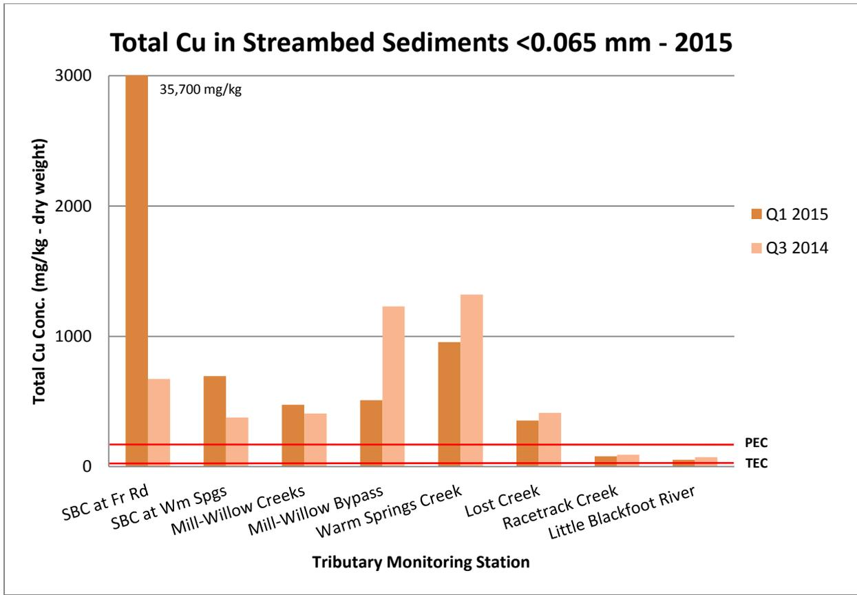
Figure 3-7. Total copper (Cu) concentrations (dry weight) in Clark Fork River tributary sediment samples, 2015. Red lines represent the “threshold effect concentration” (TEC) and the “probable effect concentration” (PEC) [MacDonald et al., 2000].
