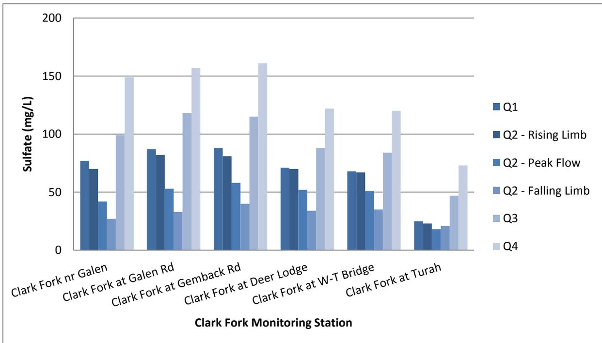
**Figure 2-27. Sulfate concentrations at mainstem sampling sites in the Clark Fork River Operable Unit, 2015.**
