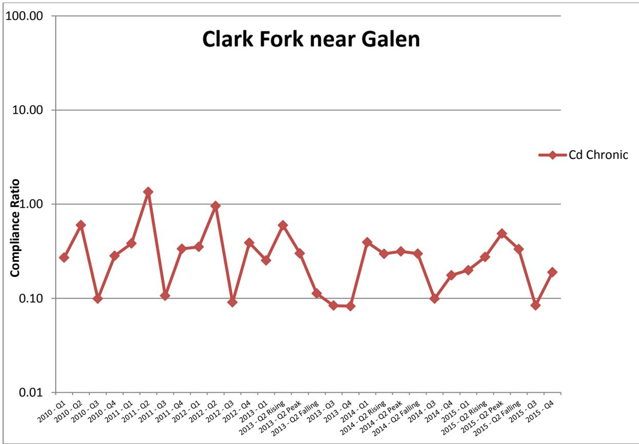
**Figure 2-46. Total recoverable cadmium (Cd) compliance ratios for the Clark Fork River near Galen site, 2010-2015. Compliance ratios are based on the chronic aquatic life standard [MDEQ, 2012b].**
