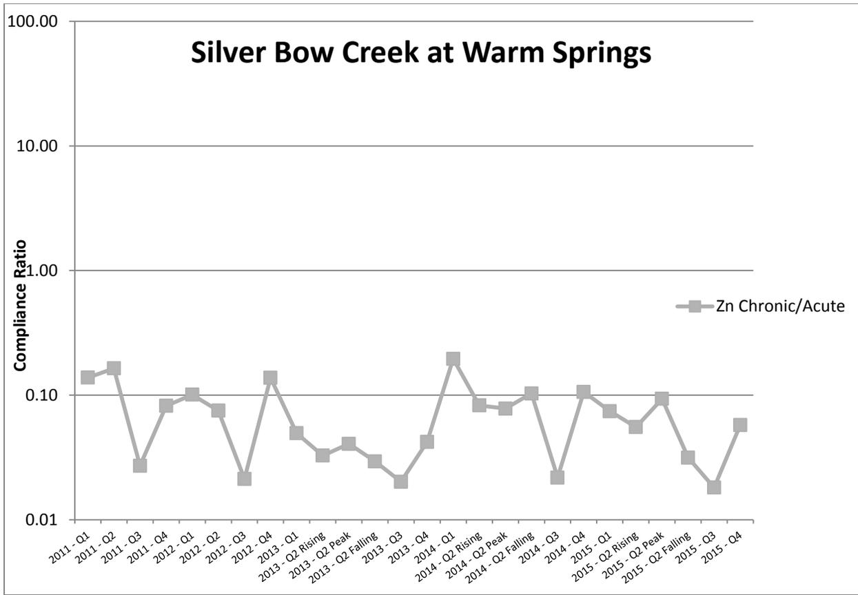
**Figure 2-77. Total recoverable zinc (Zn) compliance ratios for the Silver Bow Creek at Warm Springs site, 2011-2015. Compliance ratios are based on the aquatic life standard [MDEQ, 2012b].**
