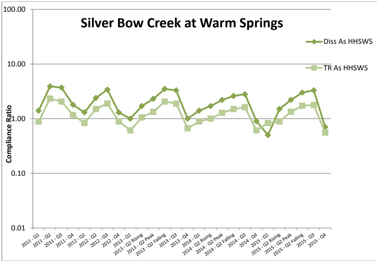
**Figure 2-42. Total recoverable (TR) and dissolved (Diss) arsenic (As) compliance ratios for the Silver Bow Creek at Warm Springs site, 2011-2015. Compliance ratios are based on the Clark Fork River Operable Unit Record of Decision performance goals for dissolved (Diss As HHSWS) and total recoverable (TR As HHSWS) arsenic concentrations [USEPA, 2004].**
