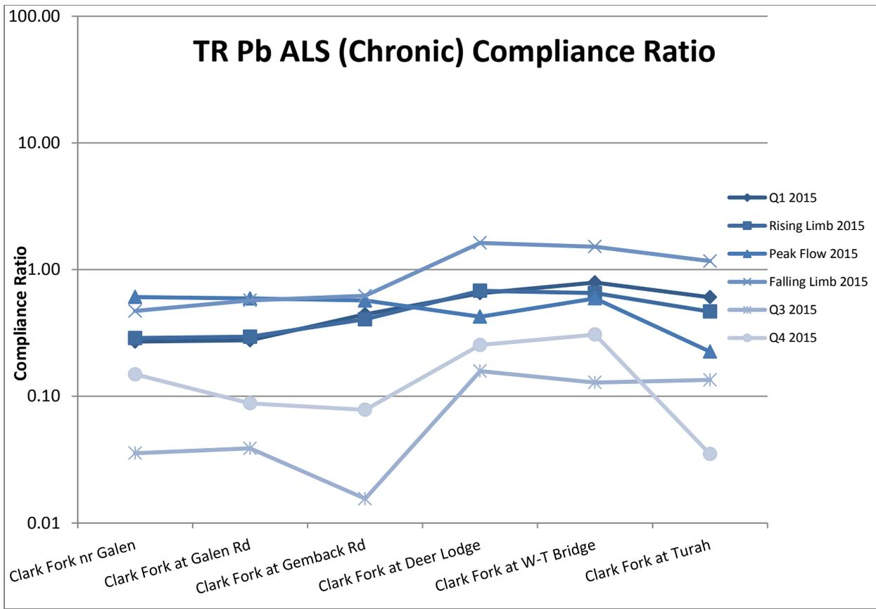
**Figure 2-67. Total recoverable lead (TR Pb) compliance ratios for the Clark Fork River mainstem sites, 2015. Compliance ratios are based on the chronic aquatic life standard (ALS) [MDEQ, 2012b].**
