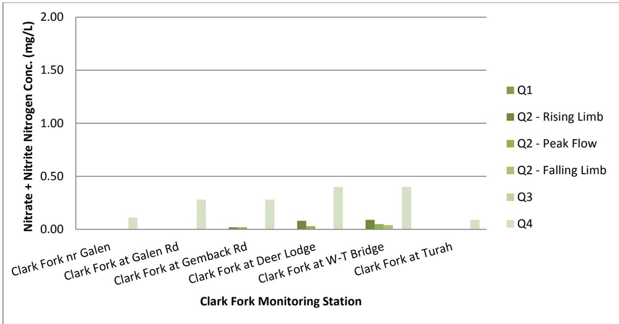
Figure 2-31. Nitrate plus nitrite nitrogen concentrations (mg/L) at Clark Fork River mainstem monitoring stations, 2015. Sites or sample periods with no bars indicate concentrations below the analytical reporting limit.
