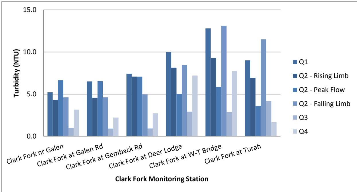
Figure 2-17. Turbidity at mainstem sampling sites in the Clark Fork River Operable Unit, 2015.
