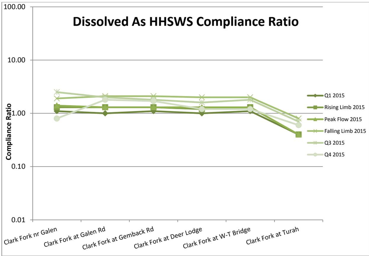
**Figure 2-39. Dissolved arsenic (Diss As) compliance ratios for the Clark Fork River mainstem sites, 2015. Compliance ratio is based on Clark Fork River Operable Unit Record of Decision performance goal for dissolved arsenic (Dissolved As HHSWS) concentration [USEPA, 2004].**
