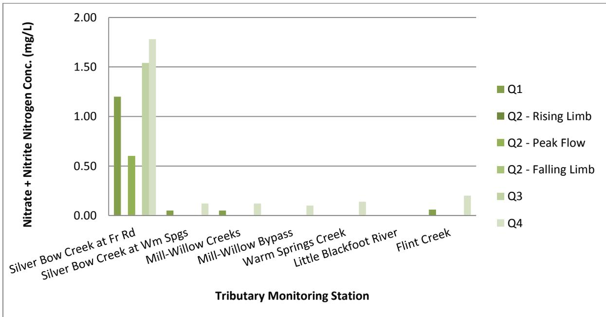
Figure 2-32. Nitrate plus nitrite nitrogen concentrations (mg/L) at Clark Fork River tributary monitoring stations, 2015. No samples were collected during the Q2-Rising Limb and Q2-Falling Limb monitoring periods at the “Silver Bow Creek at Fr Rd” site. Other sites or sample periods with no bars indicate concentrations below the analytical reporting limit.
