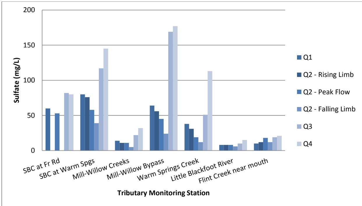
**Figure 2-28. Sulfate concentrations at tributary sampling sites in the Clark Fork River Operable Unit, 2015. No samples were collected during the Q2-Rising Limb and Q2-Falling Limb monitoring periods at the “SBC at Fr Rd” site.**
