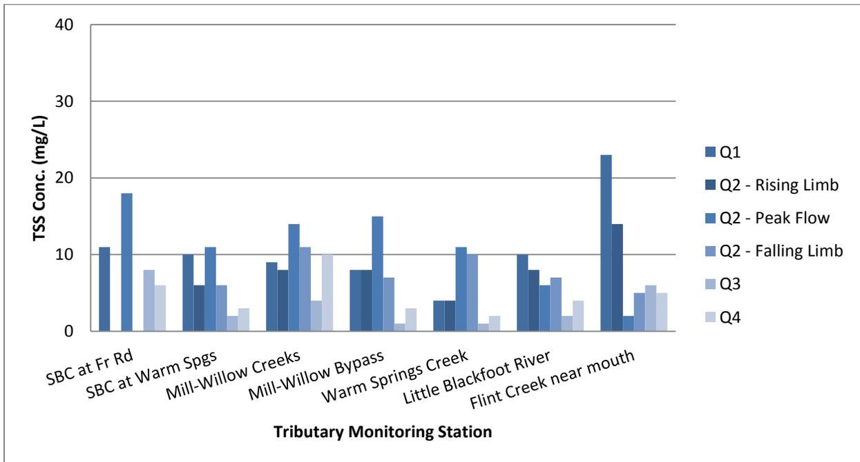
**Figure 2-20. Total suspended sediment concentrations at tributary sampling sites in the Clark Fork River Operable Unit, 2015. No samples were collected during the Q2-Rising Limb and Q2-Falling Limb monitoring periods at the “SBC at Fr Rd” site.**
