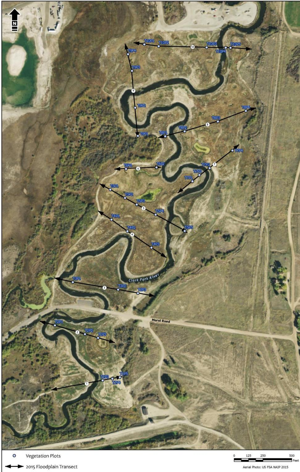
**Figure 4-2. Floodplain cover monitoring transects in Phase 1 of the Clark Fork River Operable Unit, 2015. Two sub-plots (9 ft<sup>2</sup>) were established along a 3'x15' belt transect perpendicular to plot points along each transect.**
