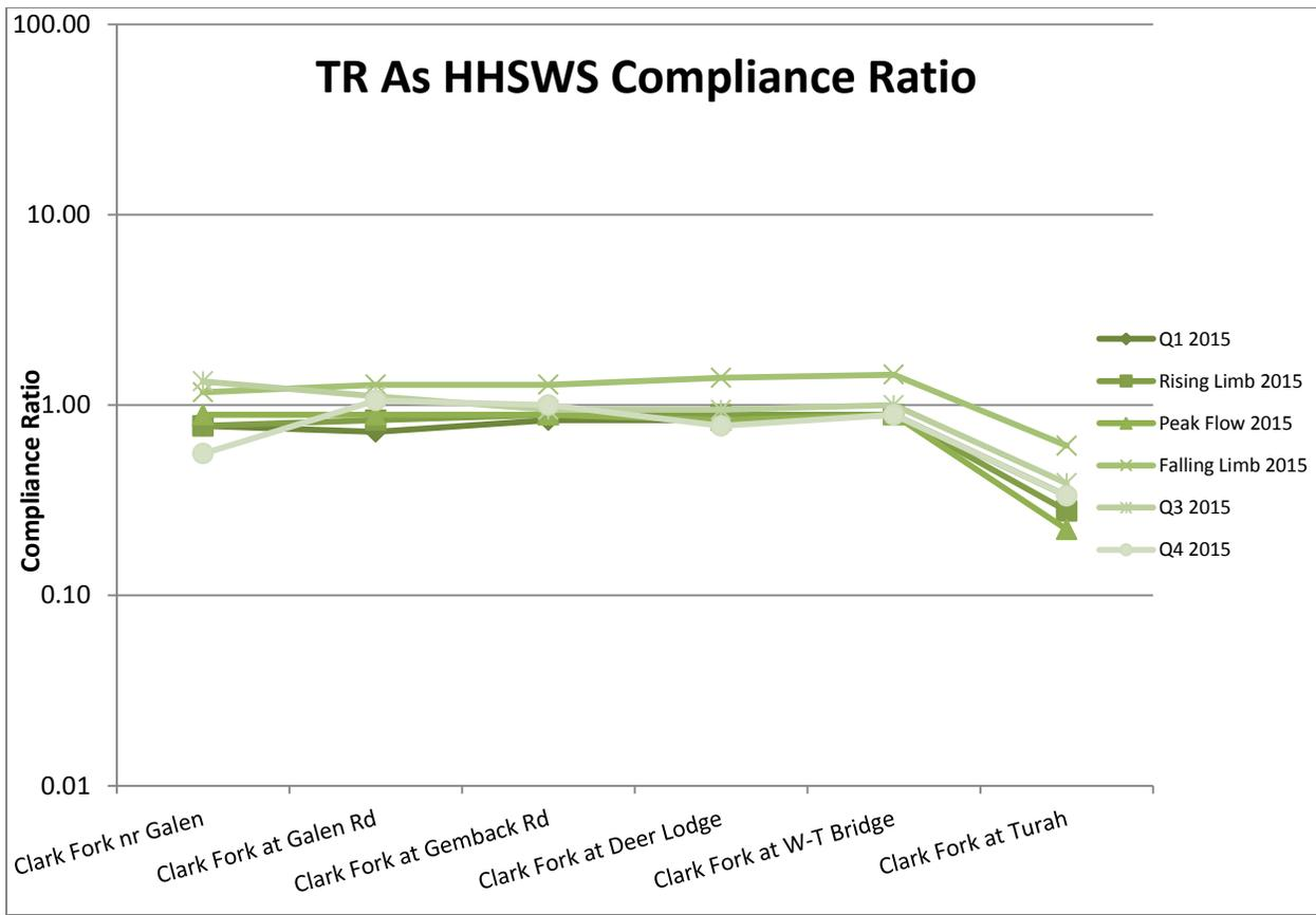
**Figure 2-40. Total recoverable arsenic (TR As) compliance ratios for the Clark Fork River mainstem sites, 2015. Compliance ratio is based on Clark Fork River Operable Unit Record of Decision performance goal for total recoverable arsenic (TR As HHSWS) concentration [USEPA, 2004].**
