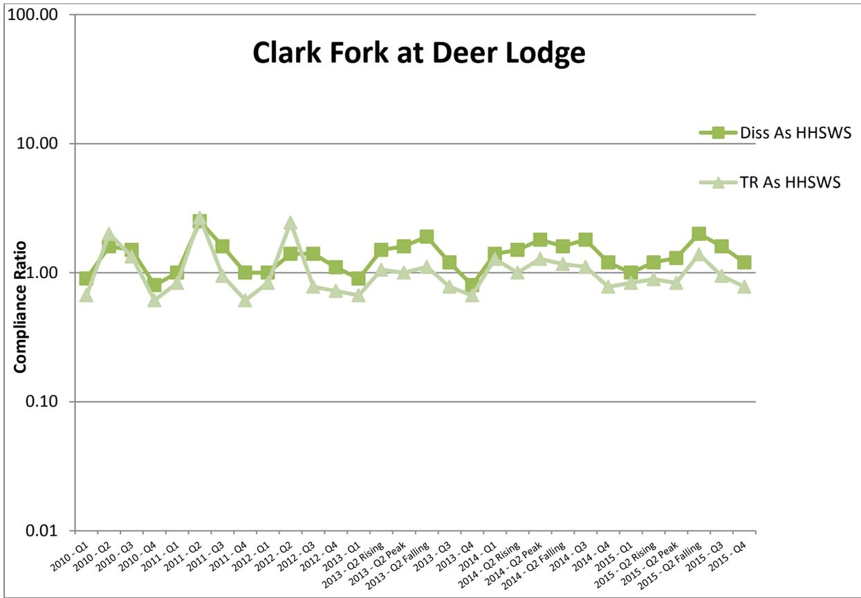
**Figure 2-37. Total recoverable (TR) and dissolved (Diss) arsenic (As) compliance ratios for the Clark Fork River at Deer Lodge site, 2010-2015. Compliance ratios are based on the Clark Fork River Operable Unit Record of Decision performance goals for dissolved (Diss As HHSWS) and total recoverable (TR As HHSWS) arsenic concentrations [USEPA, 2004].**
