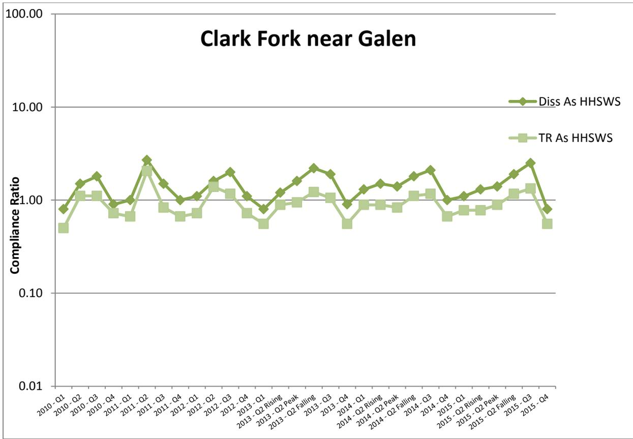
**Figure 2-36. Total recoverable (TR) and dissolved (Diss) arsenic (As) compliance ratios for the Clark Fork River near Galen site, 2010-2015. Compliance ratios are based on the Clark Fork River Operable Unit Record of Decision performance goals for dissolved (Diss As HHSWS) and total recoverable (TR As HHSWS) arsenic concentrations [USEPA, 2004].**
