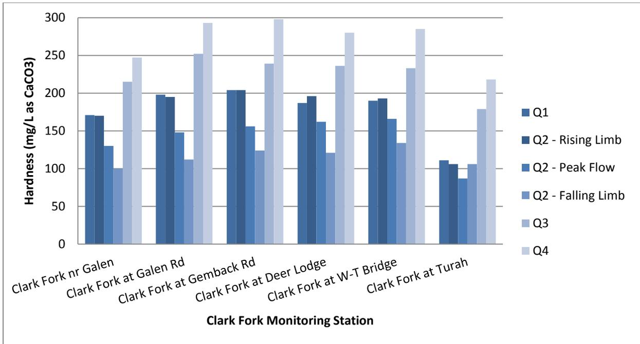
Figure 2-21. Water hardness at mainstem sampling sites in the Clark Fork River Operable Unit, 2015.
