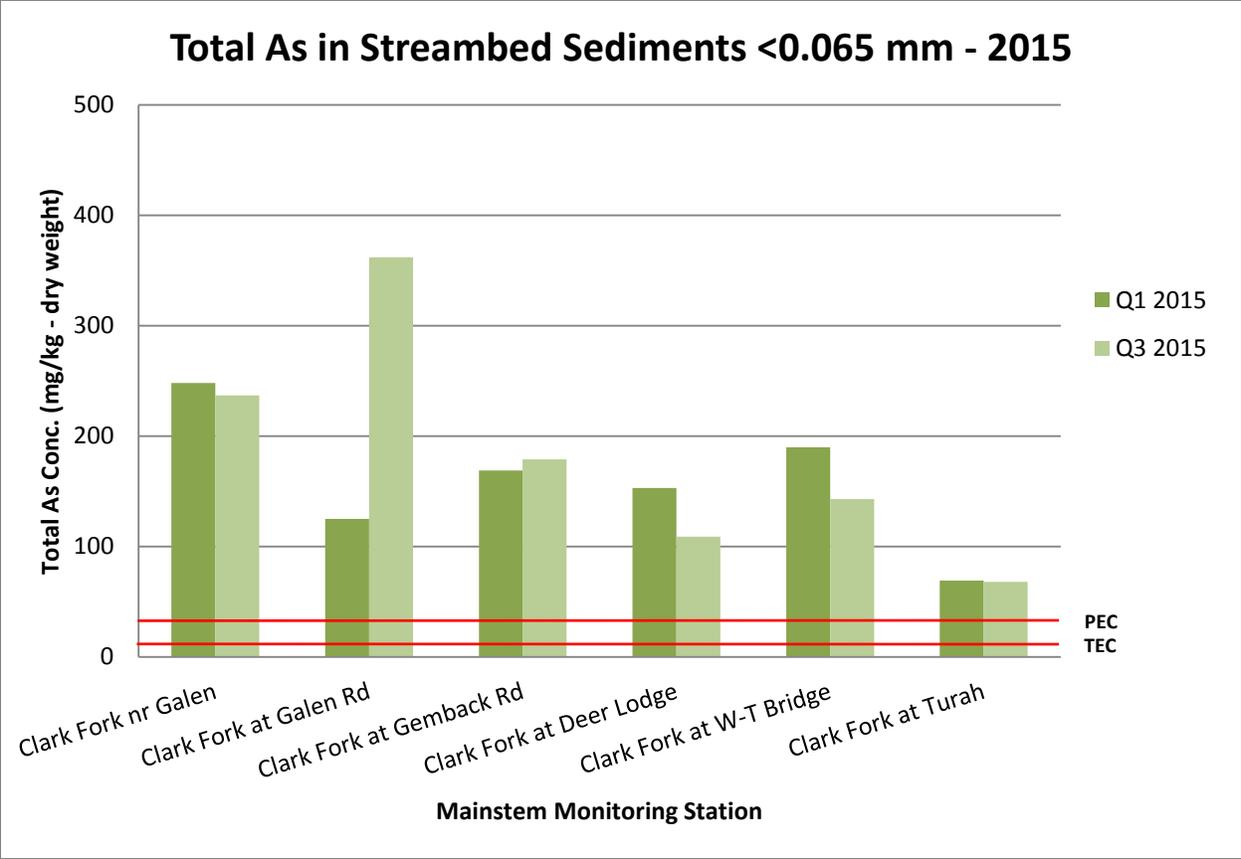
**Figure 3-2. Total arsenic (As) concentrations (dry weight) in Clark Fork River mainstem sediment samples, 2015. Red lines represent the “threshold effect concentration” (TEC) and the “probable effect concentration” (PEC) [MacDonald et al., 2000].**
