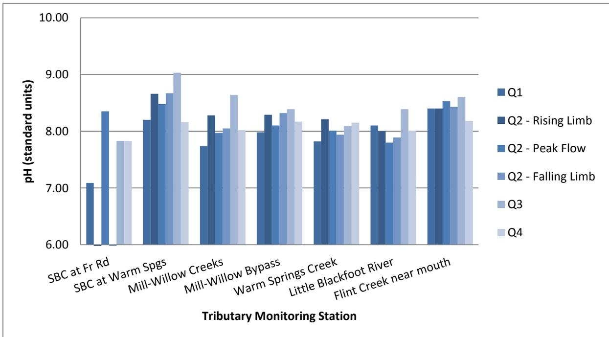
Figure 2-10. Surface water pH at tributary sampling sites in the Clark Fork River Operable Unit, 2015. No samples were collected during the Q2-Rising Limb and Q2-Falling Limb monitoring periods at the “SBC at Fr Rd” site.
