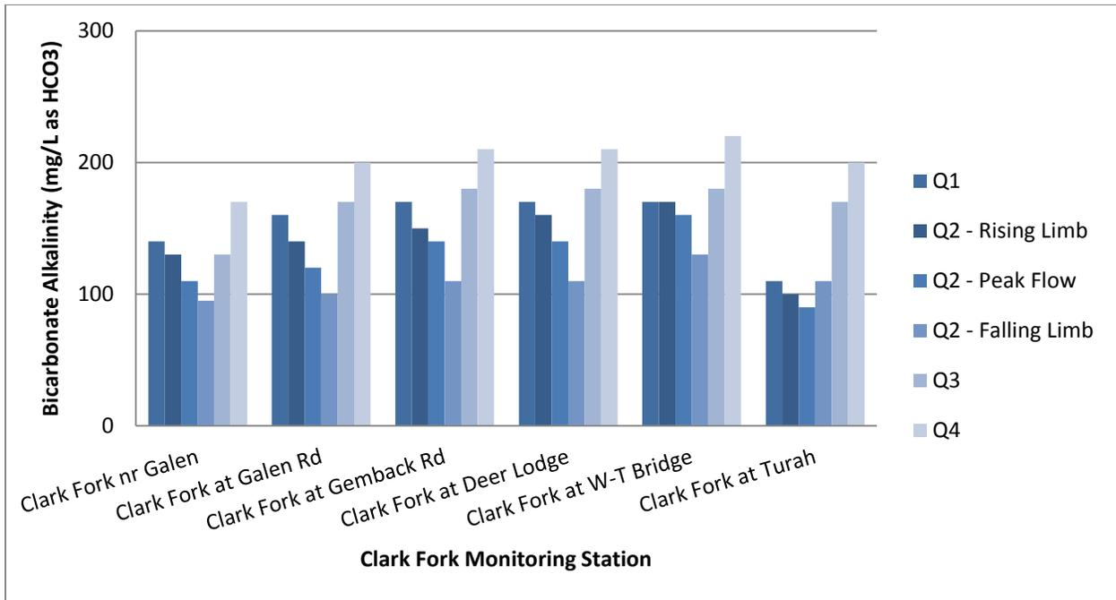
Figure 2-25. Bicarbonate alkalinity at mainstem sampling sites in the Clark Fork River Operable Unit, 2015.
