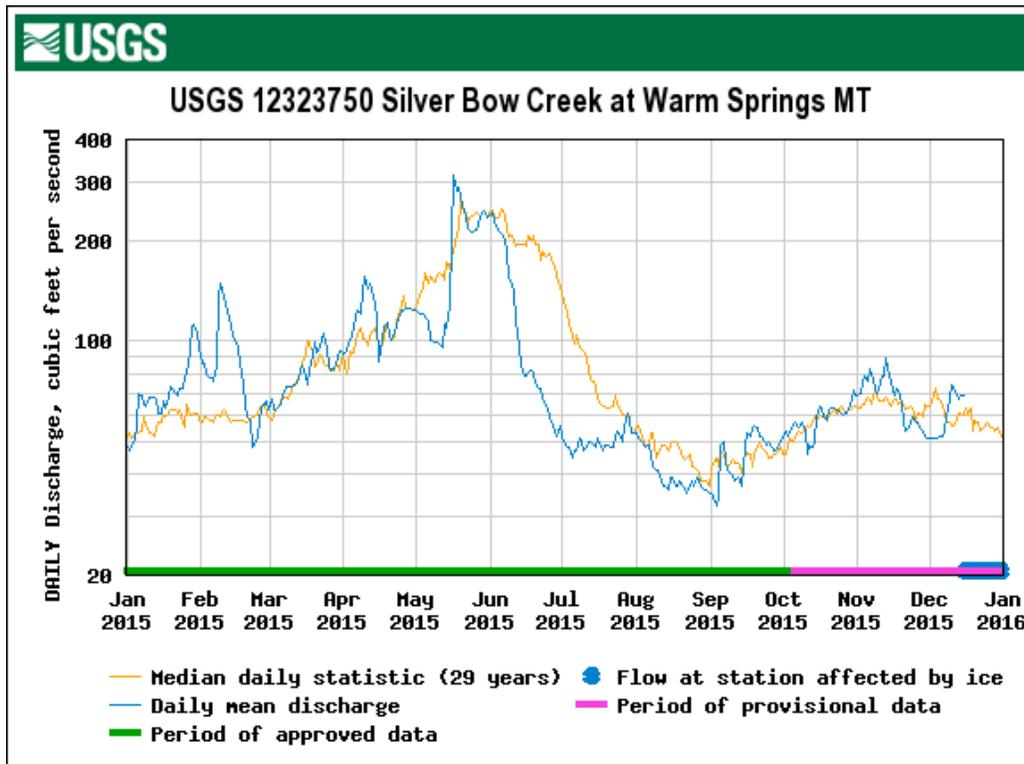
Figure 2-2. Hydrograph for Silver Bow Creek at Warm Springs, 2015.
