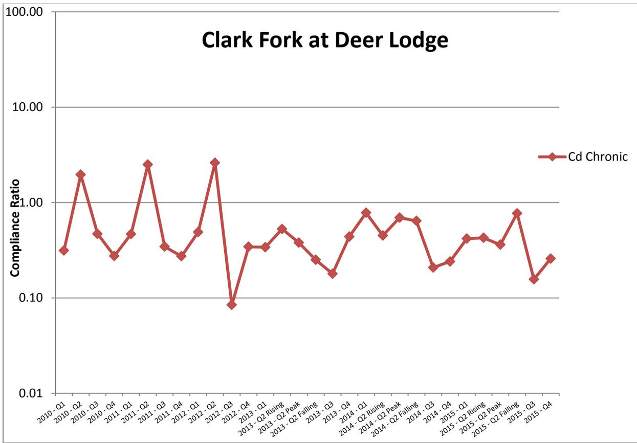
**Figure 2-47. Total recoverable cadmium (Cd) compliance ratios for the Clark Fork River at Deer Lodge site, 2010-2015. Compliance ratios are based on the chronic aquatic life standard [MDEQ, 2012b].**
