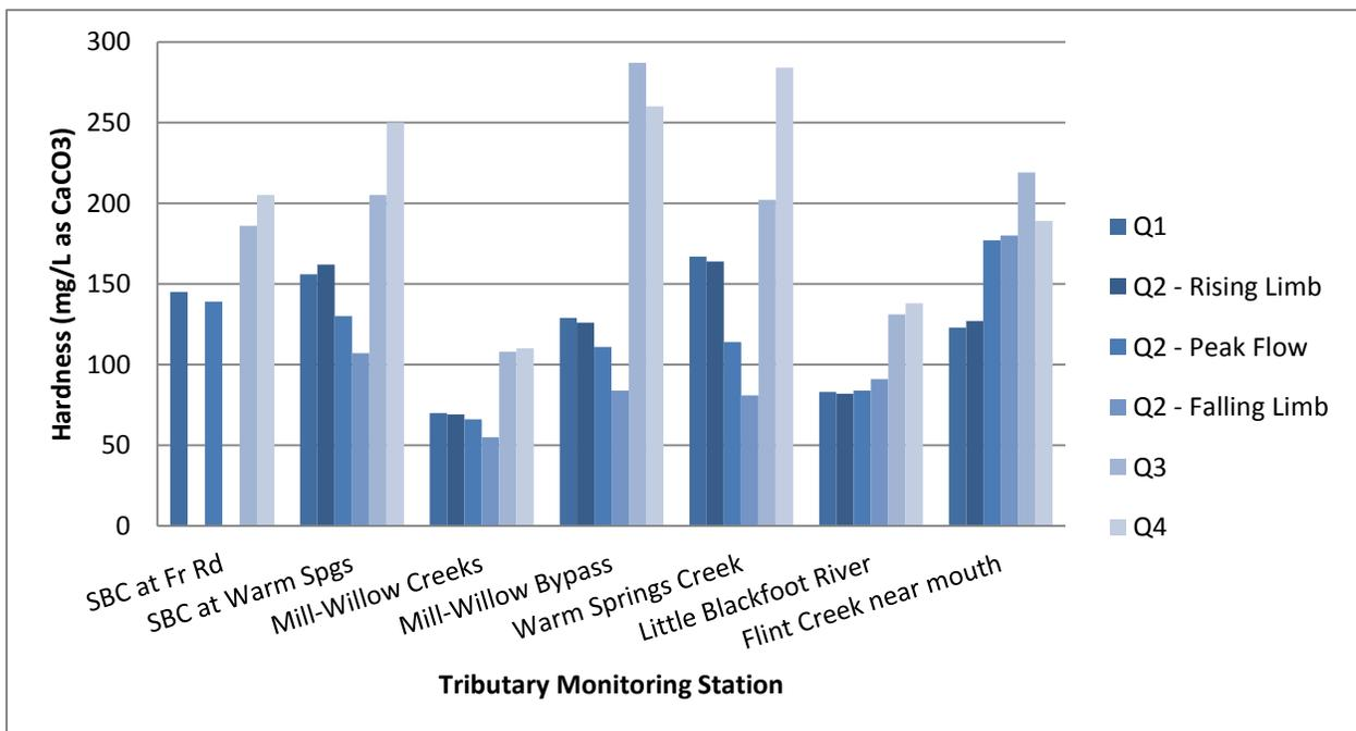
Figure 2-22. Water hardness at tributary sampling sites in the Clark Fork River Operable Unit, 2015. No samples were collected during the Q2-Rising Limb and Q2-Falling Limb monitoring periods at the “SBC at Fr Rd” site.
