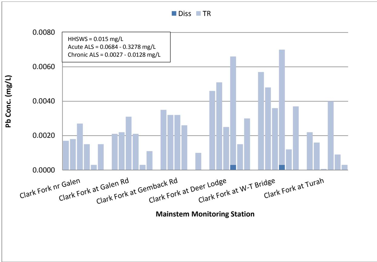
**Figure 2-63. Total recoverable (total recoverable) and dissolved (Diss) lead (Pb) concentrations at mainstem sampling sites in the Clark Fork River Operable Unit, 2015. No bars indicate concentrations below the analytical reporting limit. Applicable water quality standards are the aquatic life standards (ALS) and the human health surface water standard (HHSWS) [MDEQ, 2012b].**
