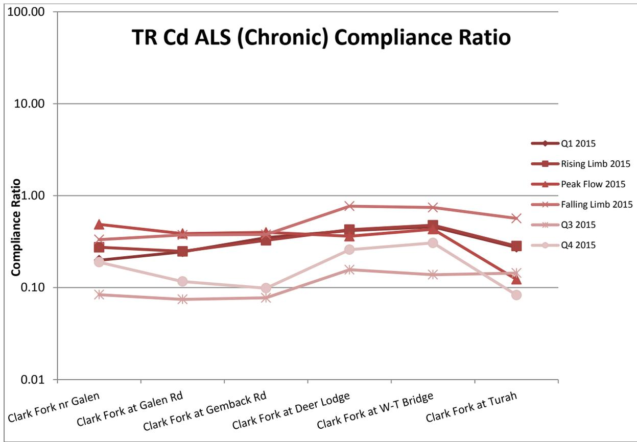
**Figure 2-49. Total recoverable cadmium (TR Cd) compliance ratios for the Clark Fork River mainstem sites, 2015. Compliance ratios are based on the chronic aquatic life standard (ALS) [MDEQ, 2012b].**
