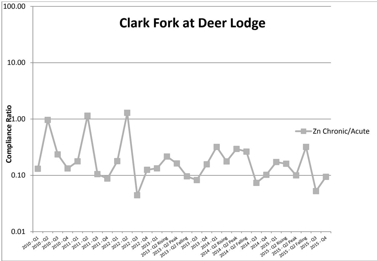
**Figure 2-73. Total recoverable zinc (Zn) compliance ratios for the Clark Fork River at Deer Lodge site, 2010-2015. Compliance ratios are based on the aquatic life standard [MDEQ, 2012b].**
