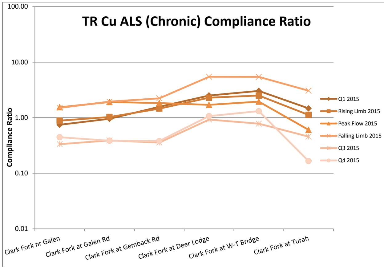
**Figure 2-58. Total recoverable copper (TR Cu) compliance ratios for the Clark Fork River mainstem sites, 2015. Compliance ratios are based on the chronic aquatic life standard (ALS) [MDEQ, 2012b].**
