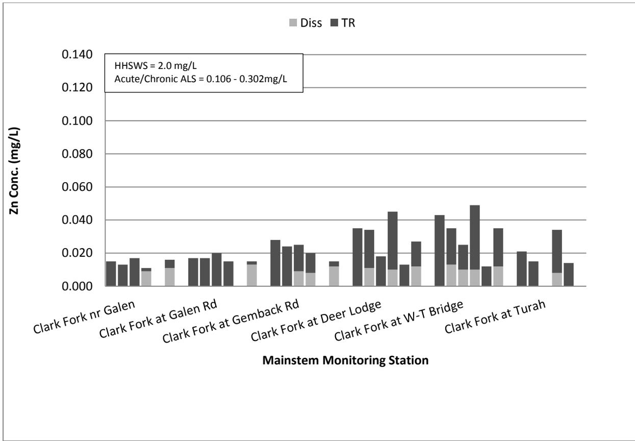
**Figure 2-71. Total recoverable (TR) and dissolved (Diss) zinc (Zn) concentrations at mainstem sampling sites in the Clark Fork River Operable Unit, 2015. No bars indicate concentrations below the analytical reporting limit. Applicable water quality standards are the aquatic life standard (ALS) and the human health surface water standard (HHSWS) [MDEQ, 2012b].**
