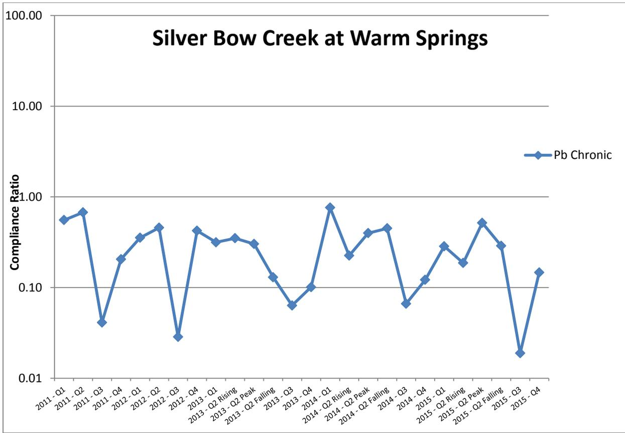
**Figure 2-69. Total recoverable lead (Pb) compliance ratios for the Silver Bow Creek at Warm Springs site, 2011-2015. Compliance ratios are based on the chronic aquatic life standard [MDEQ, 2012b].**
