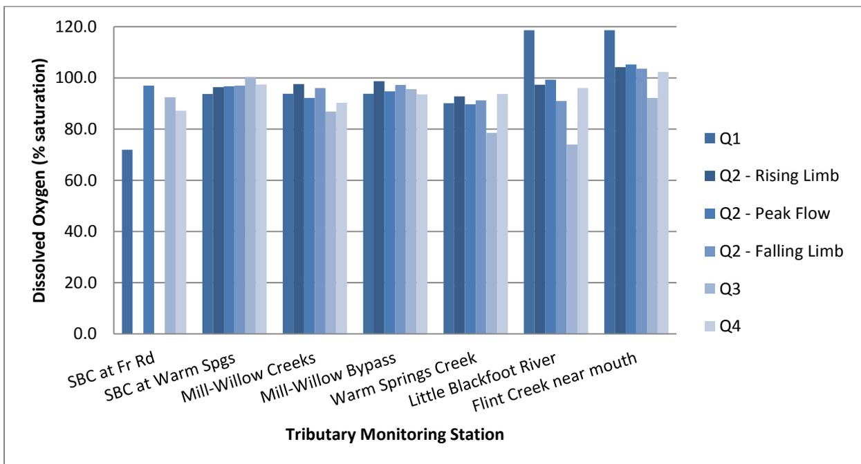
Figure 2-16. Dissolved oxygen saturation at tributary sampling sites in the Clark Fork River Operable Unit, 2015. No samples were collected during the Q2-Rising Limb and Q2-Falling Limb monitoring periods at the “SBC at Fr Rd” site.
