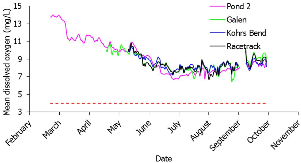
Figure 7-15. Mean daily dissolved oxygen concentrations at 2015 caged fish sites. The red dashed horizontal line denotes the freshwater ALS one day minimum.
