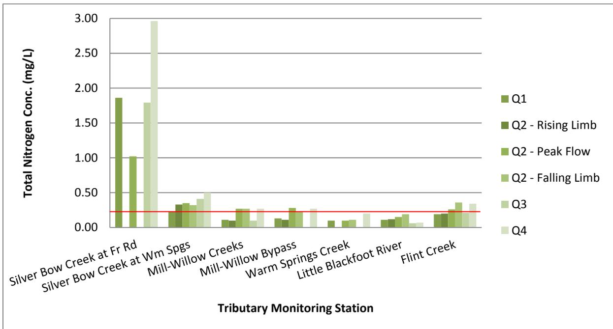
Figure 2-30. Total nitrogen concentrations (mg/L) at Clark Fork River tributary monitoring stations, 2015. Red line represents total nitrogen standard [MDEQ, 2014]. No samples were collected during the Q2-Rising Limb and Q2-Falling Limb monitoring periods at the “Silver Bow Creek at Fr Rd” site. Other sites or sample periods with no bars indicate concentrations below the analytical reporting limit.
