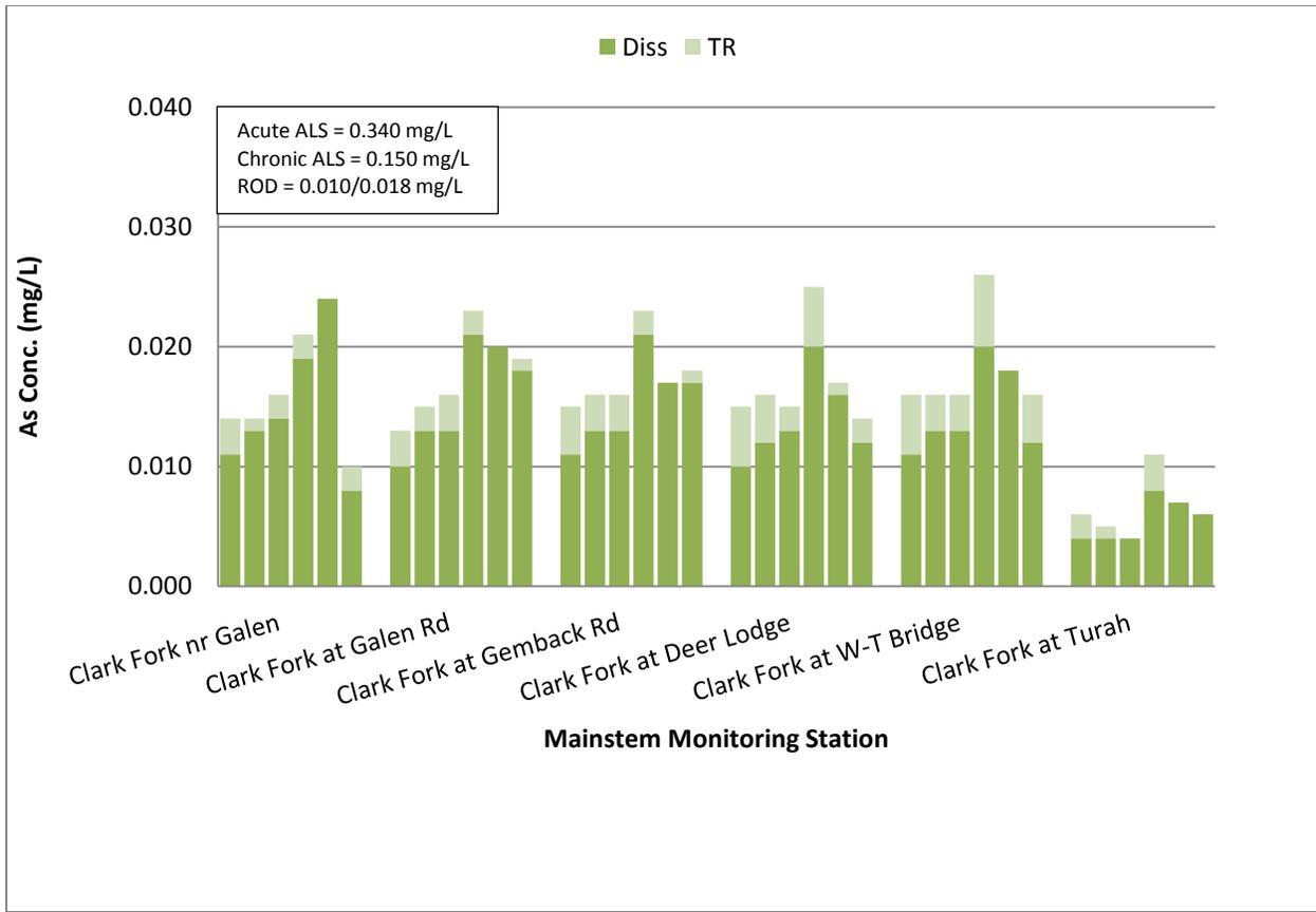
**Figure 2-35. Total recoverable (TR) and dissolved (Diss) arsenic (As) concentrations at mainstem sampling sites in the Clark Fork River Operable Unit (CFROU), 2015. Applicable water quality standards are the acute and chronic aquatic life standards (ALS) [MDEQ, 2012b] and the arsenic performance goals from the CFROU Record of Decision (ROD) [USEPA, 2004]. The ROD performance goals are 0.010 mg/L for dissolved and 0.018 mg/L for total recoverable arsenic [USEPA, 2004].**
