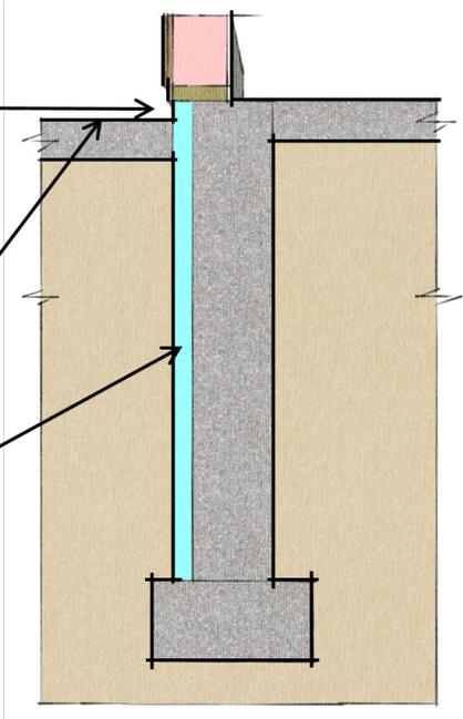
**Heated Slab-On-Grade: R-5 Under Full Slab with R-10 Edge**
