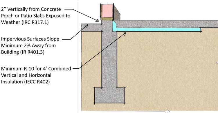
**Slab-On-Grade: Exterior Vertical Insulation at Patio or Porch Slab**
