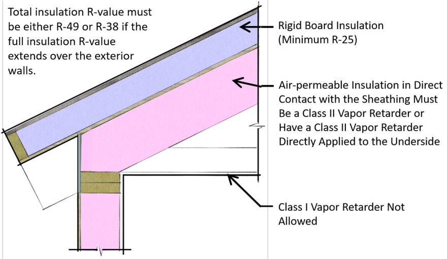
**Unvented Attic: Air-impermeable Insulation Beneath Sheathing and Air-permeable Below (IRC R806.5)**
