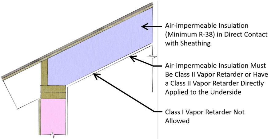
**Unvented Attic: Air-impermeable Insulation Above Sheathing and Air-permeable Below Sheathing (IRC R806.5)**
