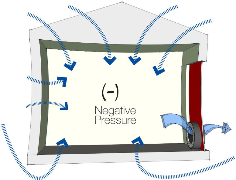
While the blower-door testing procedure is not complex, it requires care to properly set up the house and configure the digital manometer. The blower-door test procedure includes closing all exterior doors and windows and disabling all combustion appliances and exhaust fans.
