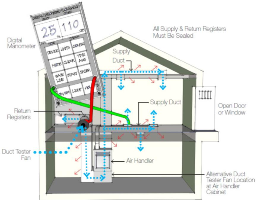
The Total Duct Leakage Test may be performed after the system has been installed or during rough-in, with or without the air handler. The leakage limits are based on the conditioned floor area. The leakage limits are:
