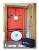
air flow and determine the air leakage rate of the house. Very efficient tight houses may have leakage rates of only 0.6 to 2.5 ACH 50.
