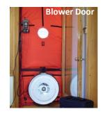
blower door is a large fan assembly, temporarily placed in an exterior doorway, which draws air flow and determine the air leakage rate of the house. Very efficient tight houses may have leakage rates of only 0.6 to 2.5 ACH 50.
