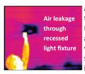
An infrared (IR) camera shows the temperature of the house's surfaces. Improperly insulated areas will appear colder than expected in winter and warmer than expected in summer. Consider having an IR investigation to confirm the house
