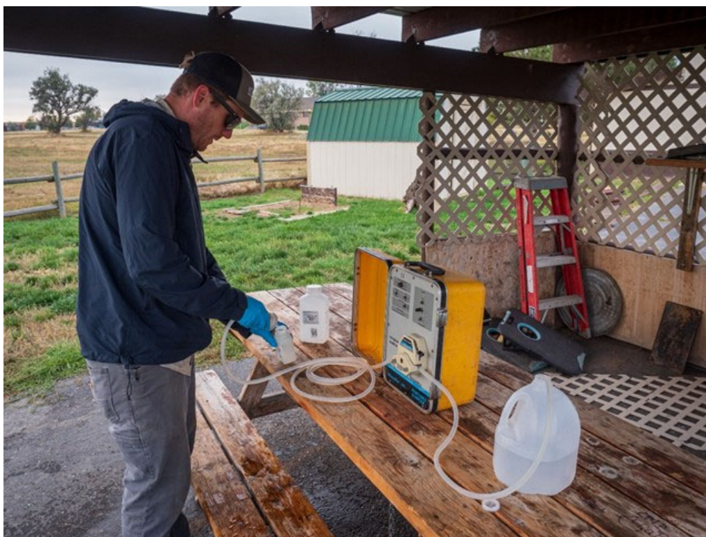
Figure 3.3. Preparing an equipment blank sample. The orange-colored peristaltic pump was used to pump deionized water from the 1-gallon container on the right through the sample filter and into the sample bottle.
