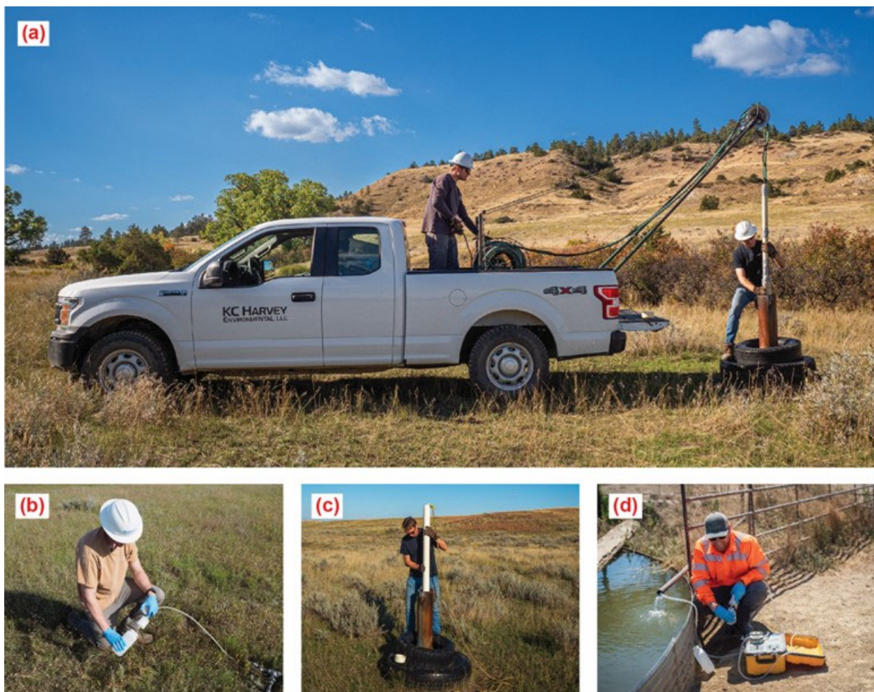
Figure 3.1. Well sampling: (a) Lowering the submersible pump into well GNW 6. (b) Filling sample bottles with flow from the submersible pump. Water from the well is pumped through the sampling manifold, a 3-ft section of ¼-in. OD poly tubing, and an in-line filter before flowing into the sample containers. (c) Lowering a bailer into well GNW 7. (d) Sampling the pump outfall at well GOW 12 using a peristaltic pump.
