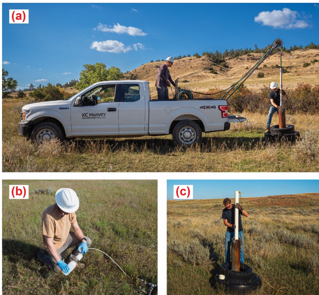
Figure 3.1. Well sampling: (a) Lowering the submersible pump into well GNW 6. (b) Filling sample bottles. Water from the well is pumped through the sampling manifold, a 3-ft section of \frac{1}{4} -in. OD poly tubing, and an in-line filter before flowing into the sample containers. (c) Lowering a bailer into well GNW 7.
