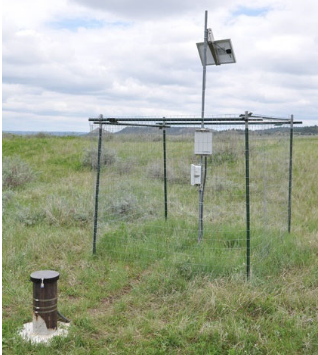
Figure 3.16. Well PW 736 with companion datalogger enclosure, solar panel, and fenced enclosure.
