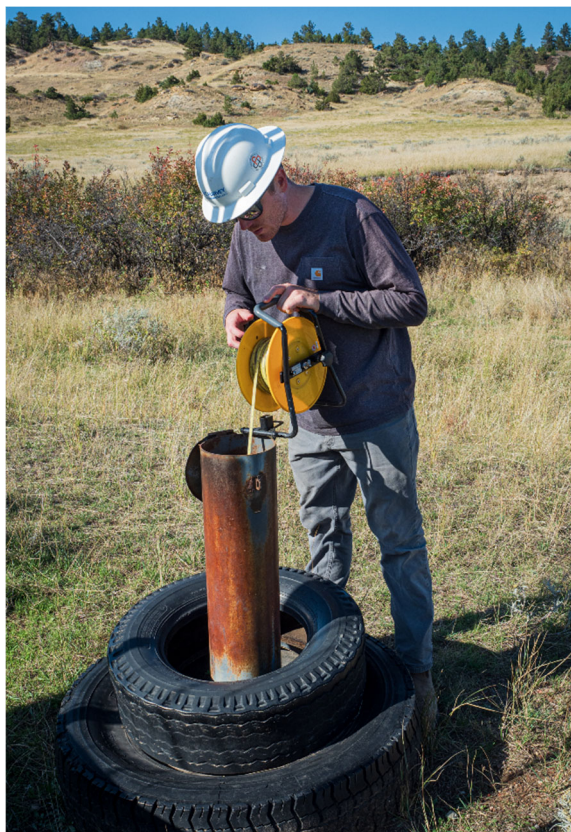
Figure 2.3. Measuring DTW with a water-level meter.
