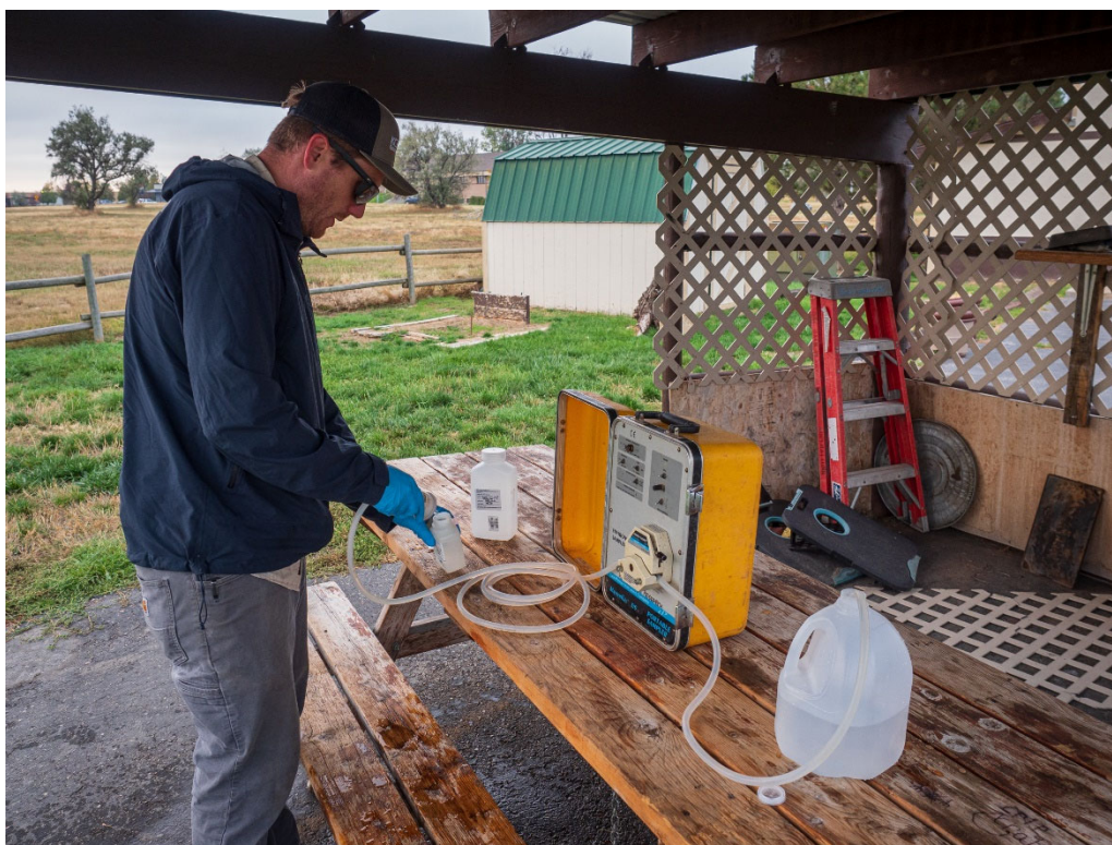
Figure 3.3. Preparing an equipment blank sample. Deionized water was pumped from the 1-gallon container on the right through a sample filter and into the sample bottle.
