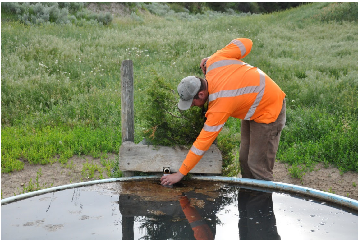
Figure 3.2. Measuring the flow rate at a spring.
