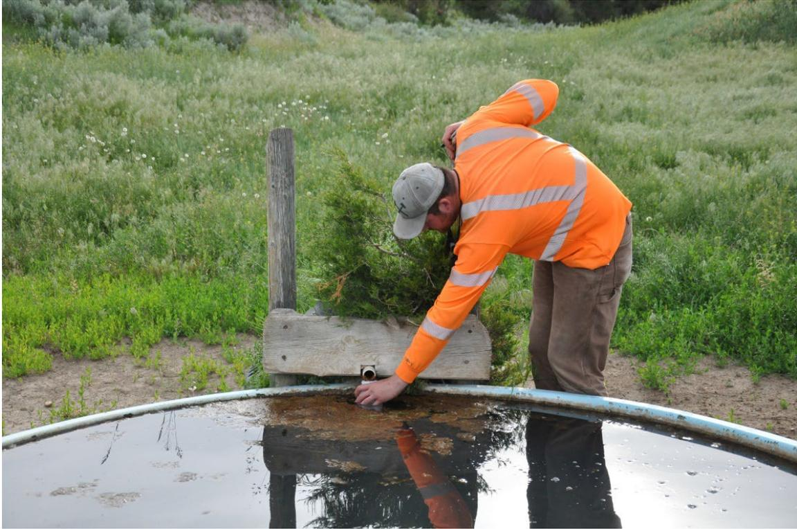
Figure 3.2. Measuring the flow rate at a spring.
