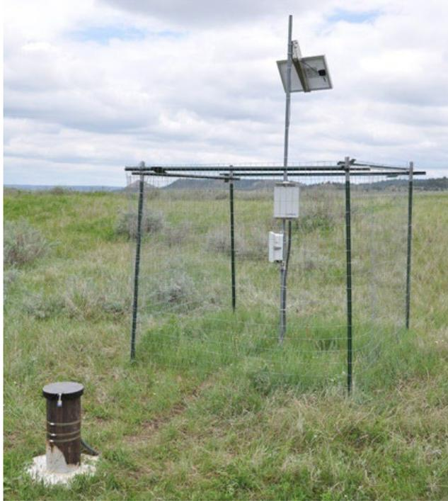
Figure 3.19. Well PW 736 with companion datalogger enclosure, solar panel, and fenced enclosure.
