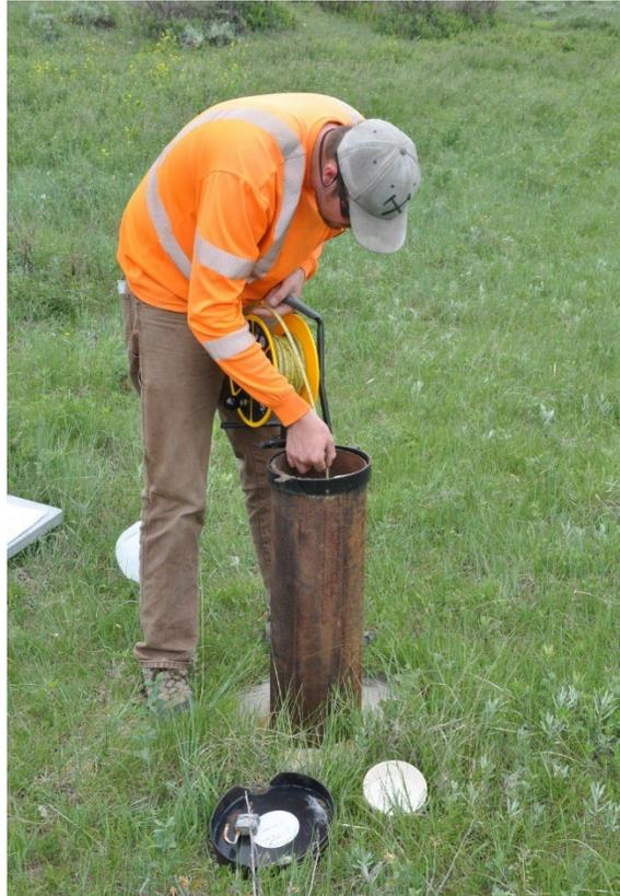
Figure 2.3. Measuring DTW with a water-level meter.
