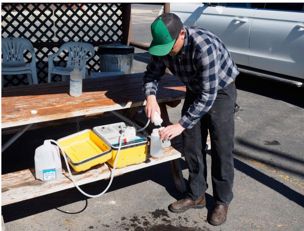
Figure 3.3. Preparing an equipment blank sample. Deionized water was pumped from the container on the left through a sample filter and into the sample bottle.
