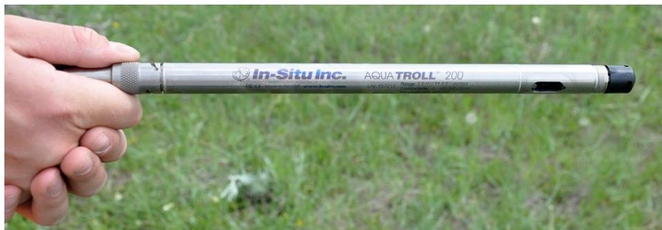
Figure 3.18. Continuous-monitoring probe.
