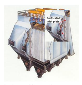
plate that distributes the gas flow through the precipitator, which makes more efficient use of the available space.
