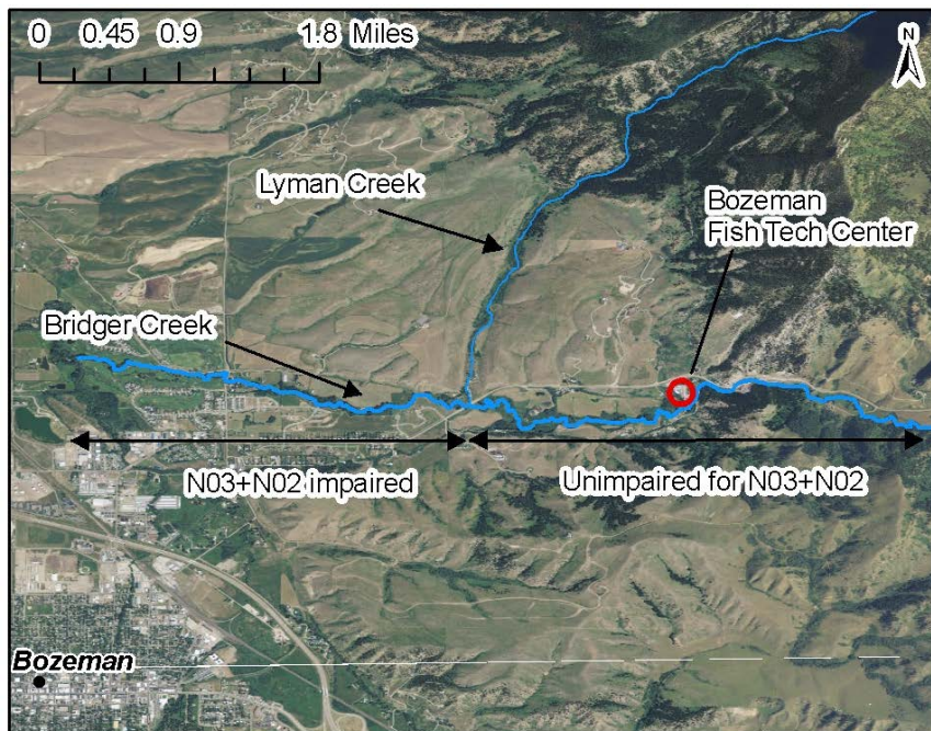
Figure 6-34. Delineation of segments above and below the Lyman Creek confluence in the Bridger Creek watershed
