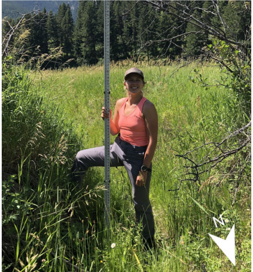
A GWC staff member stands in an incised channel cross-section. Incision is preventing the stream from flowing out onto its floodplain. (Photo: GWC)
