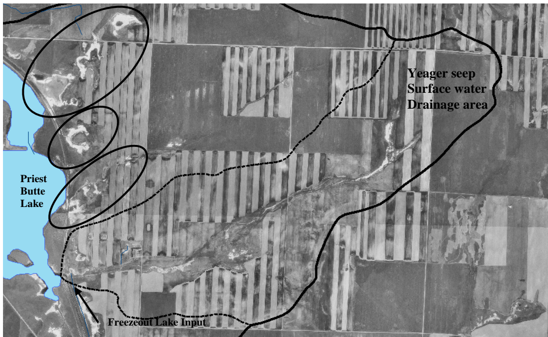
Figure 4-4. Yeager seep surface water drainage area (dashed line) and other Priest Butte Lakes east-side saline seep areas (solid ovals). The light blue lines are man-made ditches or canals. (Photo source is USGS; north is to the top of the photo; scale is approximately 1:25,000.)
