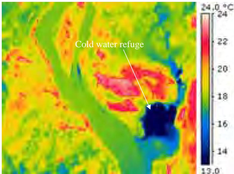
Figure 8. FLIR image of cold water refuge found at river mile 39.5
