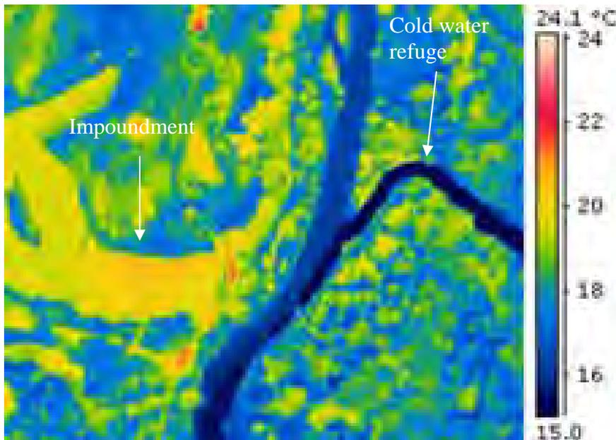
Figure 10. FLIR image of impoundment and cold water refuge found at river mile 26.8.
