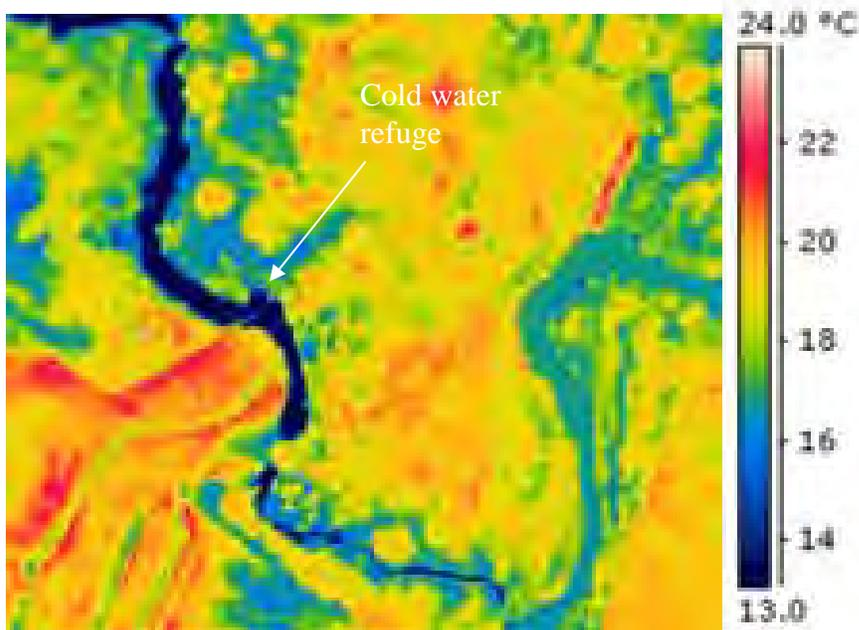
Figure 9. FLIR image of cold water refuge (entering from top left) found at river mile 37.2.
