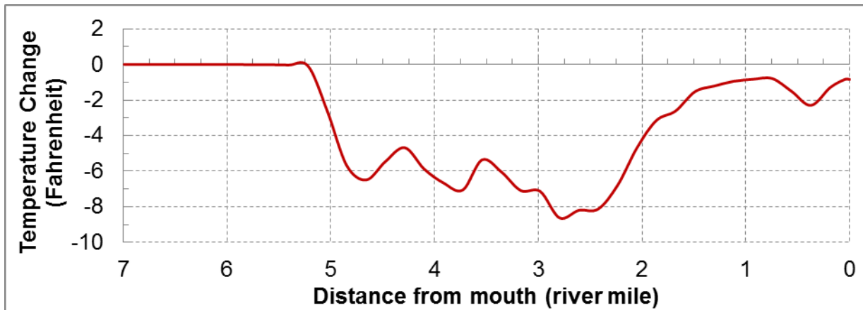
Figure D-20. Simulated water temperature reduction from the baseline condition (scenario 1) to the improved flow and shade scenario (scenario 4)
