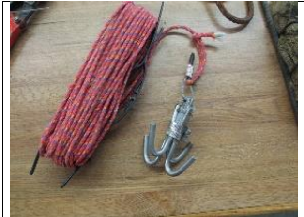
Figure 29. Grappling hook assembled using commonly available hardware
