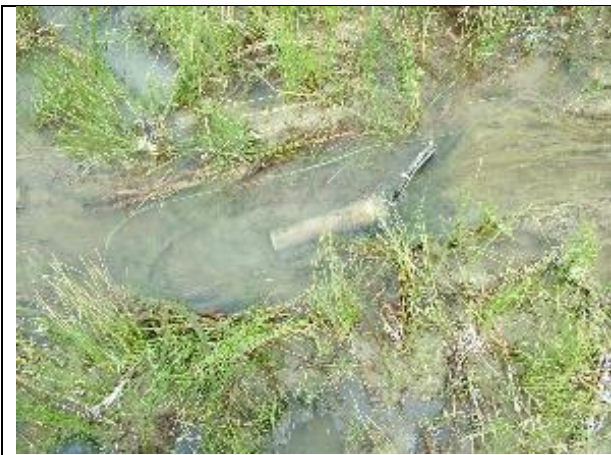
Figure 21. Deployment site on a very small stream using rebar loop at thalweg location
