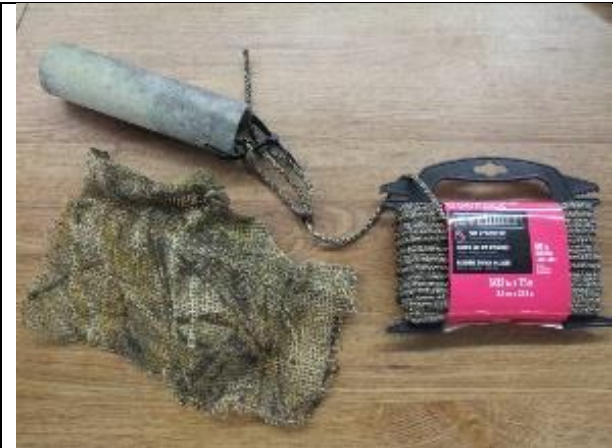
Figure 28. Camo cord temperature logger assembly showing doubled zip ties, camo cord tied through the logger and the zip ties inside the shade tube with a bowline knot, and burlap cloth to be attached around the shade tube.
