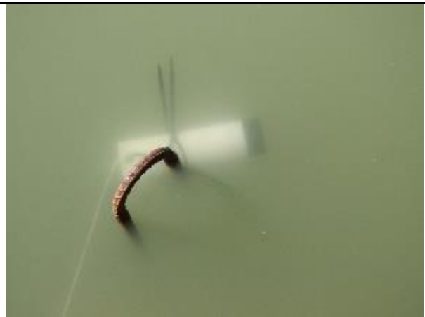
Figure 35. MiniDOT deployment in the water column using U-shaped rebar and cable tether. Note horizontal logger orientation
