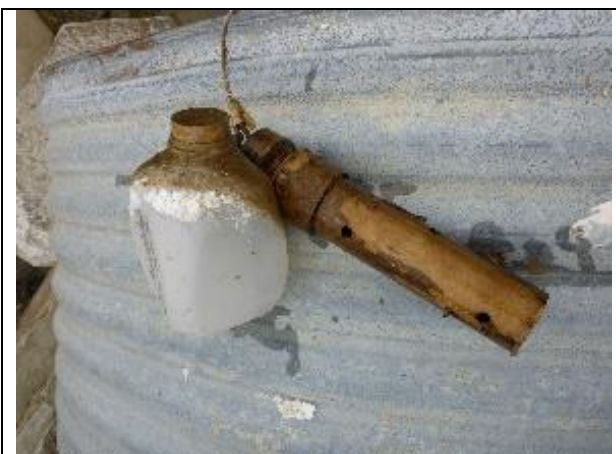
Figure 17. A float system setup to assure that the logger is not buried.
