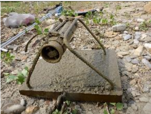
Figure 27. Cast concrete and rebar anchor and shade tube system with stainless steel cable for deployment at a bridge at a large river site.
