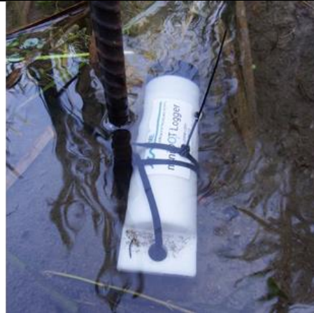
Figure 34. MiniDOT zip tied to rebar (Note 3 zip tie configuration).
