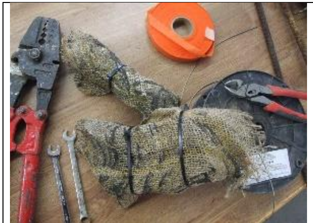
Figure 31. Camo burlap installed on shade tube and brick, tools and flagging
