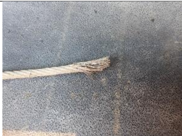
Figure 39. Vandals will go to great lengths to remove a data logger from a stream by cutting the cable.
