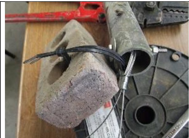
Figure 30. Shade tube zip tied to brick (note 2 zip ties).
