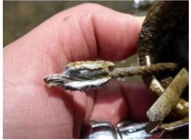
Figure 37 and 38. High EC stream resulted in corroded aluminum ferrule, which was replaced using a salinity-resistant alloy ferrule.
