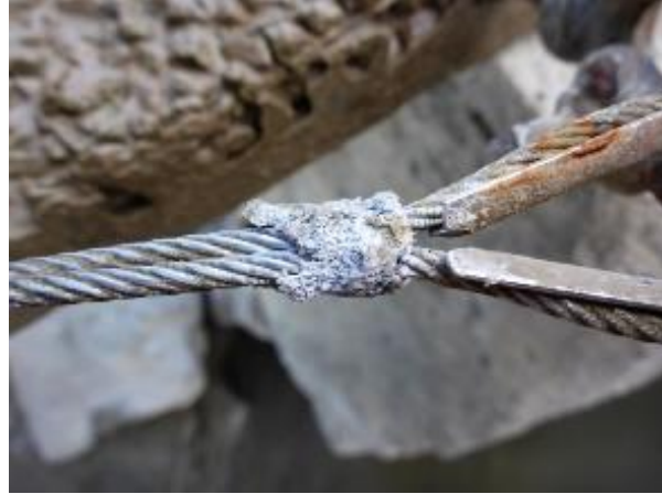
Figure 37 and 38. High EC stream resulted in corroded aluminum ferrule, which was replaced using a salinity-resistant alloy ferrule.
