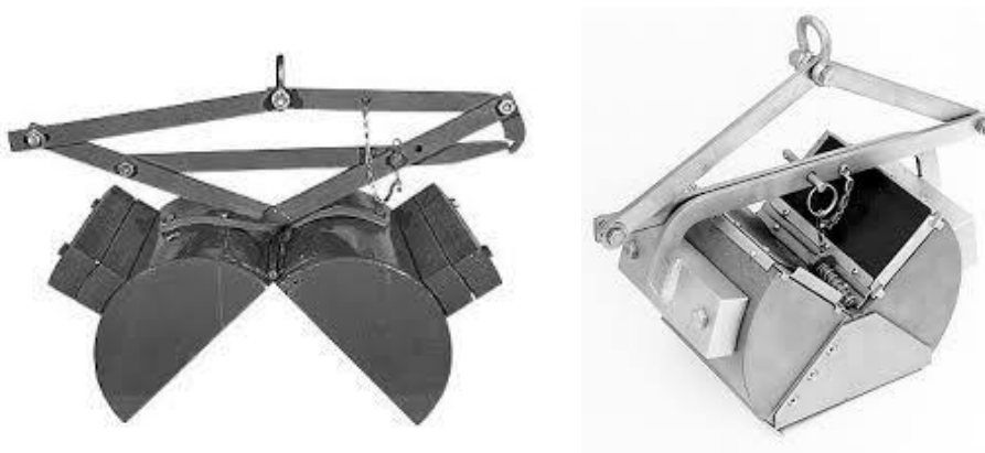
Figure 11: Ekman (left) and Ponar (right) Samplers
