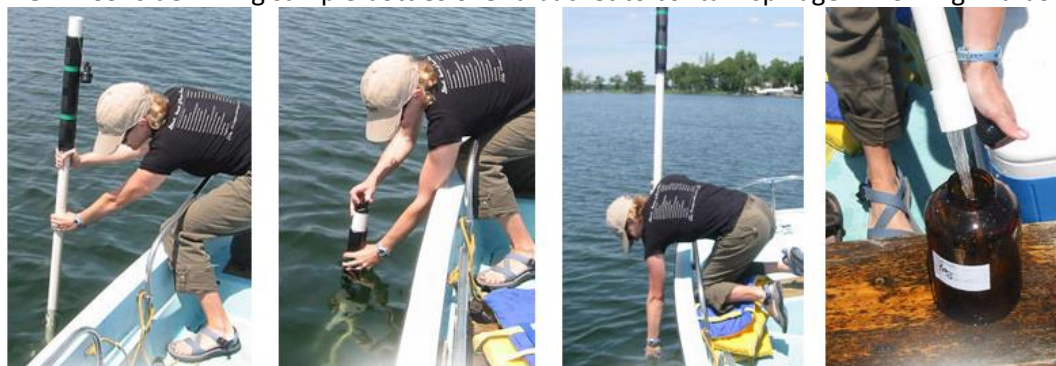
Figure 8: Using a 2-meter Integrated Sampler
