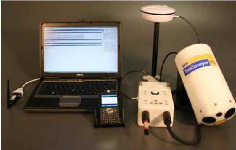
Figure 2-1. ADP setup for DGPS configuration including computer and Bluetooth Pirani dongle.
