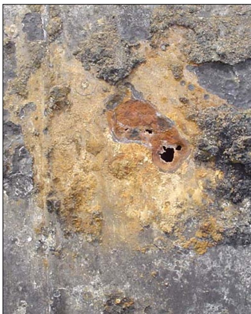
Hole in a metal tank from corrosion
